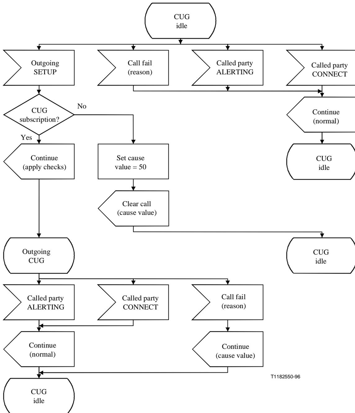
**Figure 2/Q.2955.1 – Closed user group process – Outgoing call (network side)**
