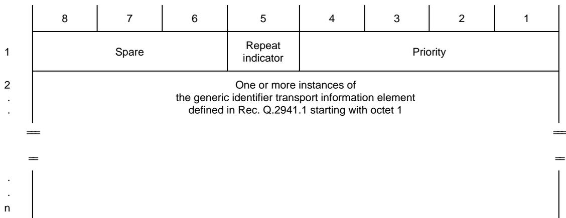
**Figure 1/Q.2726.4 – Application generated identifier parameter**
