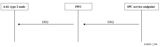
Figure 4/Q.2632.1 – ERQ from IP network
