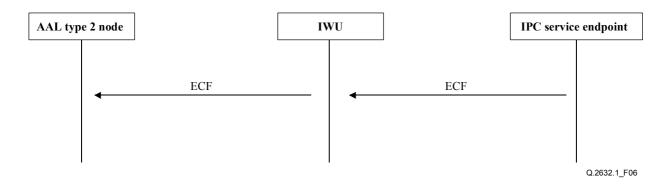
Figure 6/Q.2632.1 – ECF from IP network
