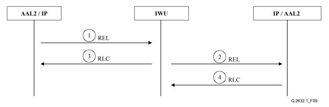
Figure 9/Q.2632.1 – General release handling
