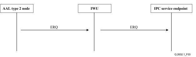
Figure 3/Q.2632.1 – ERQ from AAL type 2 network
