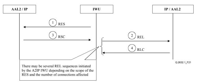
Figure 21/Q.2632.1 – General IWU-initiated reset handling
