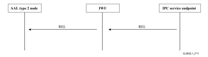
Figure 11/Q.2632.1 – REL from IP network
