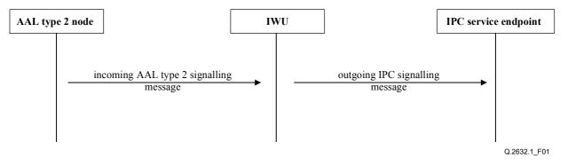
Figure 1/Q.2632.1 – AAL type 2 to IPC signalling interworking
