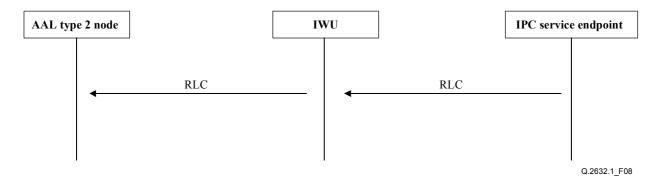
Figure 8/Q.2632.1 – RLC from IP network
