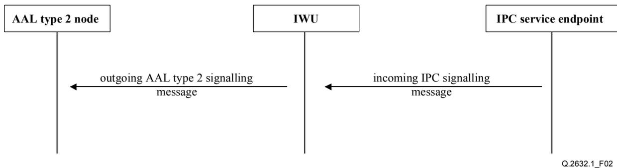
**Figure 2/Q.2632.1 – IPC to AAL type 2 signalling interworking**
