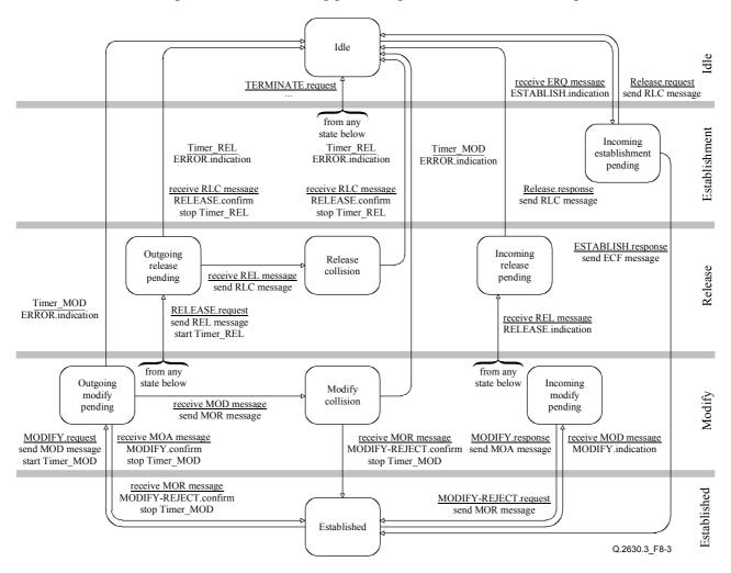
Figure 8-3/Q.2630.3 – State transition diagram for the incoming protocol procedure
