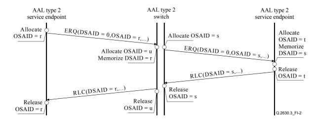
Figure I.2/Q.2630.3 – Example of a message sequence for an unsuccessful AAL type 2 connection establishment
