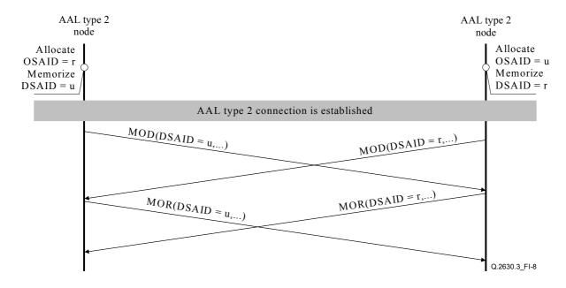
Figure I.8/Q.2630.3 – Example of a message sequence for a resource modification collision of an established AAL type 2 connection
