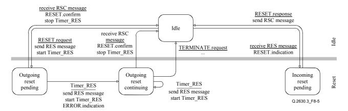
Figure 8-5/Q.2630.3 – State transition diagram for the maintenance control procedure (reset)
