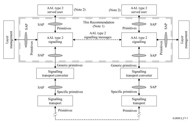
NOTE 1 – The entities and Service Access Points (SAP) bounded by the gray broken line indicate the extent of the definitions specified in this Recommendation.
