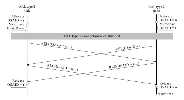
Figure I.4/Q.2630.3 – Example of a message sequence for a release collision on an AAL type 2 connection
