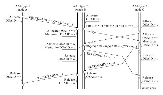
Figure I.5/Q.2630.3 – Example of a message sequence for a resource contention on two AAL type 2 connections
