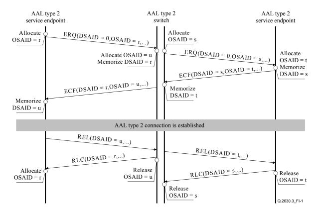
Figure I.1/Q.2630.3 – Example of successful AAL type 2 connection establishment and release message sequences
