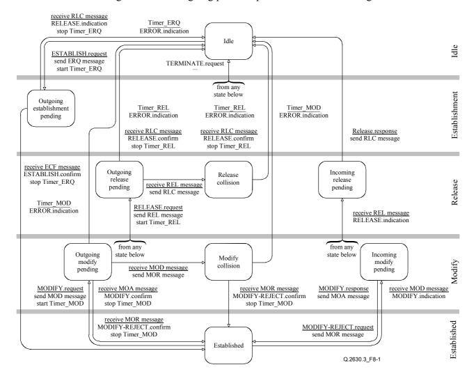
Figure 8-1/Q.2630.3 – State transition diagram for the outgoing protocol procedure
