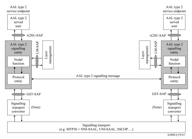
NOTE – A signalling transport converter instance is associated with each AAL type 2 signalling transport.
