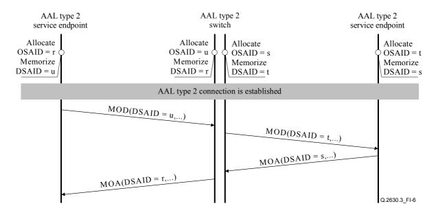
Figure I.6/Q.2630.3 – Example of a message sequence for a successful resource modification of an established AAL type 2 connection
