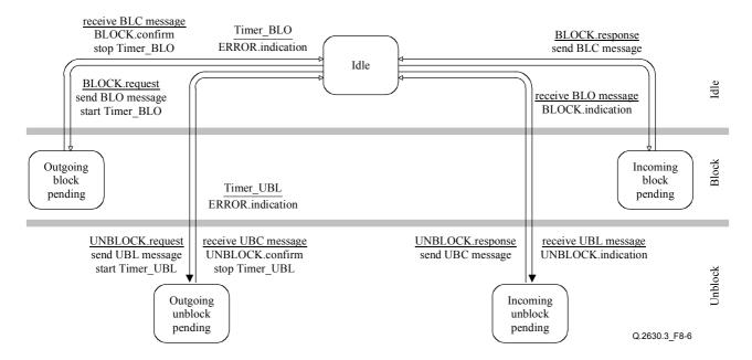
Figure 8-6/Q.2630.3 – State transitions of the maintenance control procedure (blocking and unblocking)
