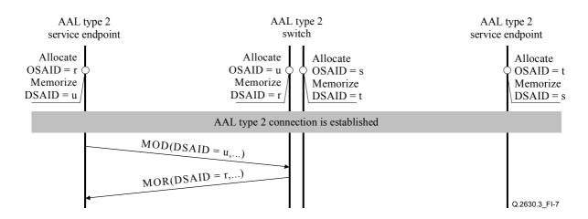
Figure I.7/Q.2630.3 – Example of a message sequence for an unsuccessful resource modification of an established AAL type 2 connection
