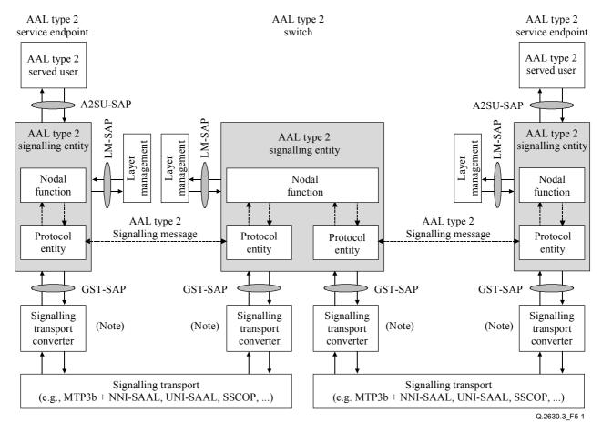
NOTE – In every AAL type 2 node, a signalling transport converter instance is associated with each AAL type 2 signalling transport.
