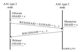
Figure I.3/Q.2630.3 – Example of a message sequence for a management operation
