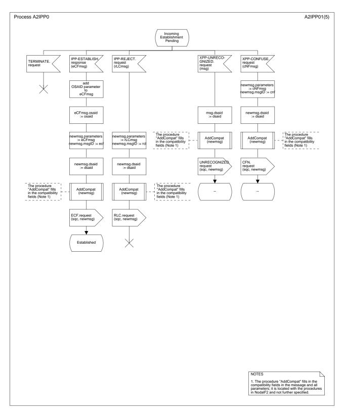
Figure B.5/Q.2630.1 – SDL diagram of the incoming protocol procedure (part 2 of 5)
