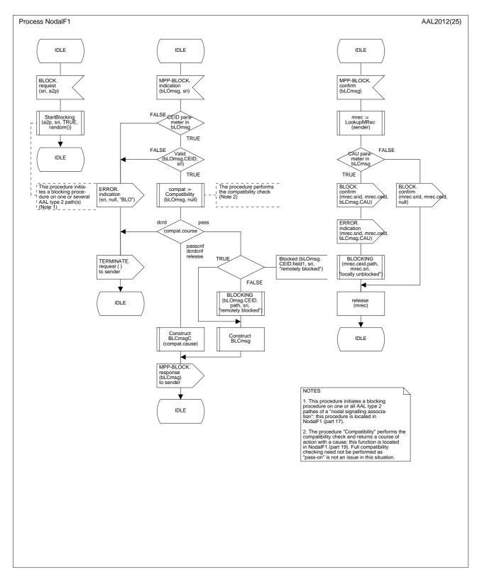
Figure B.3/Q.2630.1 – SDL diagram of the Nodal Function 1 (part 13 of 25)
