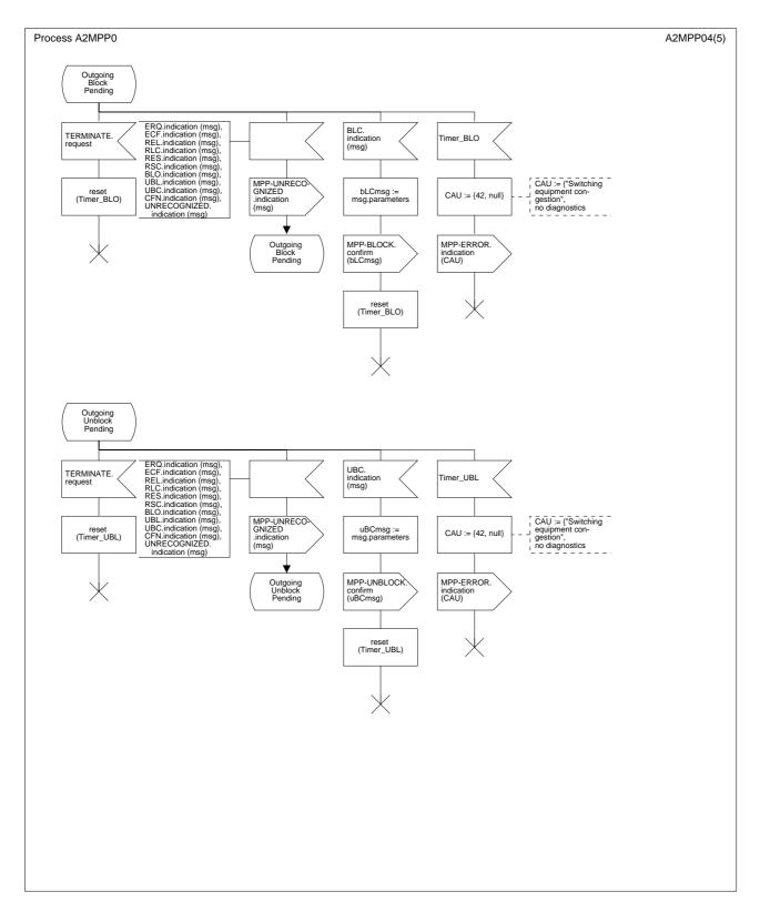
Figure B.6/Q.2630.1 – SDL diagram of the maintenance protocol procedure (part 5 of 5)
