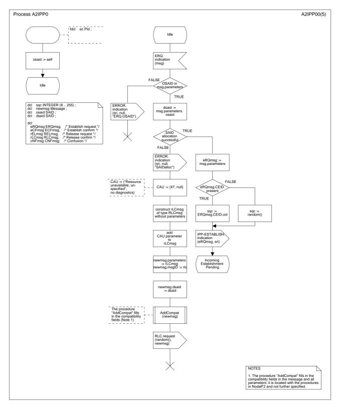
Figure B.5/Q.2630.1 – SDL diagram of the incoming protocol procedure (part 1 of 5)
