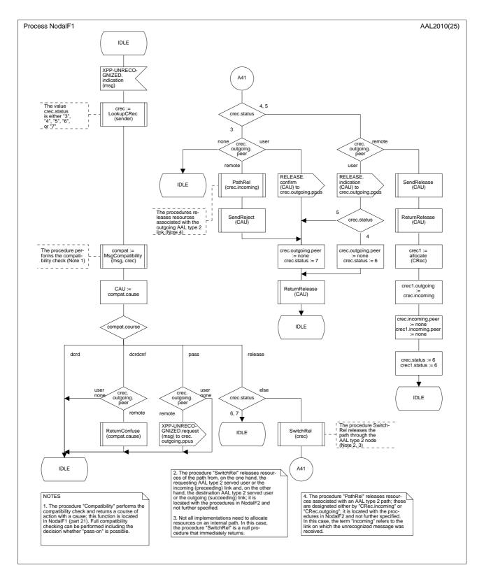
Figure B.3/Q.2630.1 – SDL diagram of the Nodal Function 1 (part 11 of 25)
