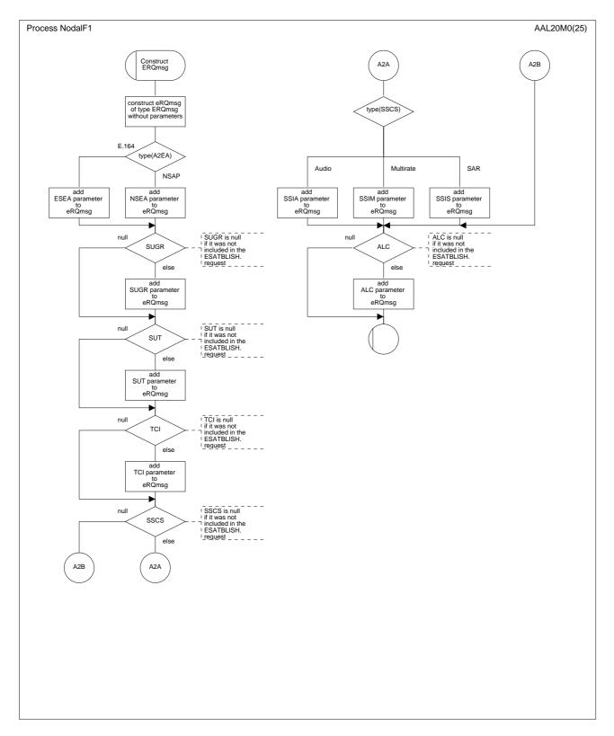
Figure B.3/Q.2630.1 – SDL diagram of the Nodal Function 1 (macros) (part 22 of 25)
