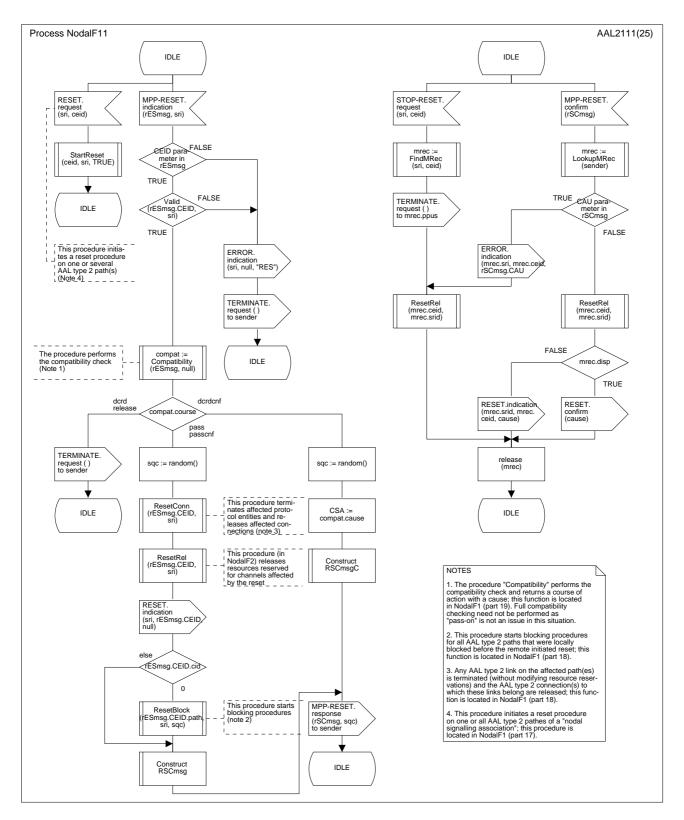
Figure B.3/Q.2630.1 – SDL diagram of the Nodal Function 1 (part 12 of 25)
