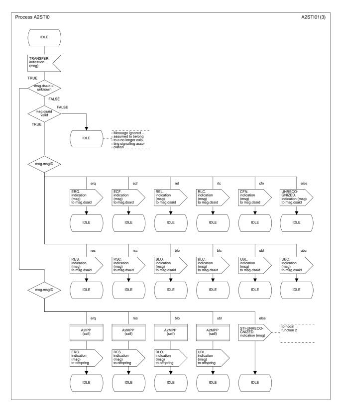
Figure B.7/Q.2630.1 – SDL diagram of the signalling transport interface (part 2 of 2)
