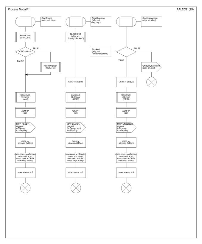
Figure B.3/Q.2630.1 – SDL diagram of the Nodal Function 1 (procedures) (part 17 of 25)
