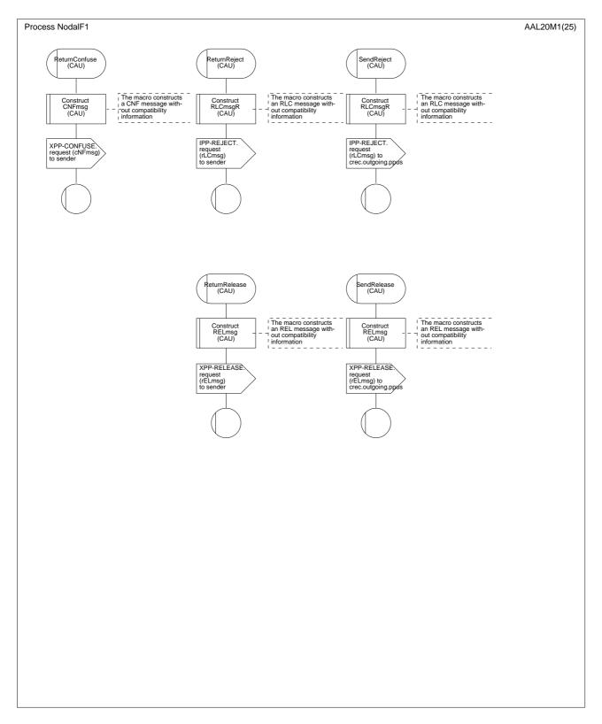
Figure B.3/Q.2630.1 – SDL diagram of the Nodal Function 1 (macros) (part 23 of 25)
