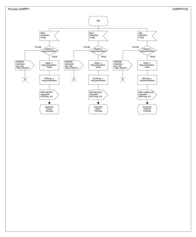
Figure B.6/Q.2630.1 – SDL diagram of the maintenance protocol procedure (part 2 of 5)
