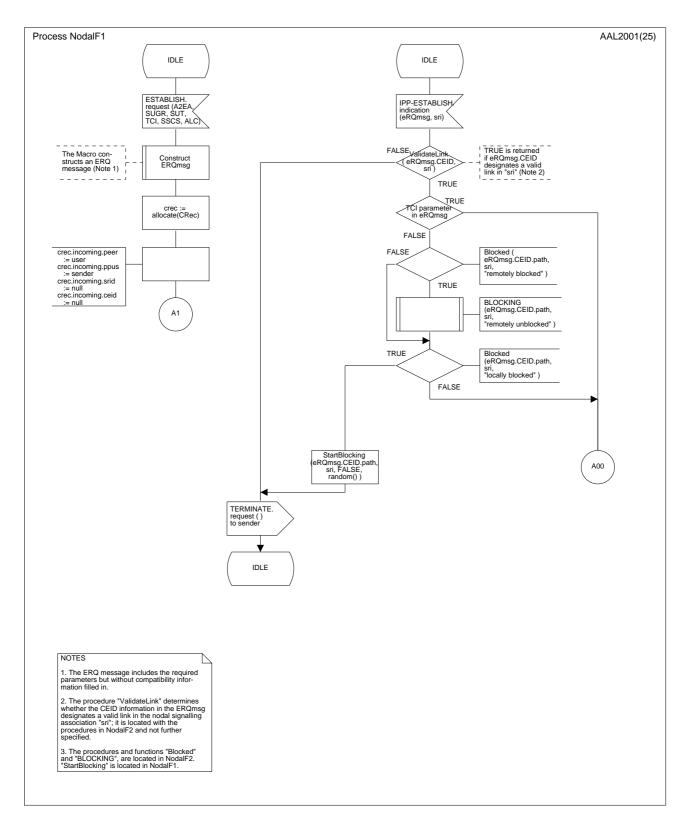
Figure B.3/Q.2630.1 – SDL diagram of the Nodal Function 1 (part 2 of 25)
