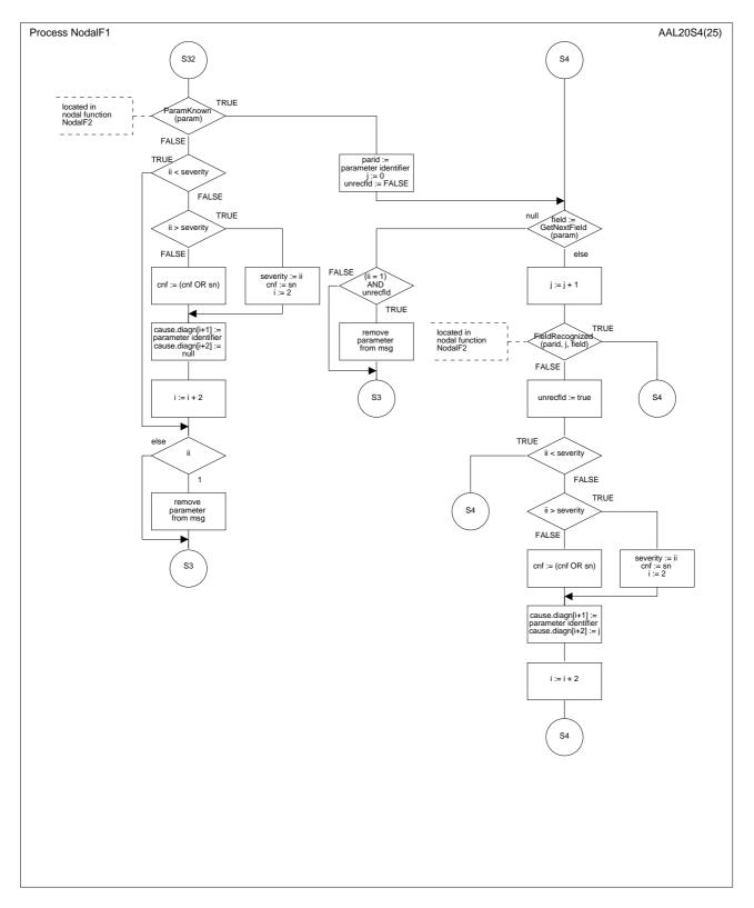
Figure B.3/Q.2630.1 – SDL diagram of the Nodal Function 1 (procedures) (part 20 of 25)
