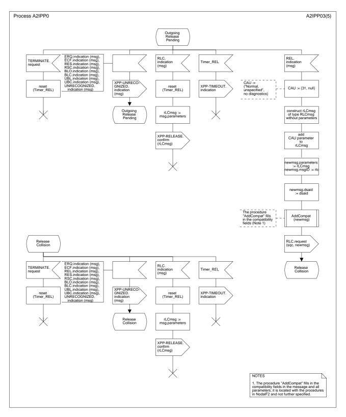
Figure B.5/Q.2630.1 – SDL diagram of the incoming protocol procedure (part 4 of 5)
