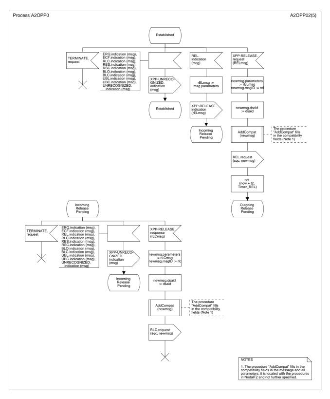
Figure B.4/Q.2630.1 – SDL diagram of the outgoing protocol procedure (part 3 of 5)
