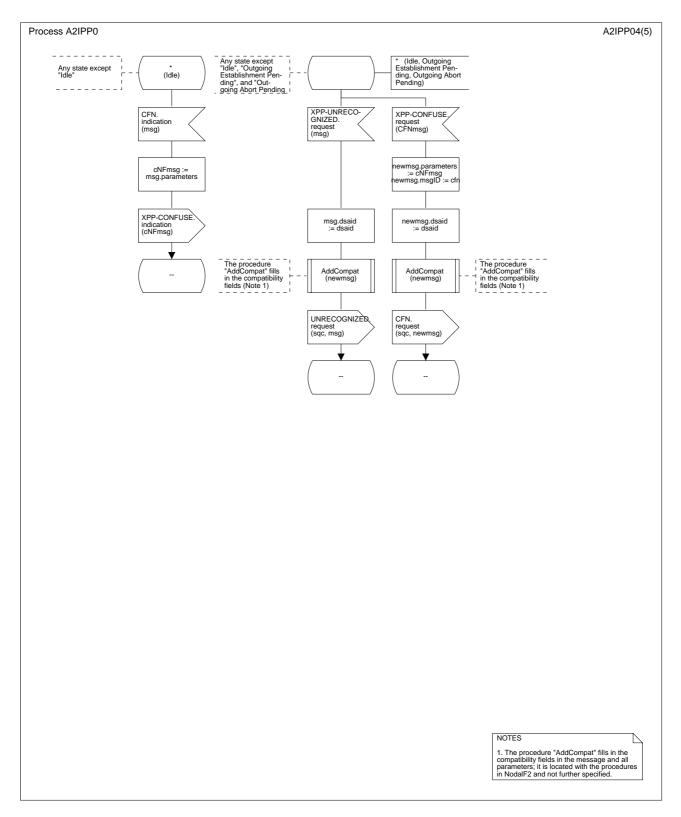
Figure B.5/Q.2630.1 – SDL diagram of the incoming protocol procedure (part 5 of 5)
