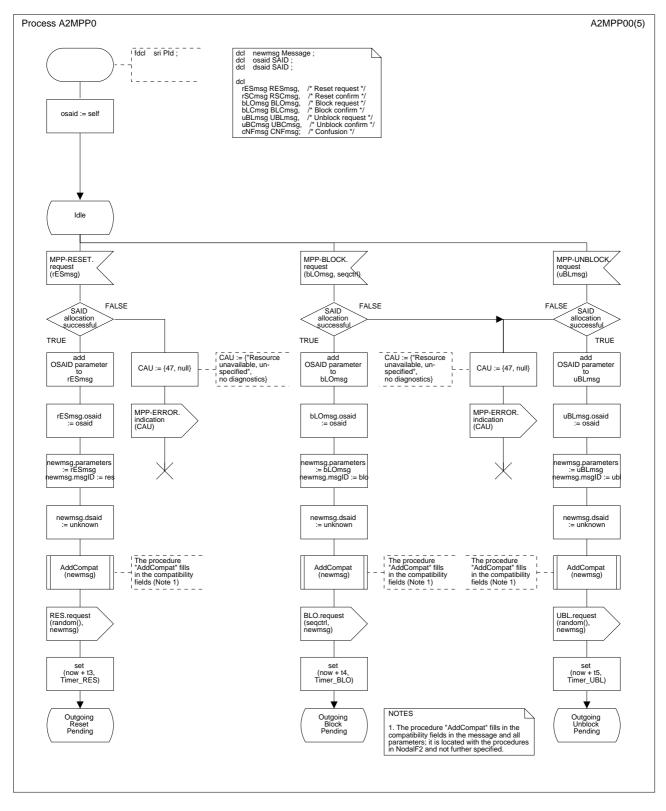
Figure B.6/Q.2630.1 – SDL diagram of the maintenance protocol procedure (part 1 of 5)
