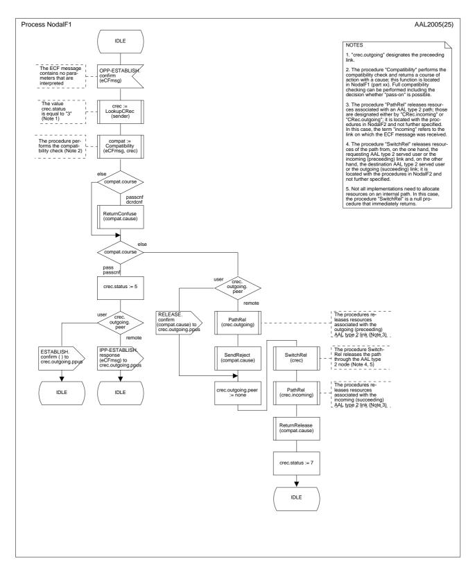
Figure B.3/Q.2630.1 – SDL diagram of the Nodal Function 1 (part 6 of 25)
