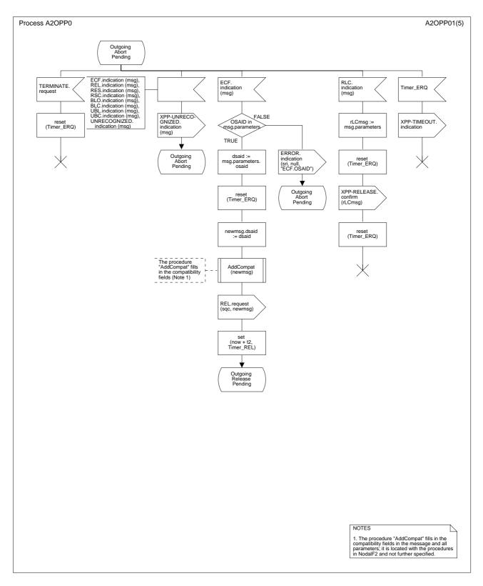
Figure B.4/Q.2630.1 – SDL diagram of the outgoing protocol procedure (part 2 of 5)
