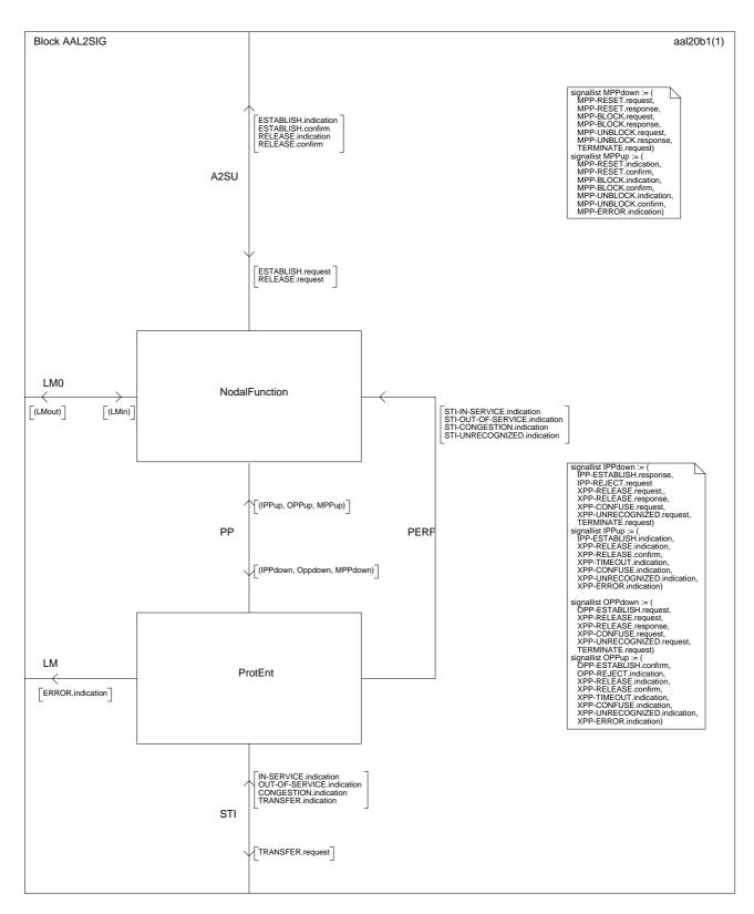
Figure B.2/Q.2630.1 – SDL block structure of the AAL type 2 signalling entity (*part 2 of 4*)
