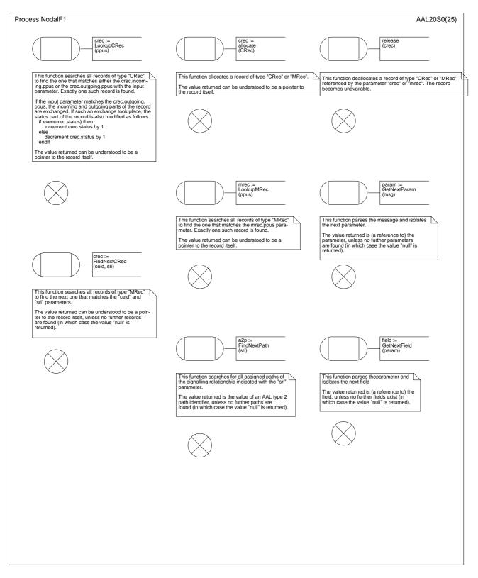
Figure B.3/Q.2630.1 – SDL diagram of the Nodal Function 1 (procedures) (part 16 of 25)
