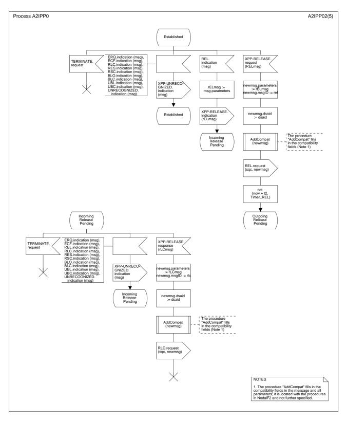
Figure B.5/Q.2630.1 – SDL diagram of the incoming protocol procedure (part 3 of 5)
