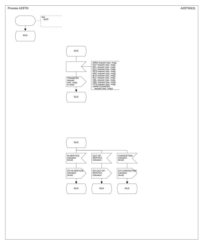
Figure B.7/Q.2630.1 – SDL diagram of the signalling transport interface (part 1 of 2)
