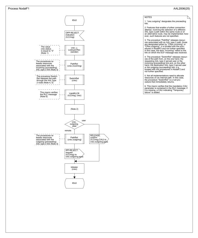
Figure B.3/Q.2630.1 – SDL diagram of the Nodal Function 1 (part 7 of 25)
