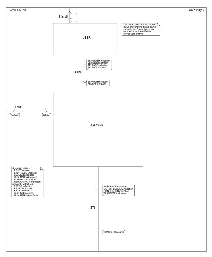
Figure B.2/Q.2630.1 – SDL block structure of the AAL type 2 signalling entity (*part 1 of 4*)
