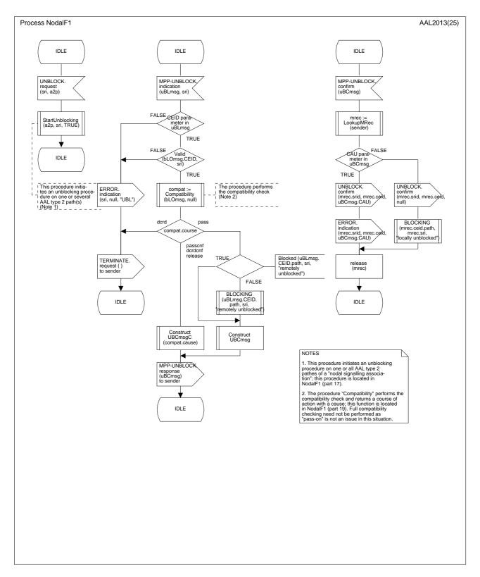
Figure B.3/Q.2630.1 – SDL diagram of the Nodal Function 1 (part 14 of 25)
