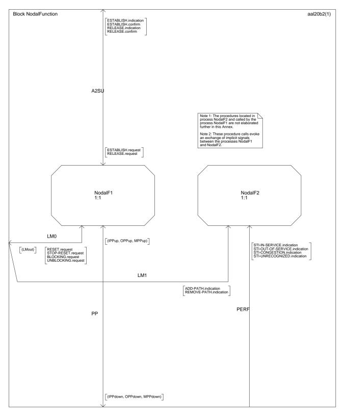
Figure B.2/Q.2630.1 – SDL block structure of the AAL type 2 signalling entity (*part 3 of 4*)
