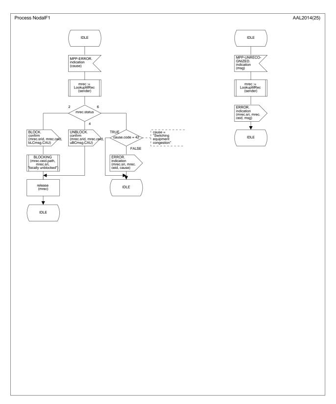
Figure B.3/Q.2630.1 – SDL diagram of the Nodal Function 1 (part 15 of 25)
