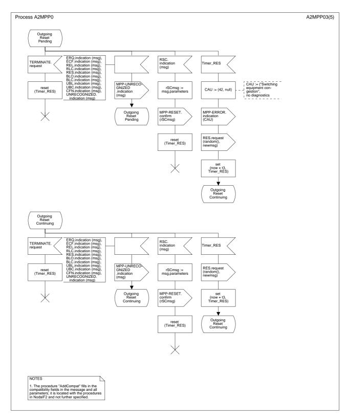
Figure B.6/Q.2630.1 – SDL diagram of the maintenance protocol procedure (part 4 of 5)
