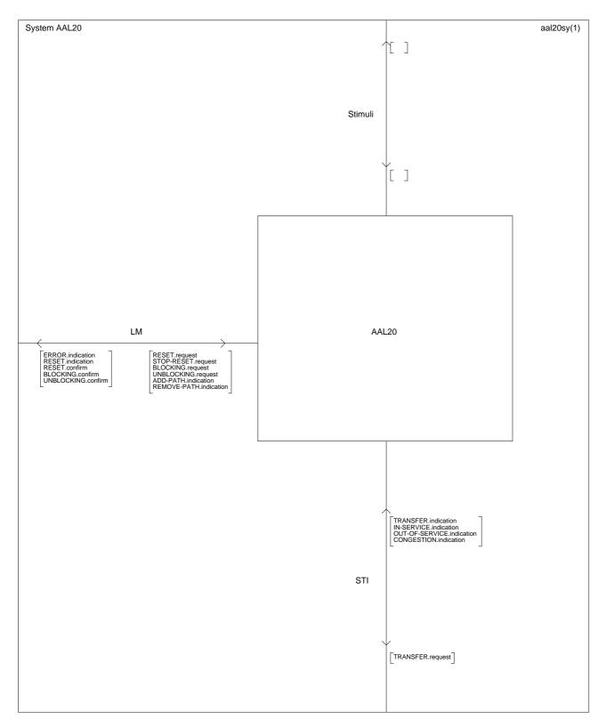
Figure B.1/Q.2630.1 – SDL system of the AAL type 2 signalling entity
