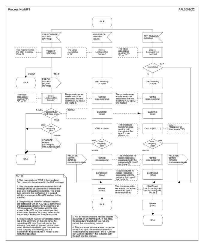
Figure B.3/Q.2630.1 – SDL diagram of the Nodal Function 1 (part 10 of 25)
