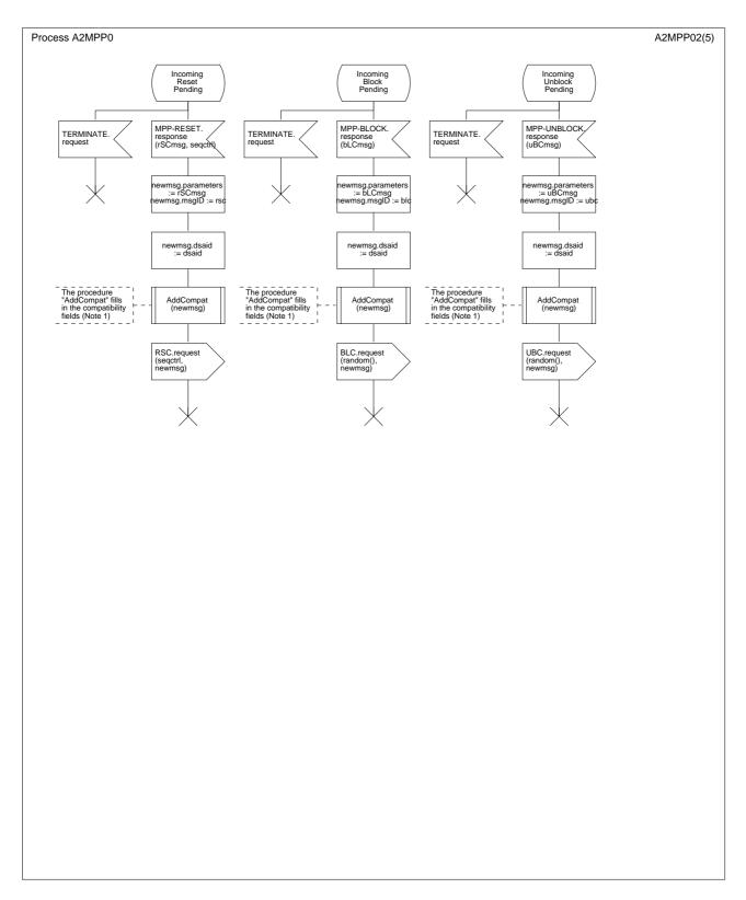
Figure B.6/Q.2630.1 – SDL diagram of the maintenance protocol procedure (part 3 of 5)
