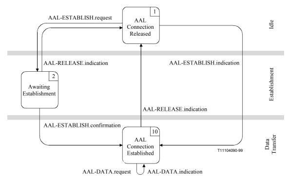
Figure I.2/Q.2150.2 – State transition diagram for sequences of primitives between the STC and SSCF-UNI
