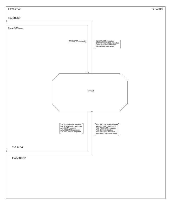
Figure 8-3/Q.2150.2 – SDL block structure of the AAL type 2 signalling transport converter
