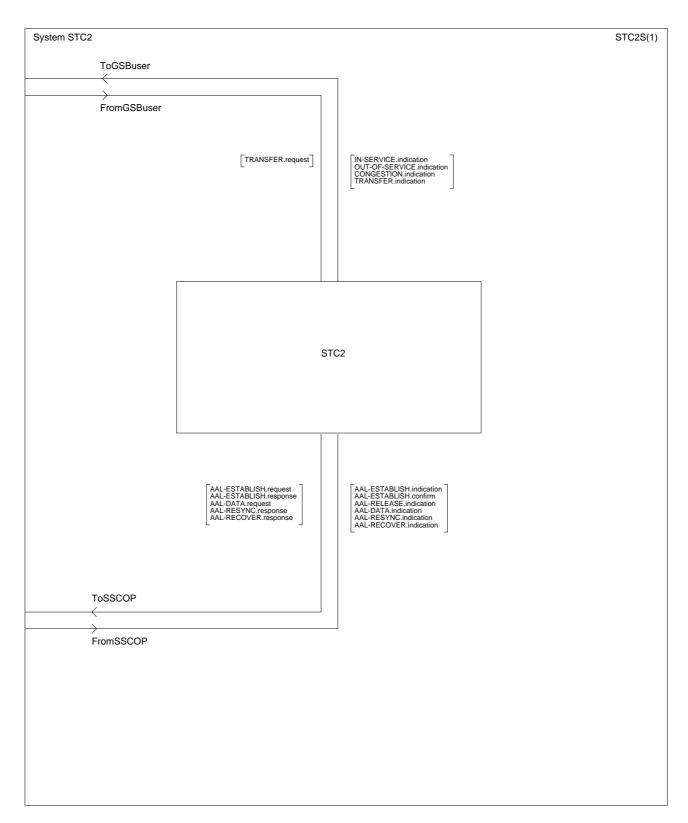
Figure 8-2/Q.2150.2 – SDL system of the AAL type 2 signalling transport converter
