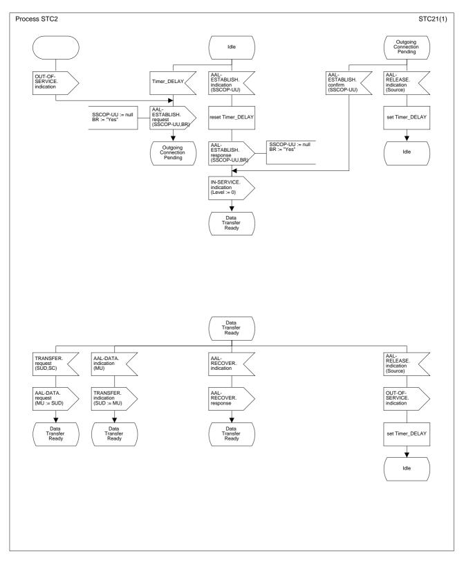
Figure 8-4/Q.2150.2 – SDL diagram for the AAL type 2 signalling transport converter
