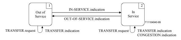
Figure 6-1/Q.2150.2 – State transition diagram for sequences of primitives between the STC and its user
