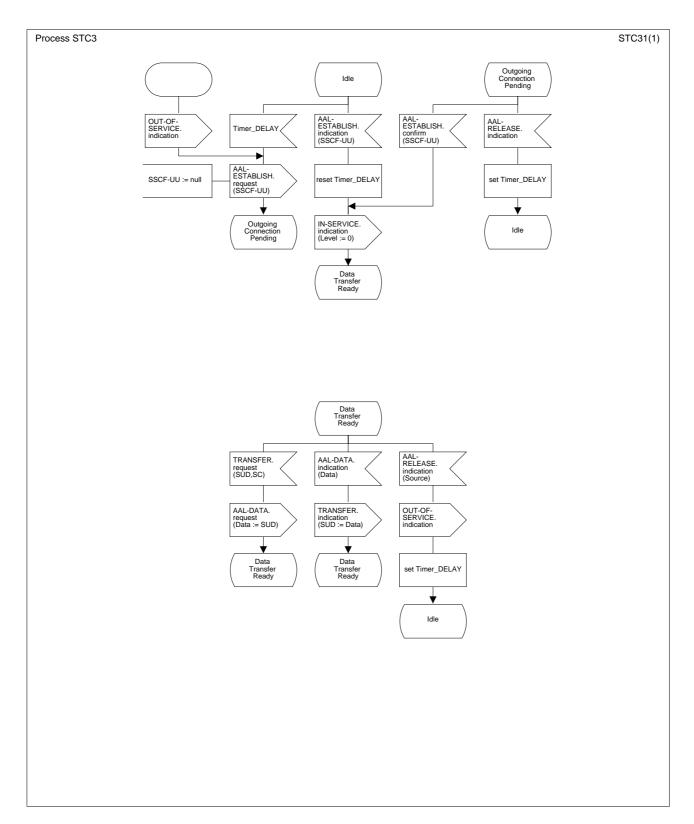
Figure I.3/Q.2150.2 – SDL diagram for the AAL type 2 signalling transport converter
