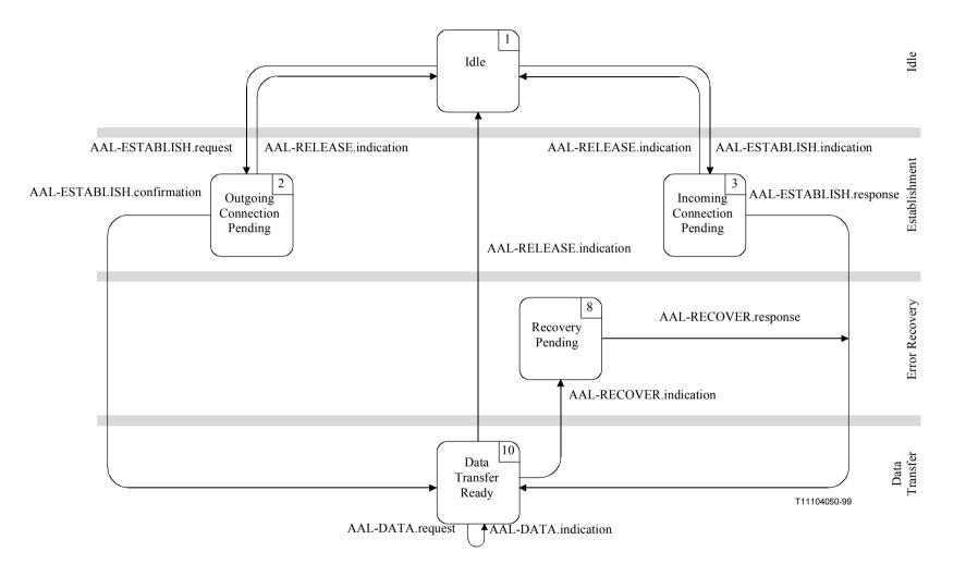
Figure 6-2/Q.2150.2 – State transition diagram for sequences of primitives between the STC and SSCOP
