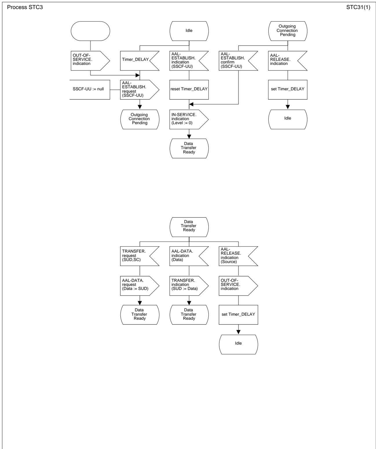
Figure I.3/Q.2150.2 – SDL diagram for the AAL type 2 signalling transport converter
