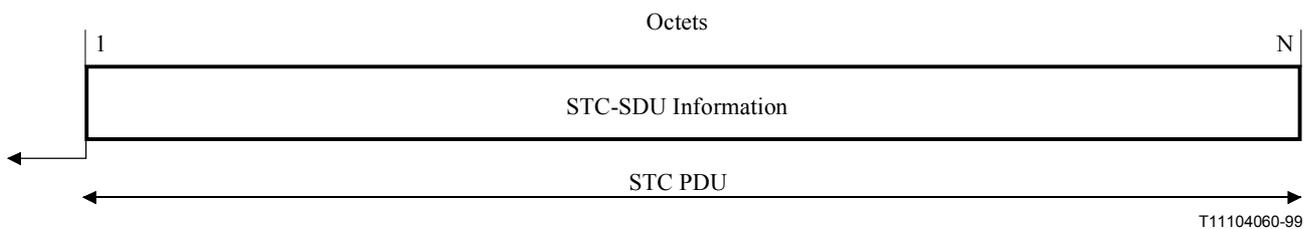
**Figure 7-1/Q.2150.2 – STC Data PDU**
