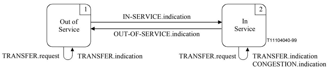
**Figure 6-1/Q.2150.2 – State transition diagram for sequences of primitives between the STC and its user**
