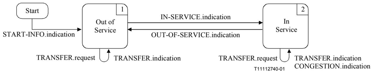
**Figure 6-1/Q.2150.0 – State transition diagram for sequences of primitives**
