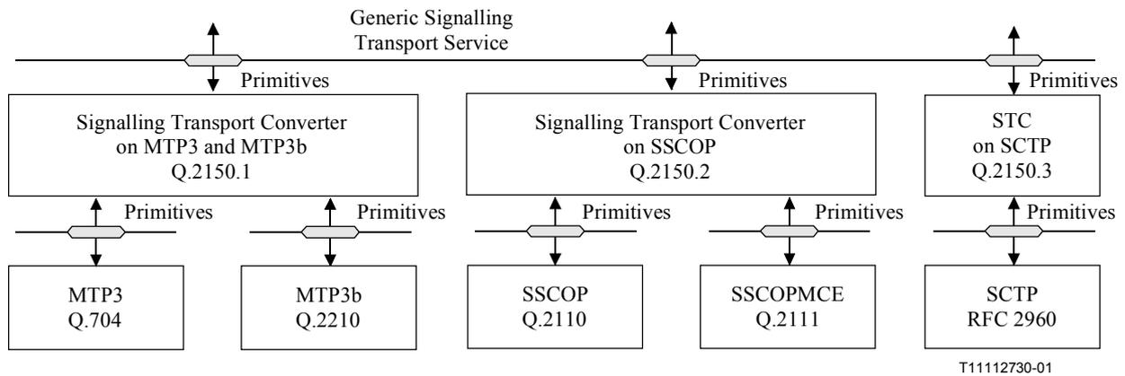
**Figure 5-2/Q.2150.0 – Example protocol stacks for the Generic Signalling Transport Service**
