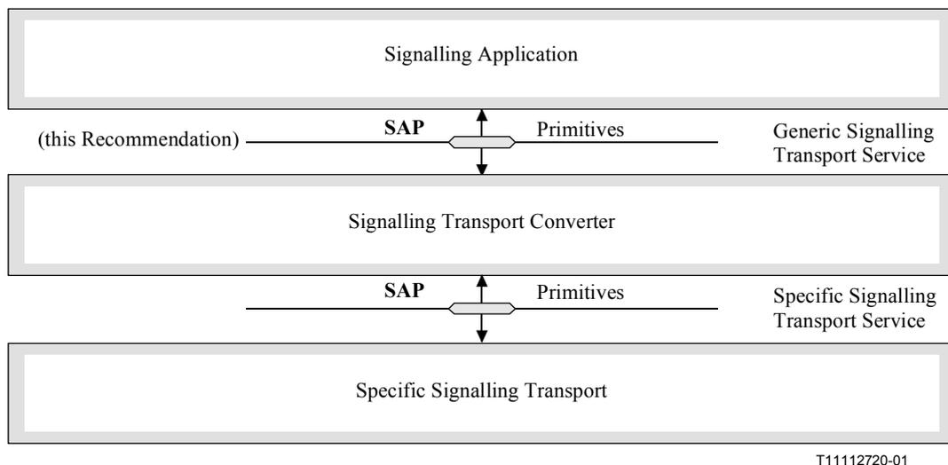
**Figure 5-1/Q.2150.0 – Framework for the Generic Signalling Transport Service**
