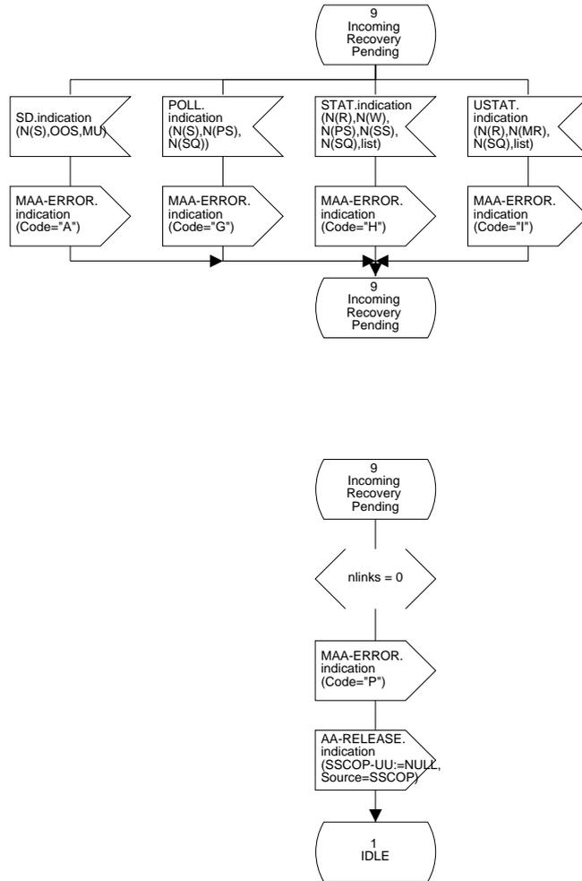
Figure 22/Q.2111 – SDL diagram of the multilink SSCOPMCE protocol entity (sheet 21 of 38)
