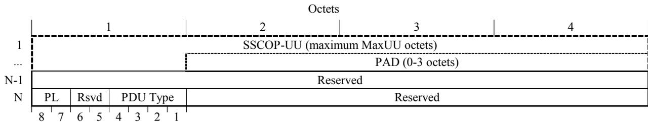
**Figure 7/Q.2111 – Begin reject PDU (BGREJ PDU)**
