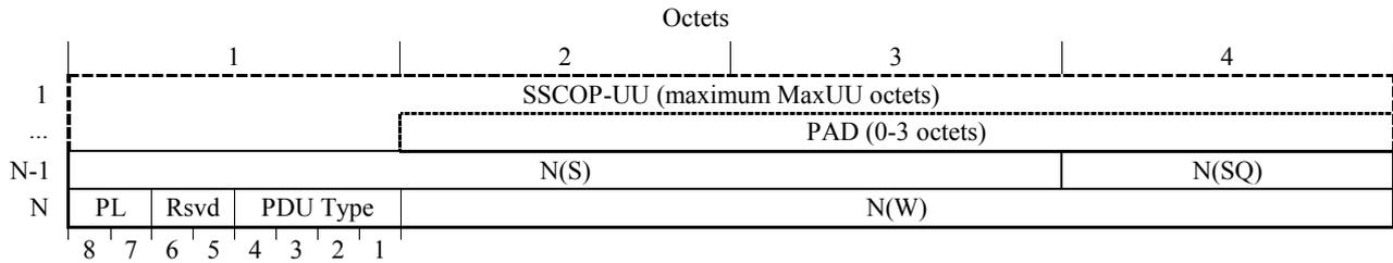
**Figure 5/Q.2111 – Begin PDU (BGN PDU)**
