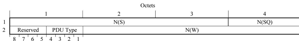
**Figure 13/Q.2111 – Error recovery acknowledge PDU (ERAK PDU)**
