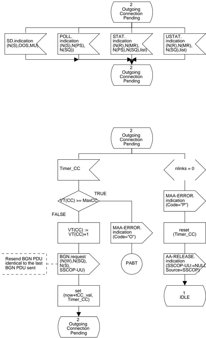
Figure 22/Q.2111 – SDL diagram of the multilink SSCOPMCE protocol entity (sheet 6 of 38)
