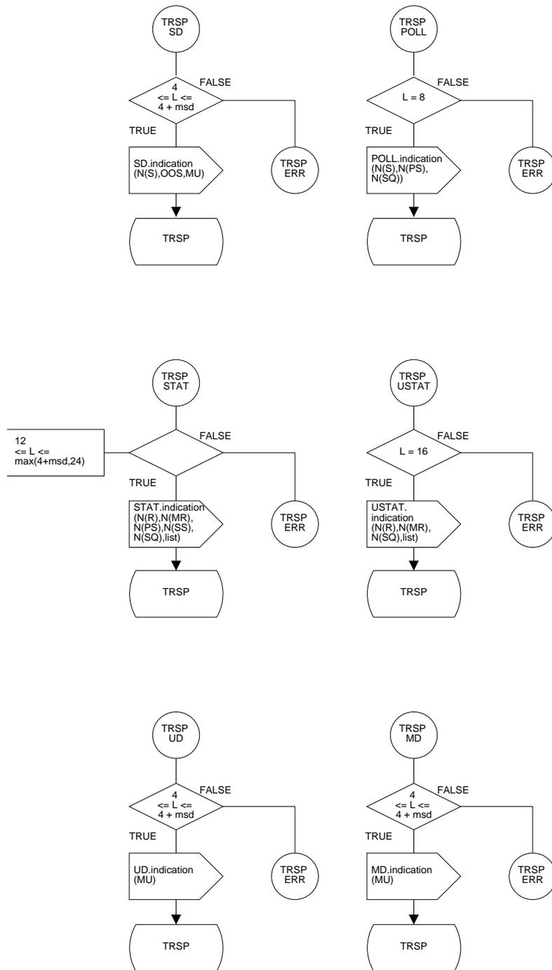
Figure B.1/Q.2111 – SDL diagram of the ancillary process TRSP (sheet 4 of 4)
