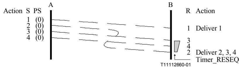
**Figure II.15/Q.2111 – Recovery of out-of-sequence receipt of SD PDUs with Timer\_RESEQ**
