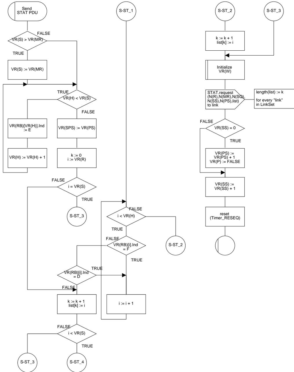
Figure 22/Q.2111 – SDL diagram of the multilink SSCOPMCE protocol entity (sheet 34 of 38)
