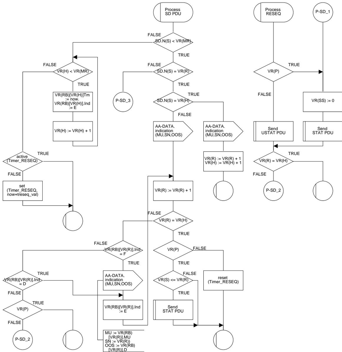
Figure 22/Q.2111 – SDL diagram of the multilink SSCOPMCE protocol entity (sheet 31 of 38)
