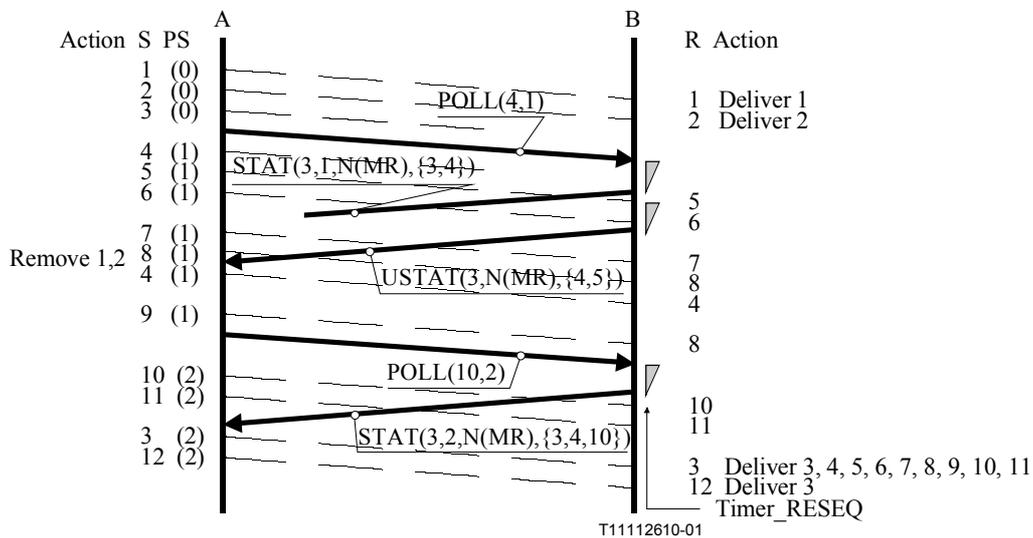
**Figure II.10/Q.2111 – Error recovery via STAT and USTAT PDUs with loss of a STAT PDU**
