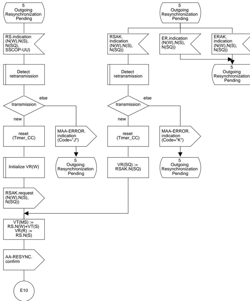
Figure 22/Q.2111 – SDL diagram of the multilink SSCOPMCE protocol entity (sheet 12 of 38)
