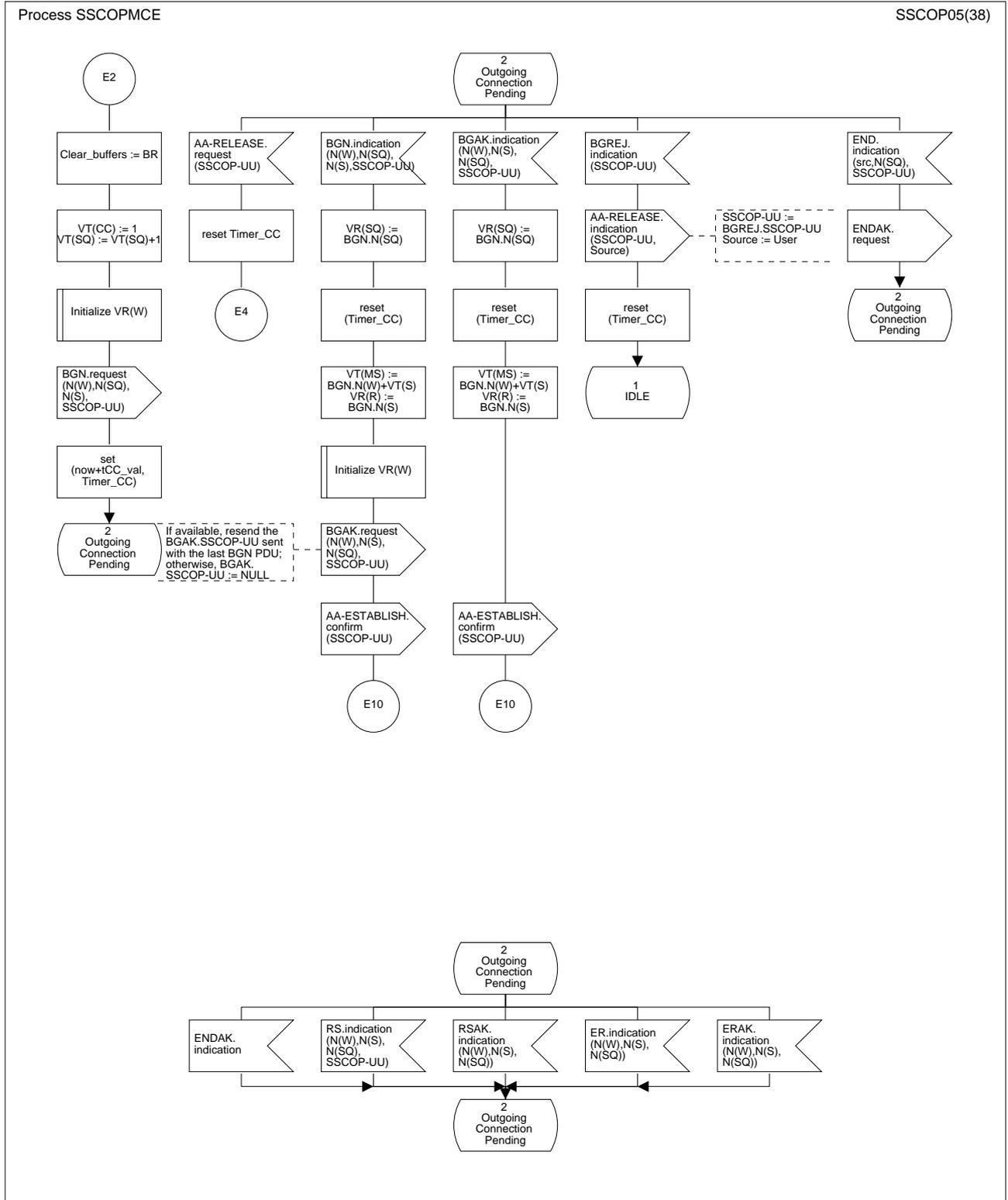
Figure 22/Q.2111 – SDL diagram of the multilink SSCOPMCE protocol entity (sheet 5 of 38)
