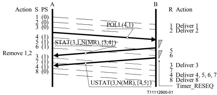
**Figure II.9/Q.2111 – Error recovery via STAT and USTAT PDU of the last transmitted SD PDUs**
