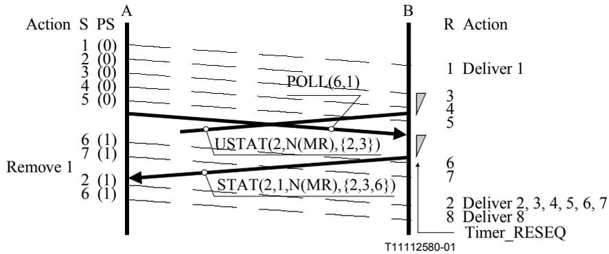
**Figure II.7/Q.2111 – Error recovery via STAT PDU**
