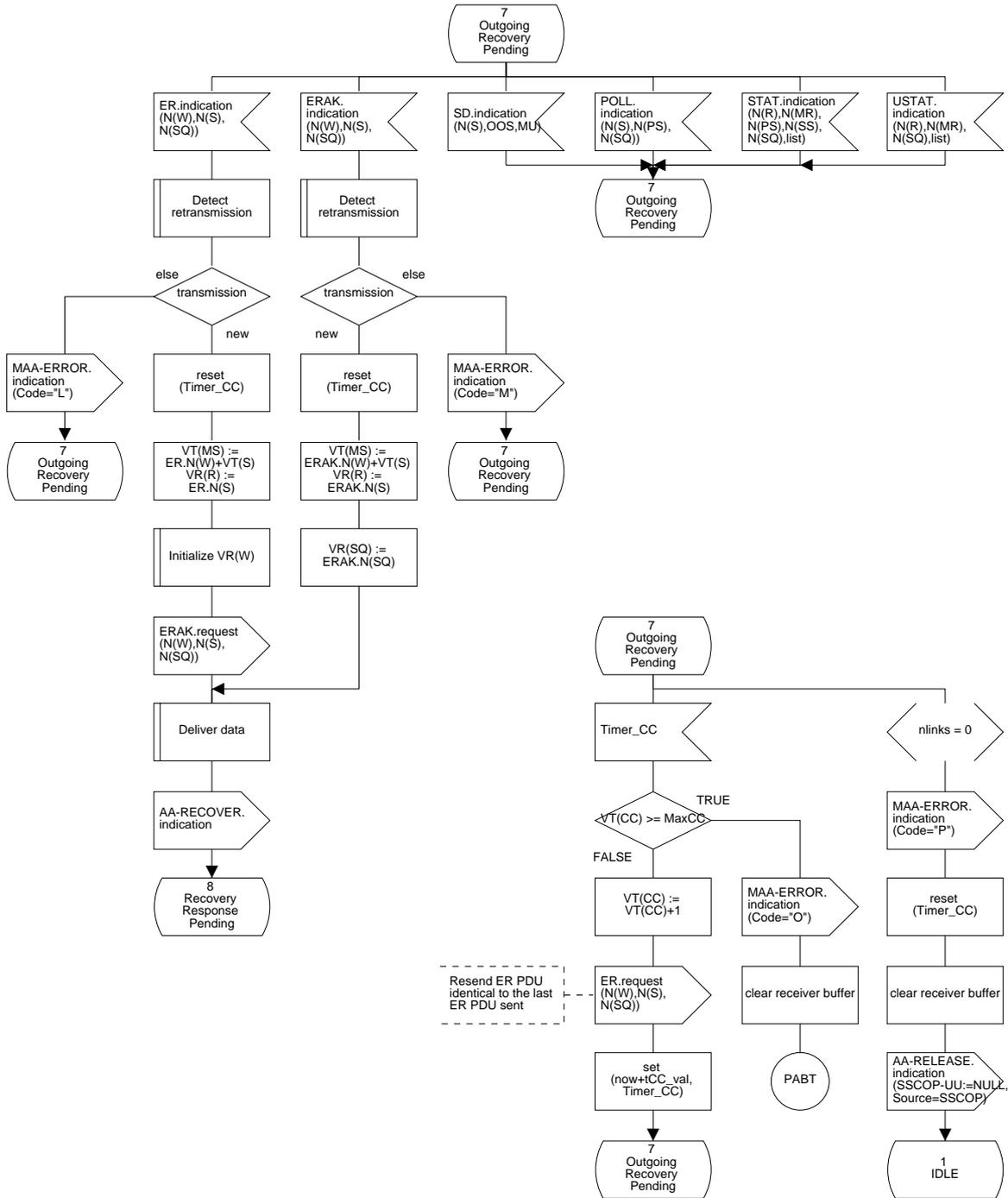
Figure 22/Q.2111 – SDL diagram of the multilink SSCOPMCE protocol entity (sheet 17 of 38)
