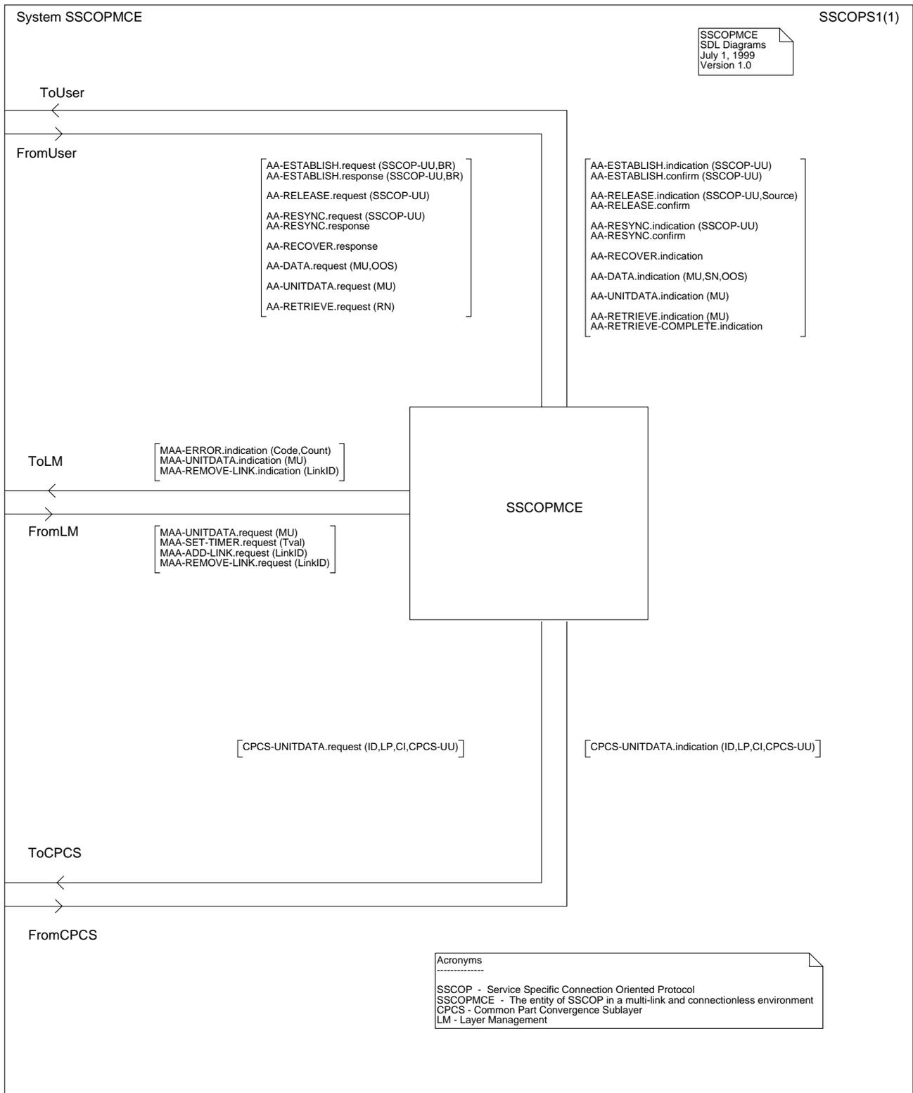
**Figure 20/Q.2111 – SDL system of the multilink SSCOPMCE protocol entity**
