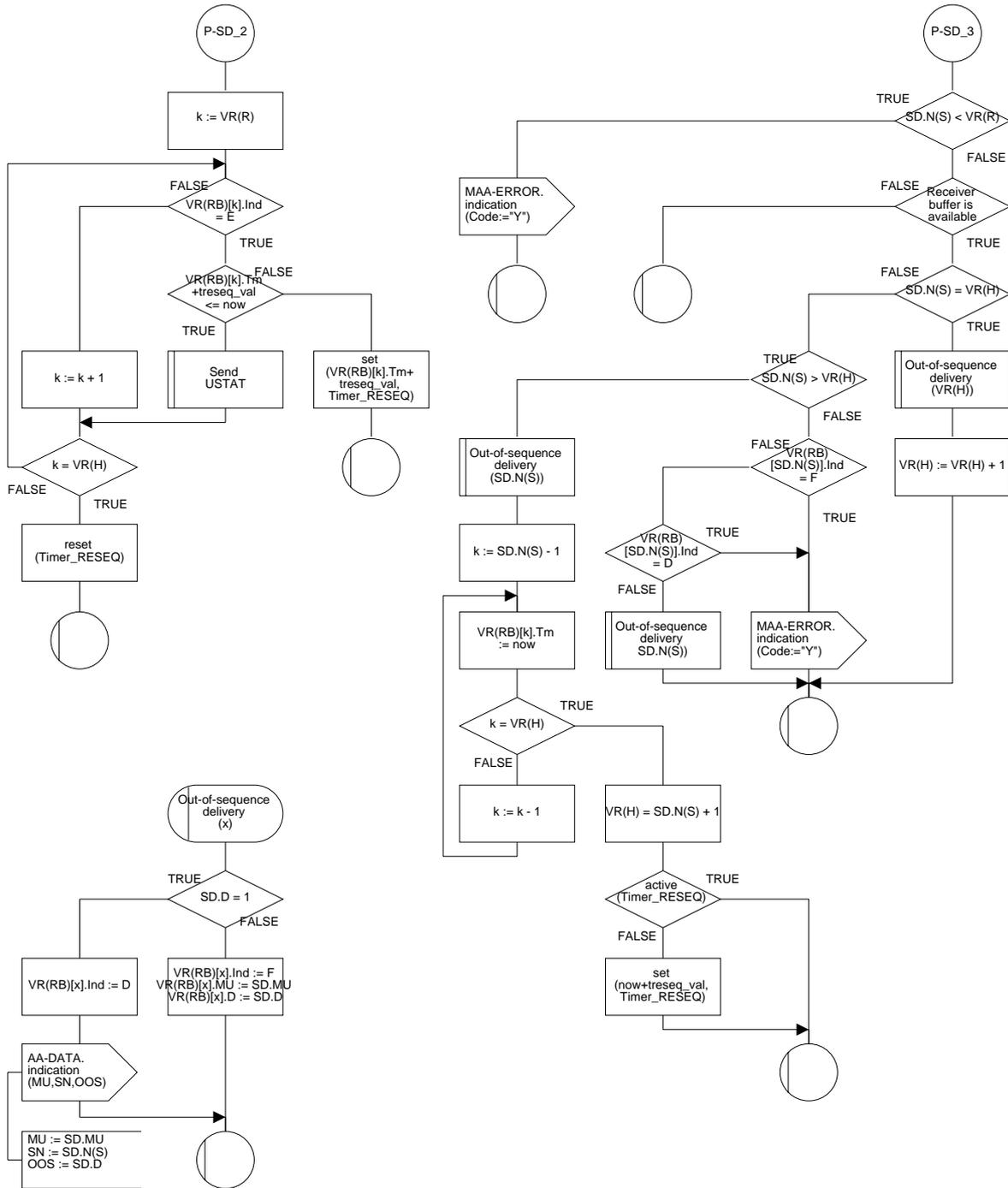
Figure 22/Q.2111 – SDL diagram of the multilink SSCOPMCE protocol entity (sheet 32 of 38)
