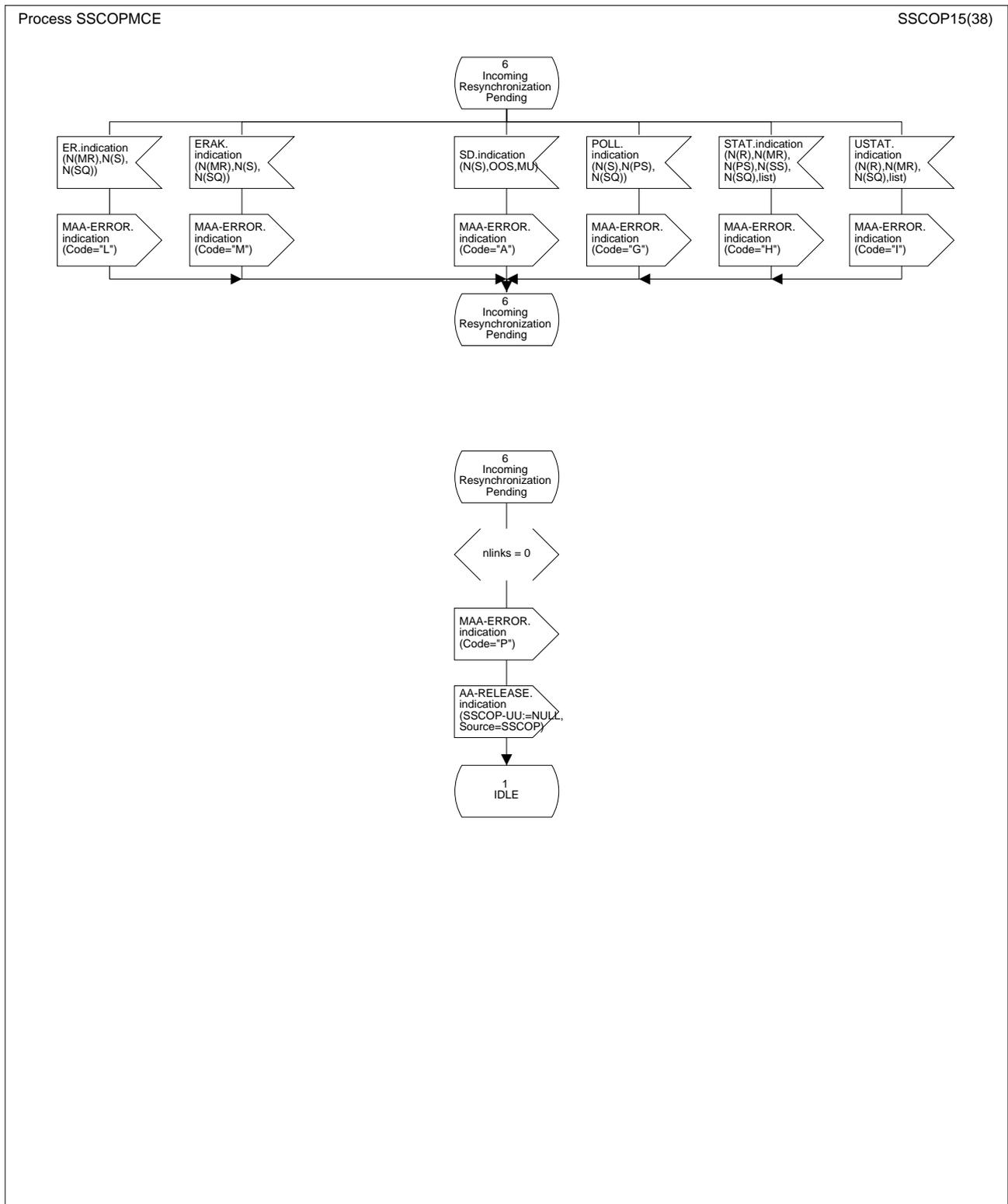
Figure 22/Q.2111 – SDL diagram of the multilink SSCOPMCE protocol entity (sheet 15 of 38)
