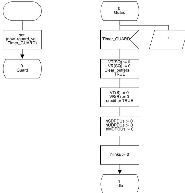
Figure 22/Q.2111 – SDL diagram of the multilink SSCOPMCE protocol entity (sheet 2 of 38)
