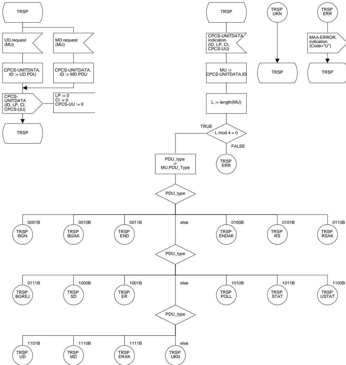
Figure B.1/Q.2111 – SDL diagram of the ancillary process TRSP (sheet 2 of 4)
