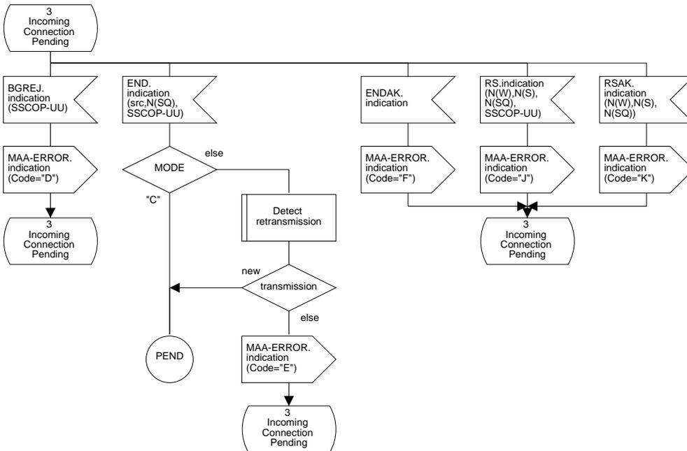
Figure 22/Q.2111 – SDL diagram of the multilink SSCOPMCE protocol entity (sheet 7 of 38)
