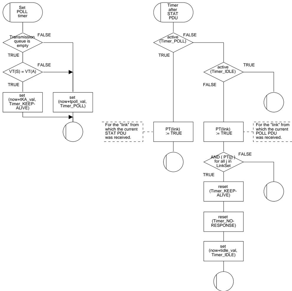
Figure 22/Q.2111 – SDL diagram of the multilink SSCOPMCE protocol entity (sheet 28 of 38)
