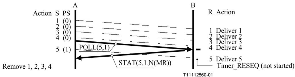
**Figure II.5/Q.2111 – Operation in the error-free case**
