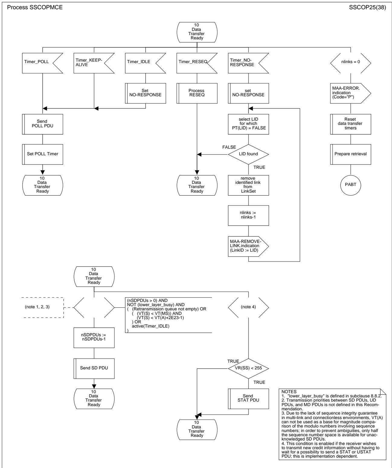
Figure 22/Q.2111 – SDL diagram of the multilink SSCOPMCE protocol entity (sheet 25 of 38)
