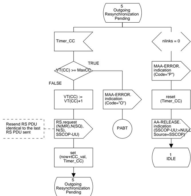
Figure 22/Q.2111 – SDL diagram of the multilink SSCOPMCE protocol entity (sheet 13 of 38)
