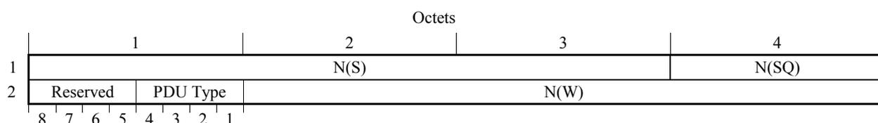
**Figure 12/Q.2111 – Error recovery PDU (ER PDU)**
