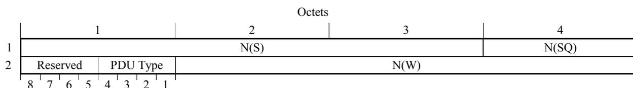
**Figure 11/Q.2111 – Resynchronization acknowledge PDU (RSAK PDU)**
