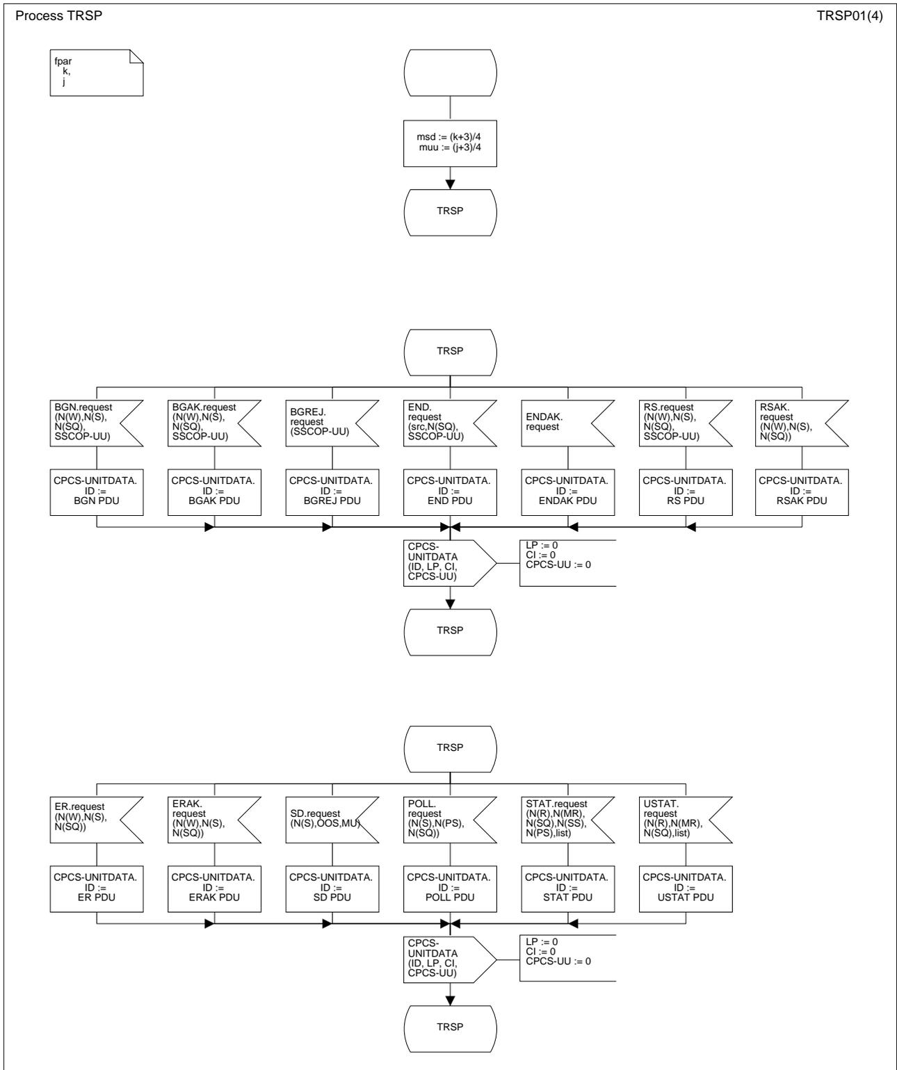
Figure B.1/Q.2111 – SDL diagram of the ancillary process TRSP (sheet 1 of 4)
