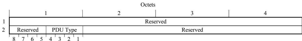
**Figure 9/Q.2111 – End acknowledge PDU (ENDAK PDU)**
