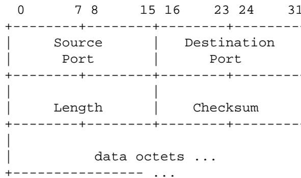
**Figure C.4/Q.2111 – UDP header format**
