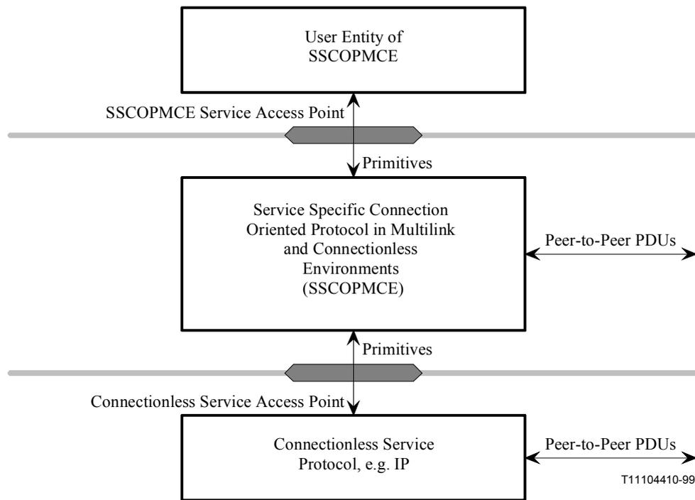
**Figure 3/Q.2111 – SSCOPMCE in a connectionless environment**
