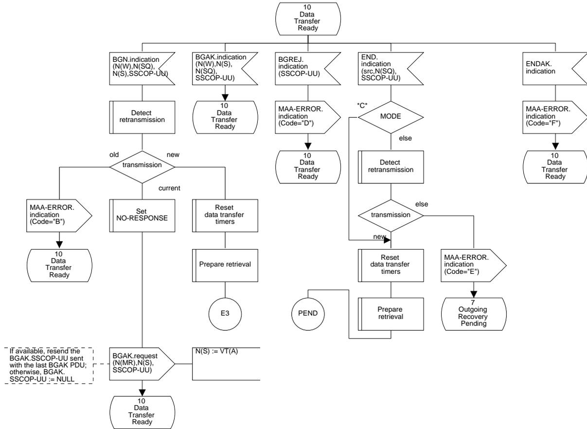
Figure 22/Q.2111 – SDL diagram of the multilink SSCOPMCE protocol entity (sheet 23 of 38)
