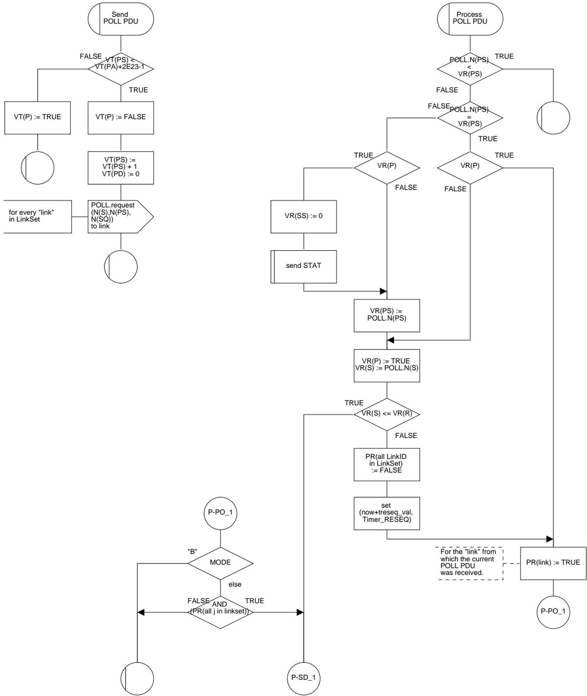
Figure 22/Q.2111 – SDL diagram of the multilink SSCOPMCE protocol entity (sheet 33 of 38)
