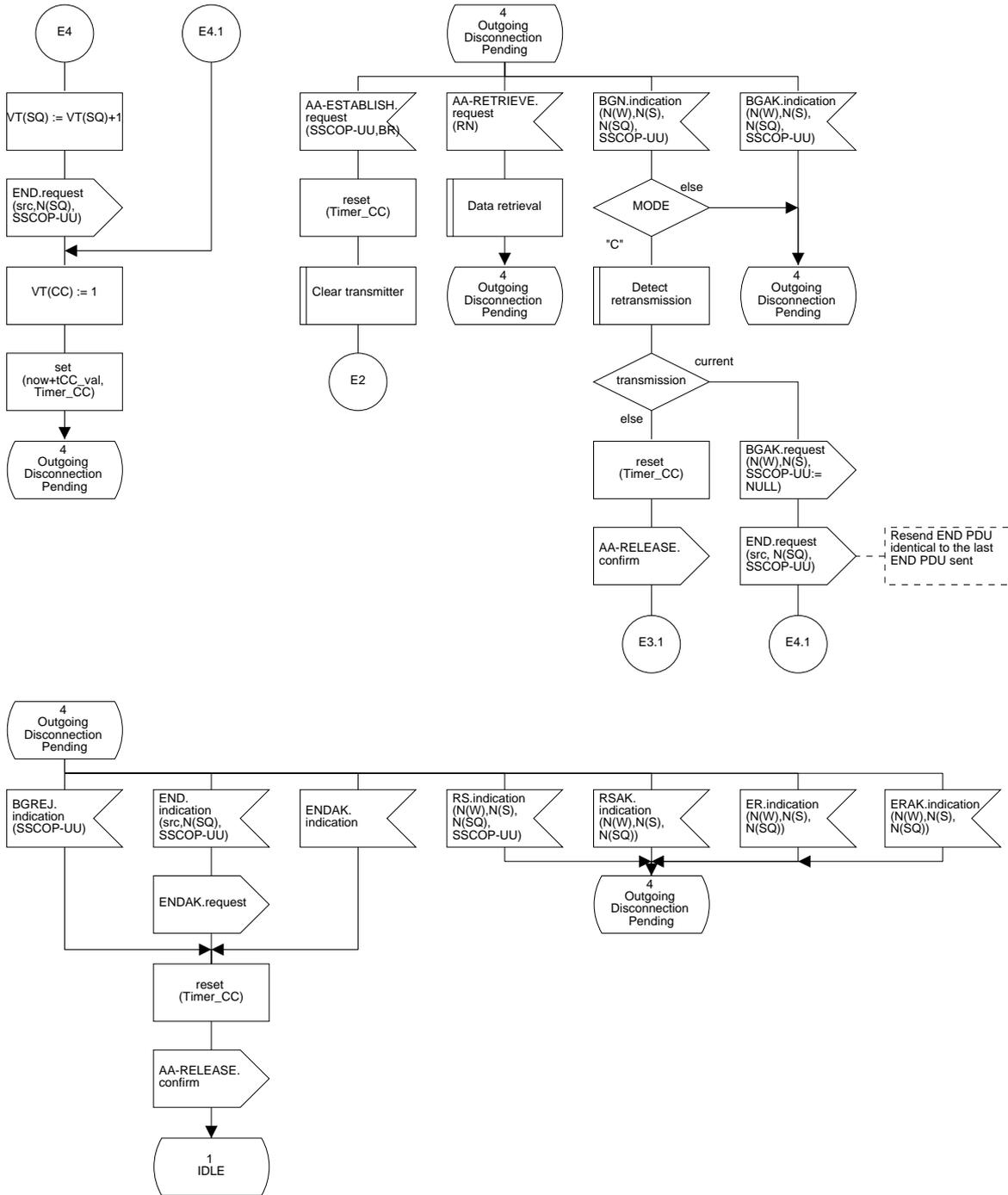
Figure 22/Q.2111 – SDL diagram of the multilink SSCOPMCE protocol entity (sheet 9 of 38)
