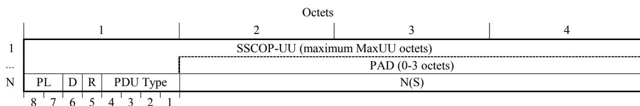
**Figure 14/Q.2111 – Sequenced data PDU (SD PDU)**
