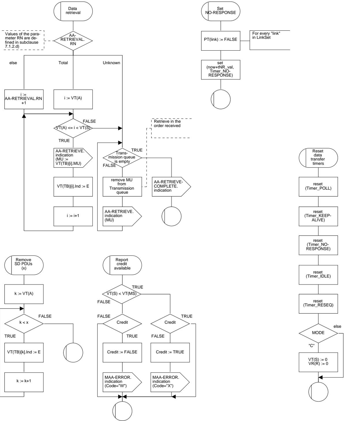
Figure 22/Q.2111 – SDL diagram of the multilink SSCOPMCE protocol entity (sheet 29 of 38)
