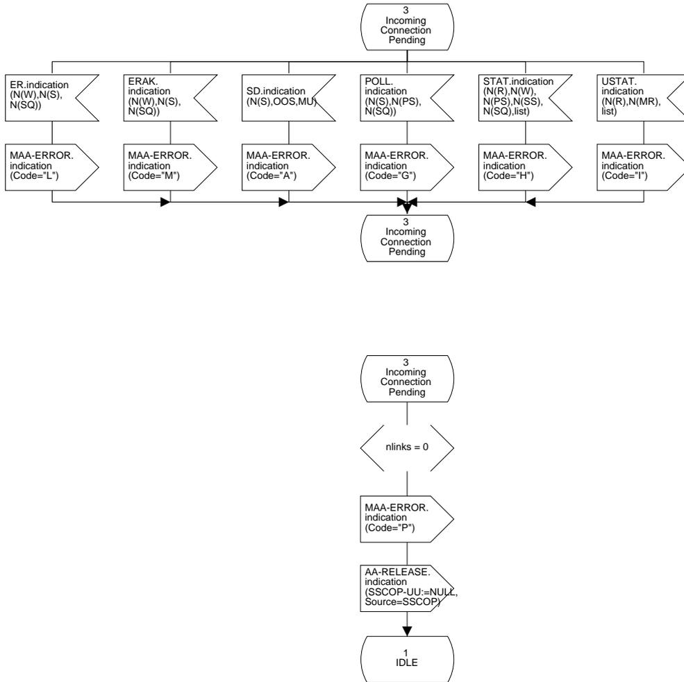
Figure 22/Q.2111 – SDL diagram of the multilink SSCOPMCE protocol entity (sheet 8 of 38)
