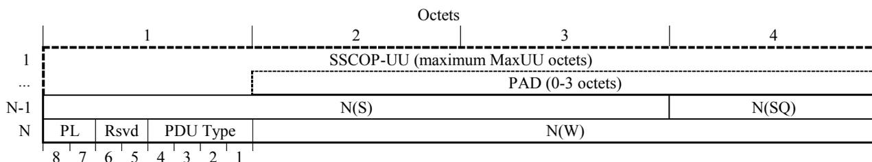
**Figure 10/Q.2111 – Resynchronization PDU (RS PDU)**
