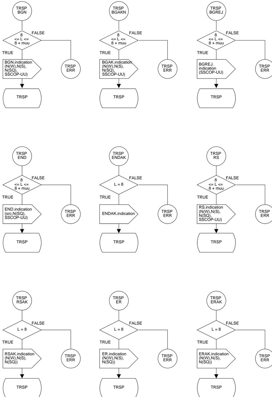
Figure B.1/Q.2111 – SDL diagram of the ancillary process TRSP (sheet 3 of 4)
