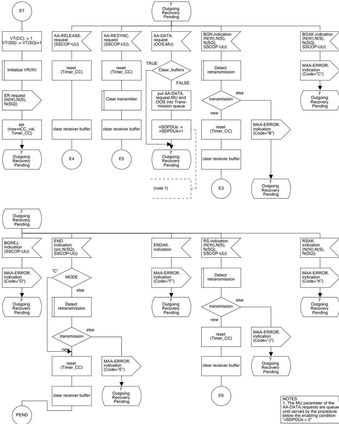
Figure 22/Q.2111 – SDL diagram of the multilink SSCOPMCE protocol entity (sheet 16 of 38)
