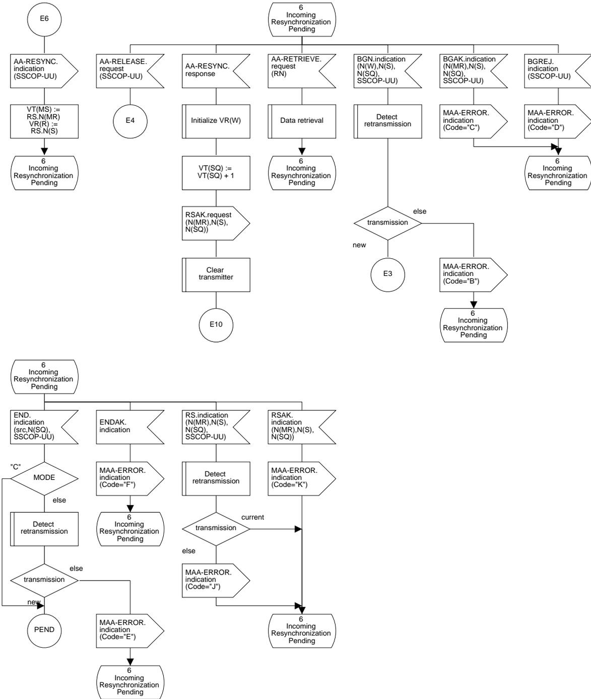
Figure 22/Q.2111 – SDL diagram of the multilink SSCOPMCE protocol entity (sheet 14 of 38)
