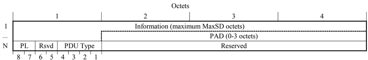
**Figure 18/Q.2111 – Unnumbered data PDU (UD PDU) or Management data PDU (MD PDU)**
