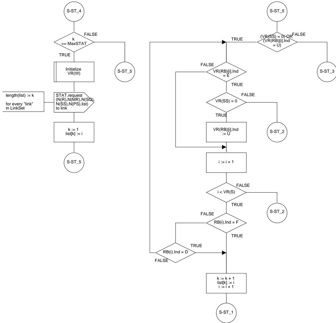
Figure 22/Q.2111 – SDL diagram of the multilink SSCOPMCE protocol entity (sheet 35 of 38)
