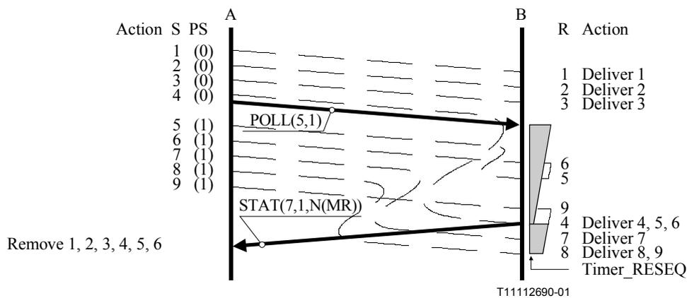
**Figure II.18/Q.2111 – Acknowledgment of SD PDUs received after a POLL PDU with missing sequence of SD PDUs**
