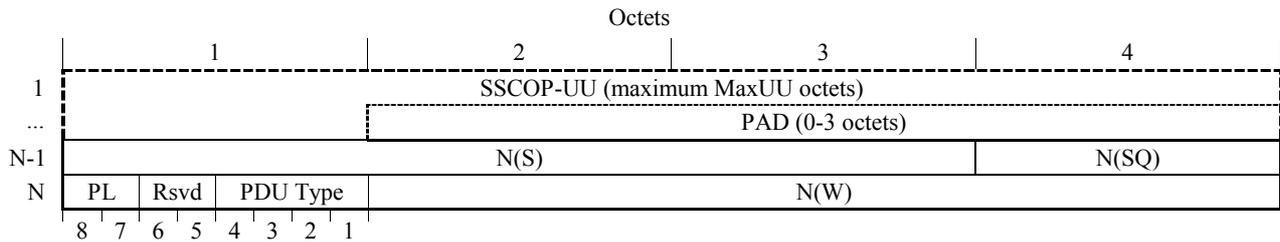
**Figure 6/Q.2111 – Begin acknowledge PDU (BGAK PDU)**
