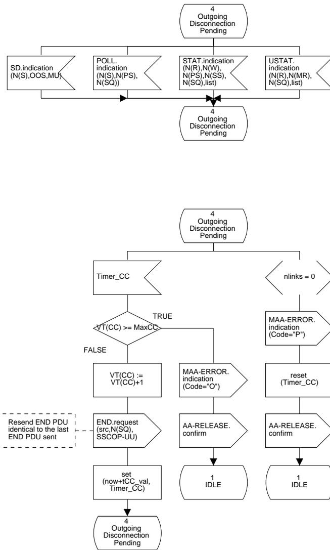
Figure 22/Q.2111 – SDL diagram of the multilink SSCOPMCE protocol entity (sheet 10 of 38)
