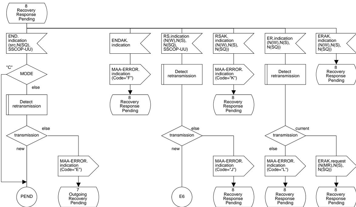
Figure 22/Q.2111 – SDL diagram of the multilink SSCOPMCE protocol entity (sheet 18 of 38)
