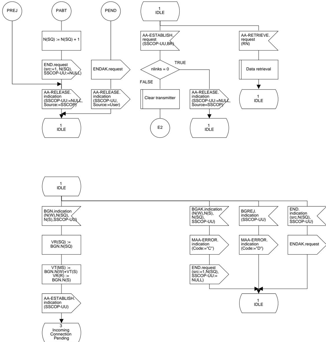
Figure 22/Q.2111 – SDL diagram of the multilink SSCOPMCE protocol entity (sheet 3 of 38)
