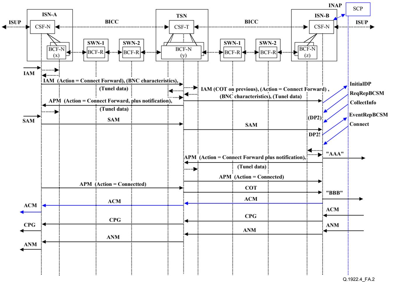
Figure A.2/Q.1922.4 – IN call with SCP request to collect further digits & per-call bearer set-up using bearer information transport tunnel – fast set-up (forward)
