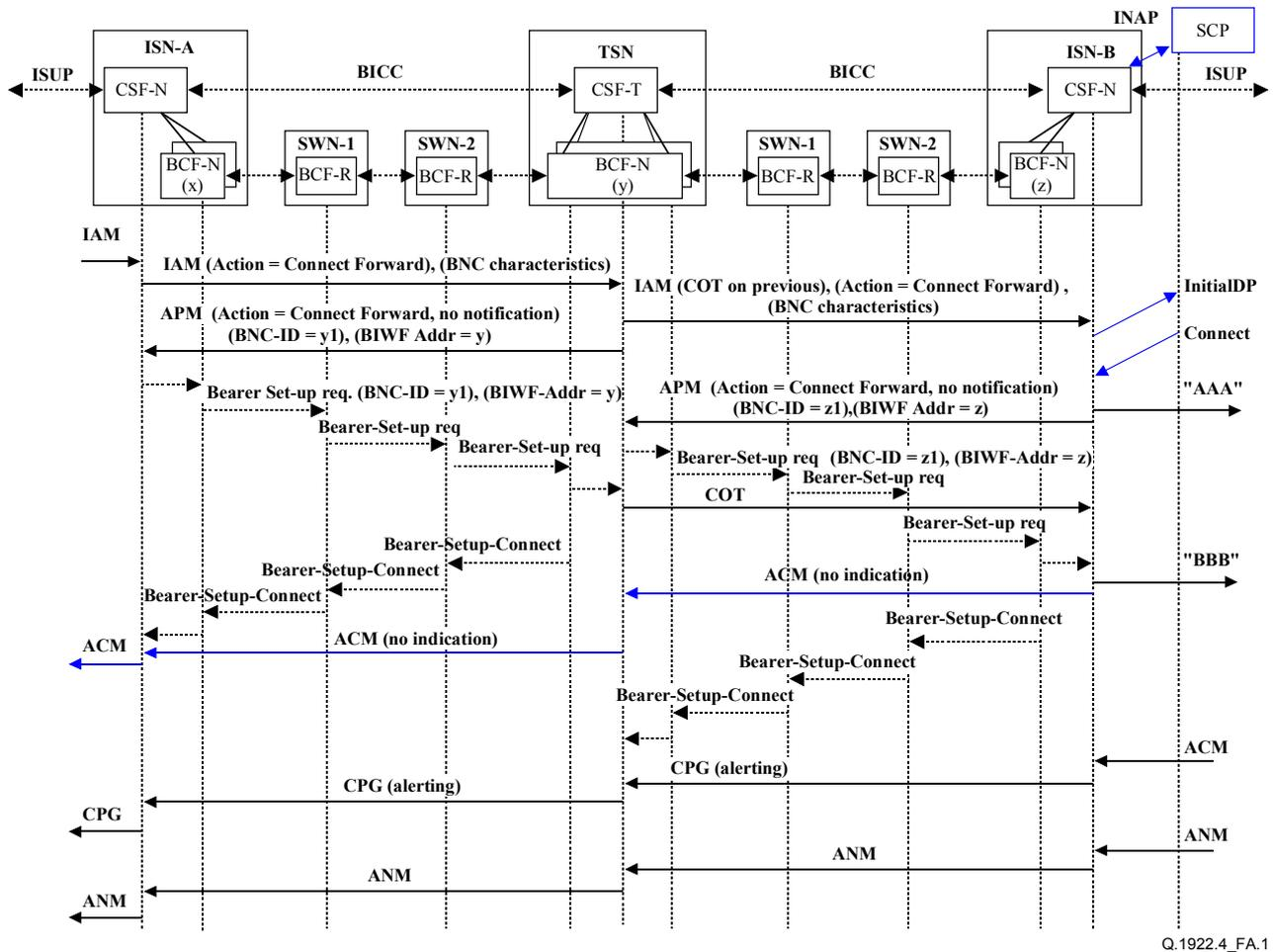
Figure A.1/Q.1922.4 – IN basic call for a call with forward establishment of backbone network connection
