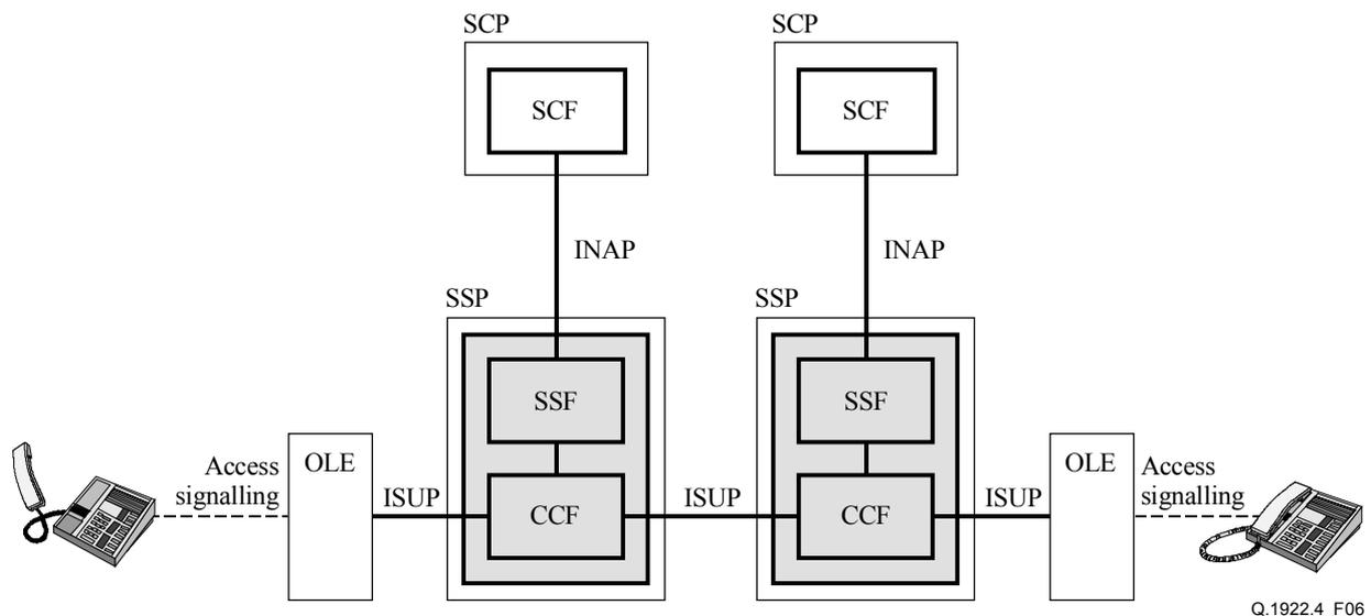
**Figure 6/Q.1922.4 – Configuration with two SSPs involved in the call**
