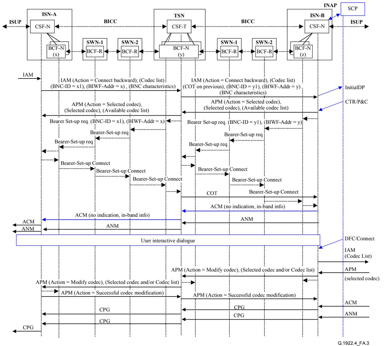
**Figure A.3/Q.1922.4 – IN call with user interactive dialogue (in-band) & Backward establishment of backbone network connection, with Codec negotiation**
