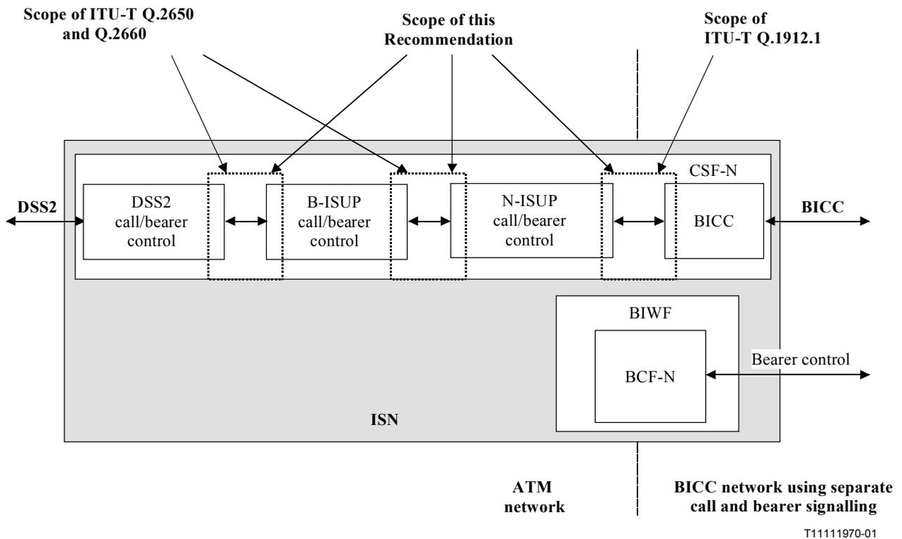
Figure 1/Q.1912.4 – Scope of this Recommendation for BICC/DSS2 interworking
