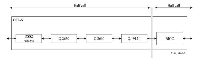
Figure 2/Q.1912.4 – Functional description of the interworking configuration
