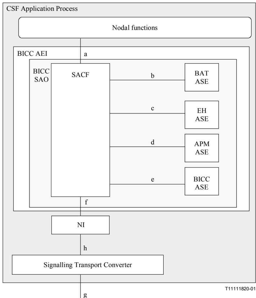
**Figure 1/Q.1902.5 – BICC specification model**
