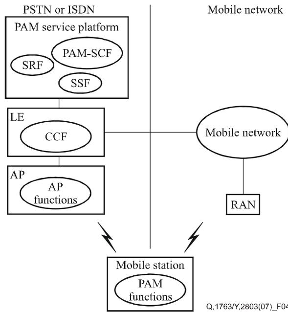
**Figure 4 – Scenario for assigning functional entities to the same physical node when using a discrete PAM service number**
