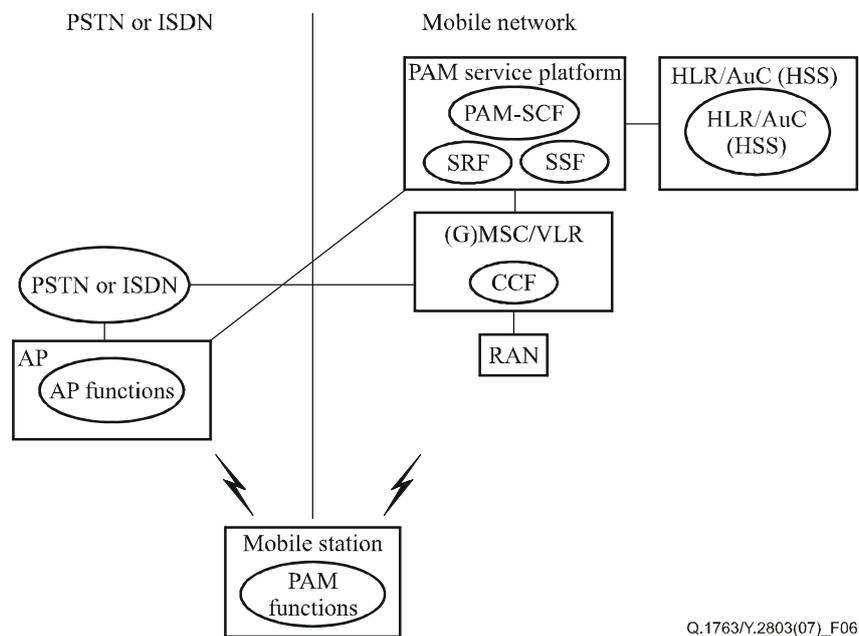
**Figure 6 – Scenario for assigning FEs to the same physical node when using MSISDN as the PAM service number**
