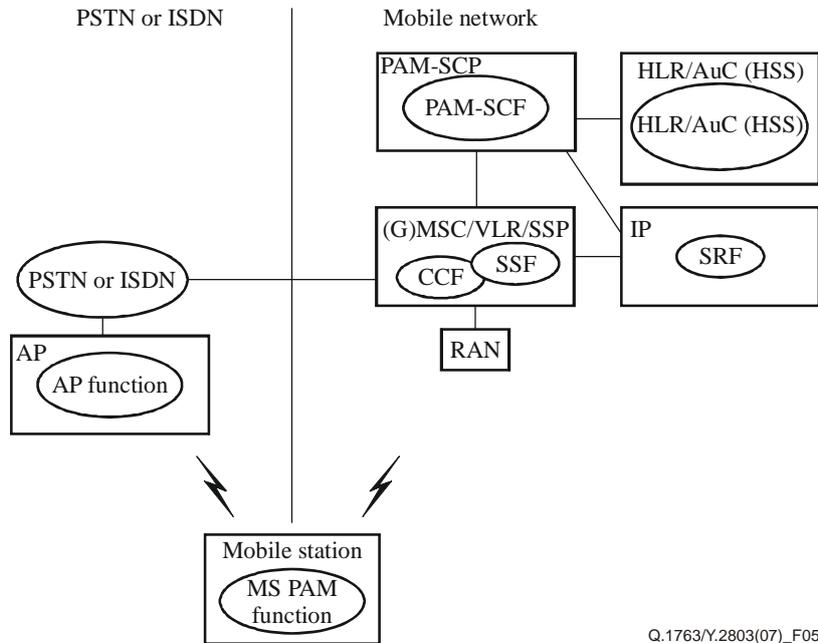
**Figure 5 – Scenario for assigning FEs to different physical nodes when using MSISDN as the PAM service number**
