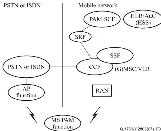
**Figure 2 – The functional model of the PAM service using a MSISDN as the PAM service number**
