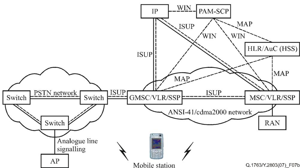
**Figure 7b – The network configuration of the PAM service using MSISDN as the PAM service number for an ANSI-41/cdma2000 mobile network**
