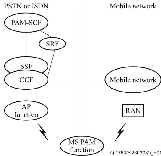
**Figure 1 – The functional model of the PAM service using a discrete PAM service number**
