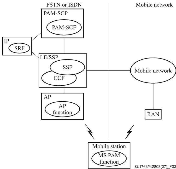
**Figure 3 – Scenario for assigning FEs to different physical nodes when using a discrete PAM service number**
