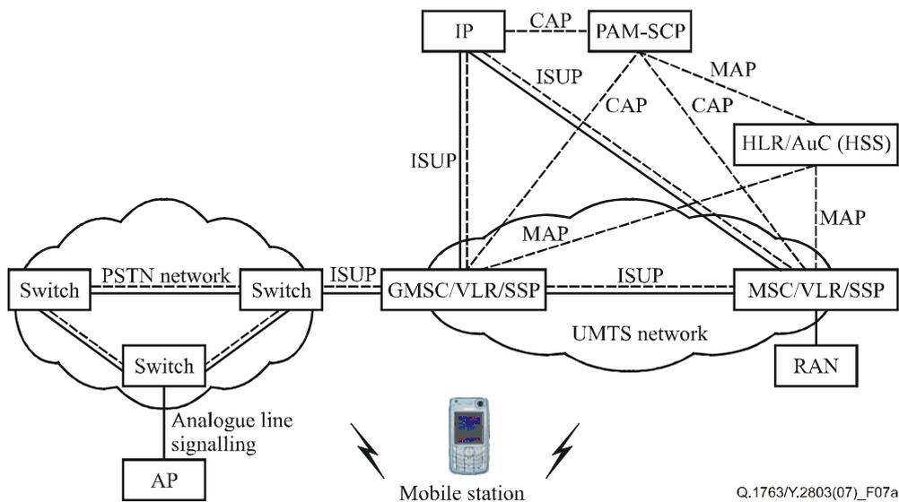
**Figure 7a – The network configuration of the PAM service using MSISDN as the PAM service number for a GSM/UTRAN mobile network**
