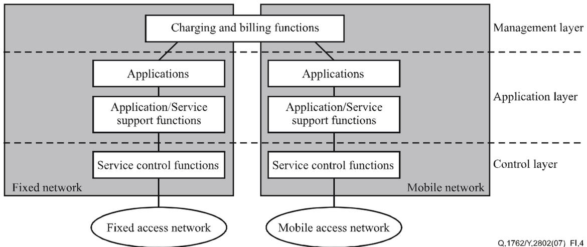
**Figure I.4 – Scenario: Convergence in charging and billing functions**
