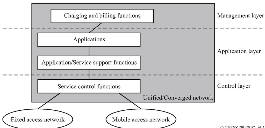
**Figure I.1 – Scenario: Convergence in service control functions**
