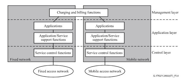
Figure I.4 – Scenario: Convergence in charging and billing functions
