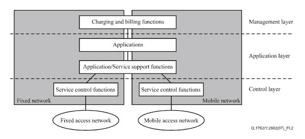
Figure I.2 – Scenario: Convergences in application/service support functions
