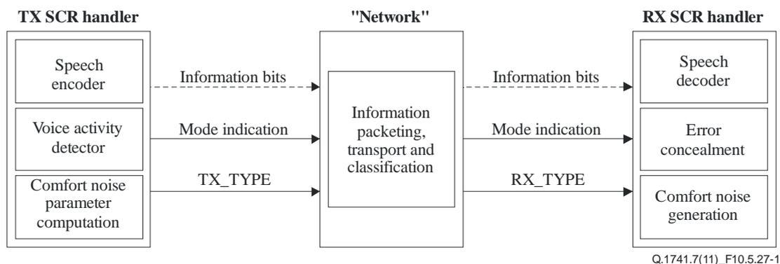
Figure 10.5.27-1 – Block diagram of one link SCR operation
