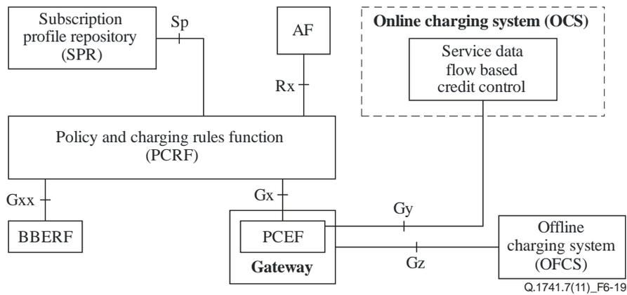
**Figure 6-19 – Overall PCC logical architecture (non-roaming)**
