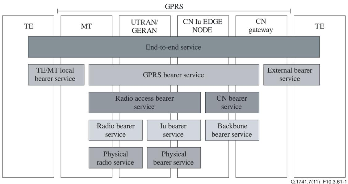
Figure 10.3.61-1 – End-to-end QoS architecture
