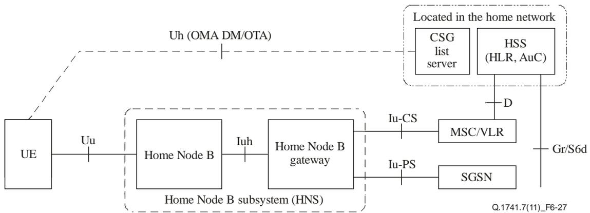
**Figure 6-27 – Configuration of PLMN supporting the home NodeB subsystem**
