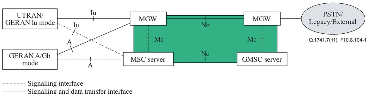
Figure 10.8.104-1 – CS core network logical architecture
