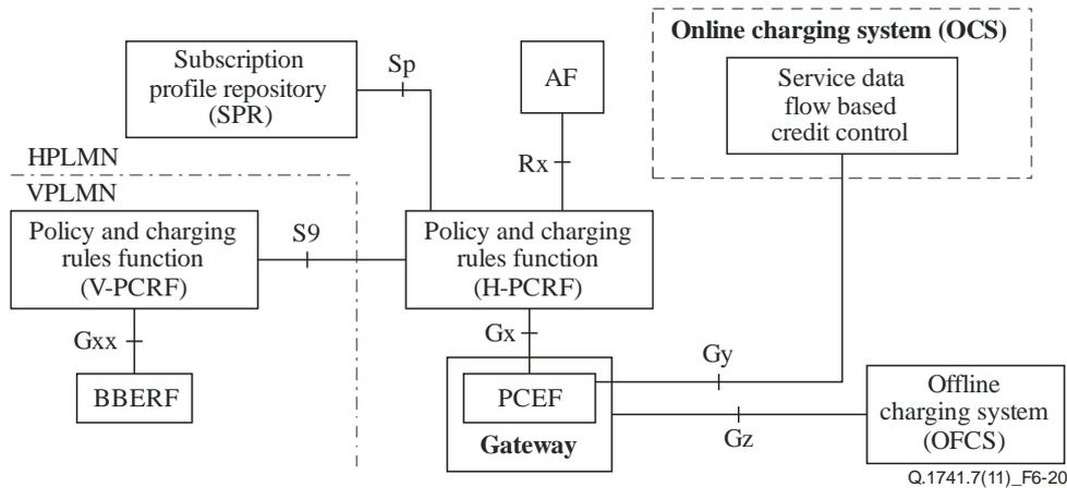
**Figure 6-20 – PCC architecture (roaming with home routed access)**
