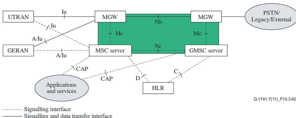
**Figure 10.3.60-1 – CS core network logical architecture**
