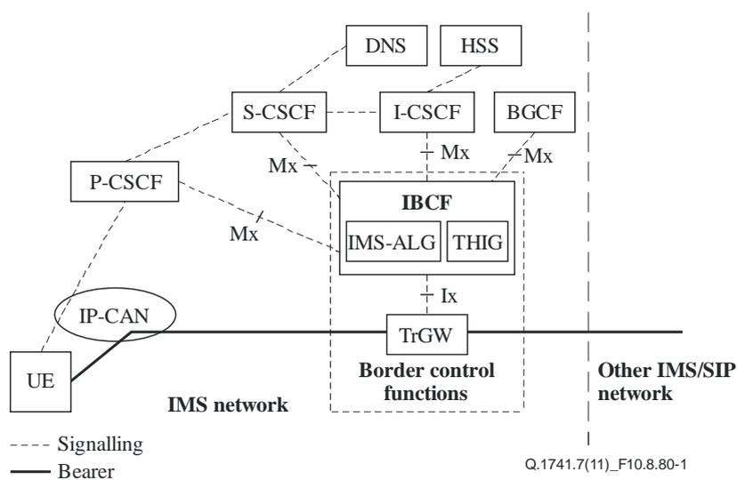
Figure 10.8.80-1 – Reference model for IMS Border Control Functions
