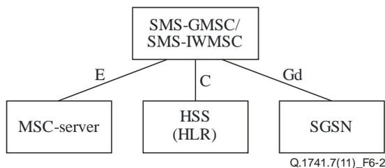
**Figure 6-2 – Configuration for Short Message Service**
