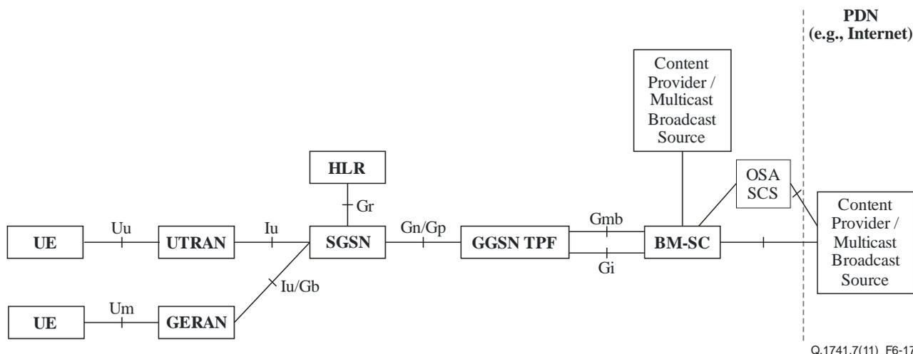
**Figure 6-17 – Configuration of MBMS entities for GPRS**
