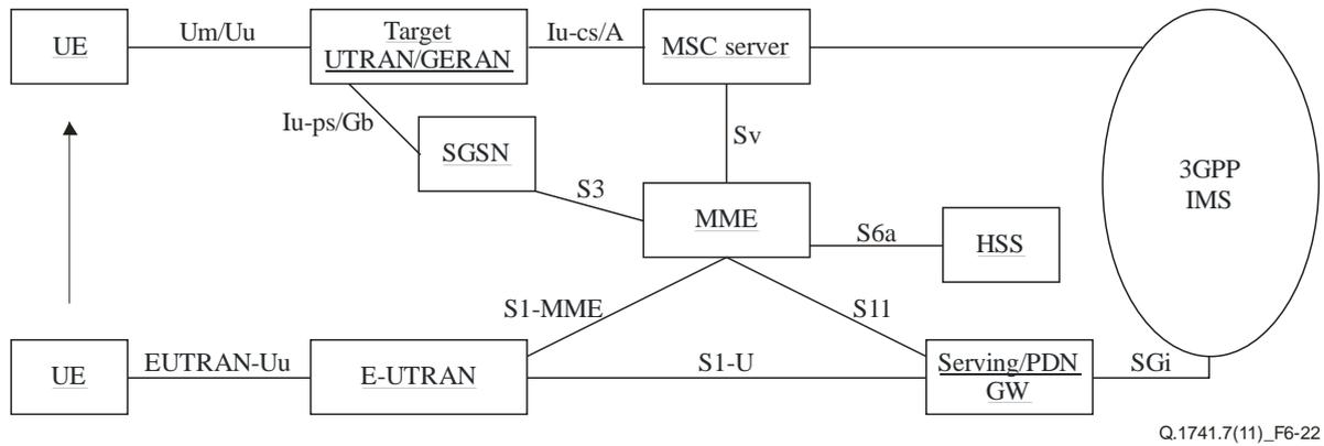
**Figure 6-22 – SRVCC architecture for E-UTRAN to 3GPP UTRAN/GERAN**
