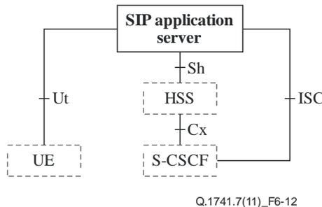
**Figure 6-12 – Functional architecture for the management of the user's service related information**
