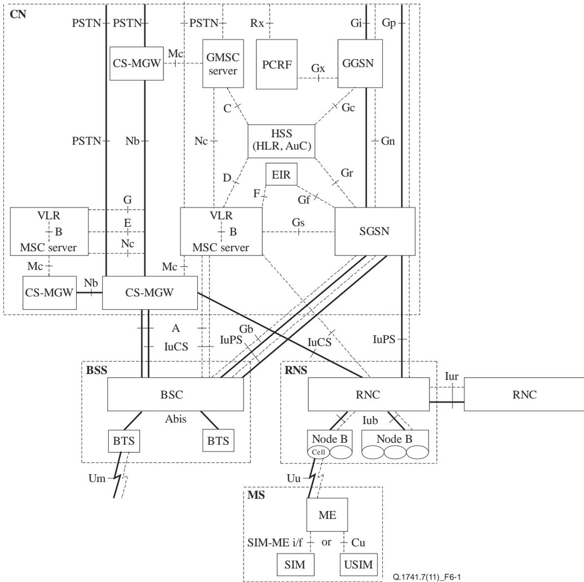
**Figure 6-1 – Basic Configuration of a PLMN supporting CS and PS (using GPRS) services and interfaces**
