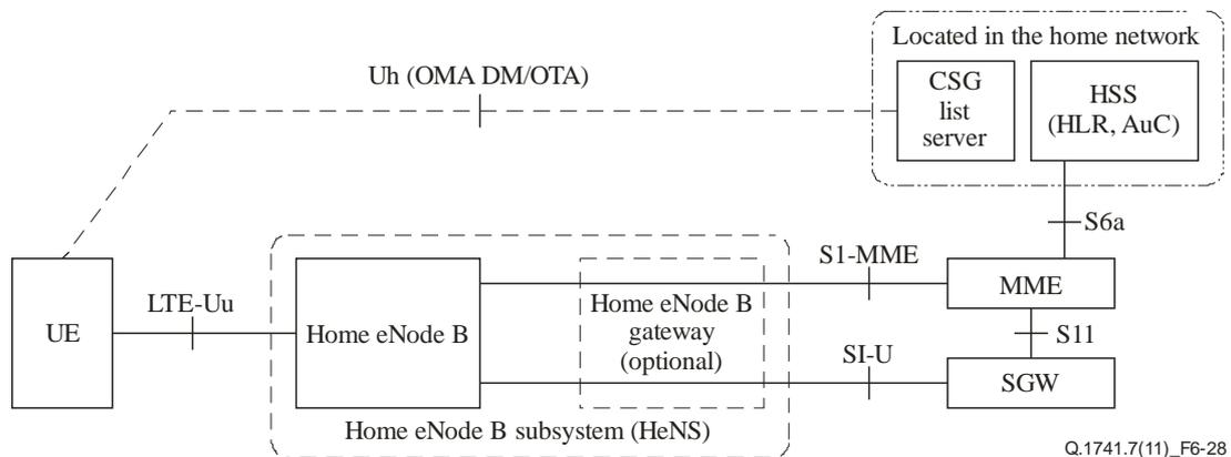
**Figure 6-28 – Configuration of PLMN supporting Home eNodeB Subsystem**
