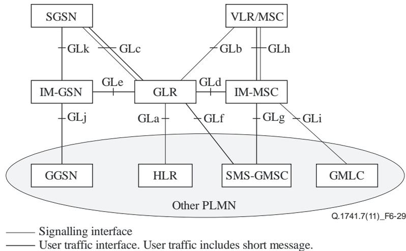
**Figure 6-29 – Configuration of a PLMN and interfaces with GLR**
