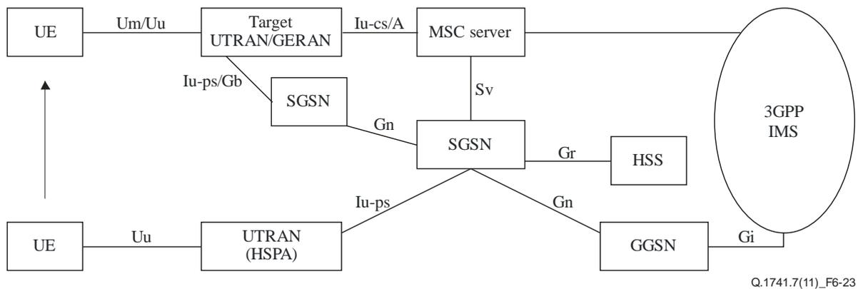
**Figure 6-23 – SRVCC architecture for UTRAN (HSPA) to 3GPP UTRAN/GERAN with Gn based SGSN**
