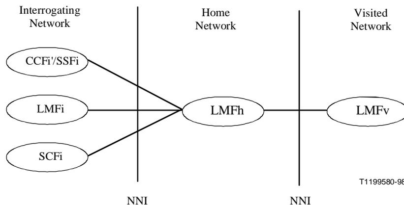
**Figure 7-6/Q.1711 – Network interconnection for retrieval of data for routing calls**
