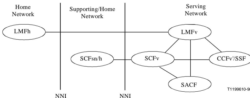
**Figure 7-8b/Q.1711 – VHE scenario: Relay Service Control
