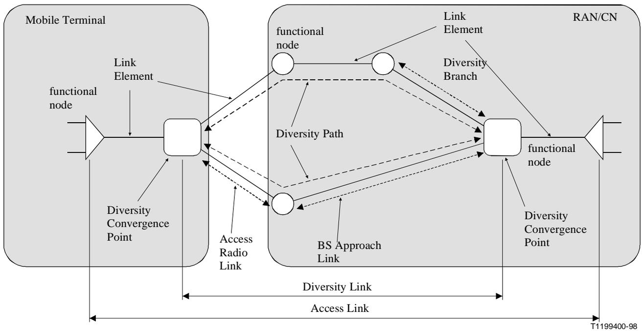
**Figure 3-2/Q.1711 – Naming of the elements associated with the MT-RAN/CN access related communication**
