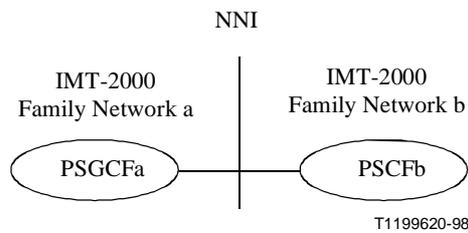
**Figure 7-9/Q.1711 – Network interconnection for packet data services**
