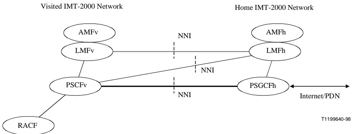
**Figure 7-11a/Q.1711 – Network interconnection scenario I for IMT-2000 packet data services: Using Internet Protocol addresses (either static or dynamic) assigned by the Home network**
