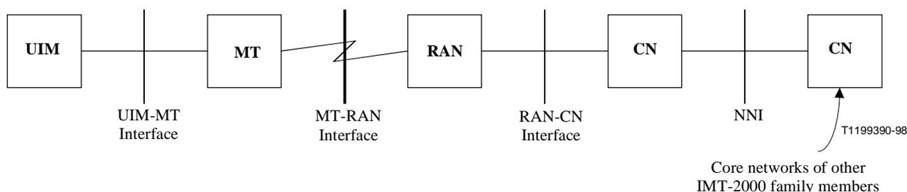
**Figure 3-1/Q.1711 – Physical interfaces of an IMT-2000 family member system**
