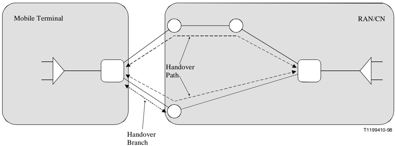
**Figure 3-3/Q.1711 – Naming of elements associated with diversity handover**
