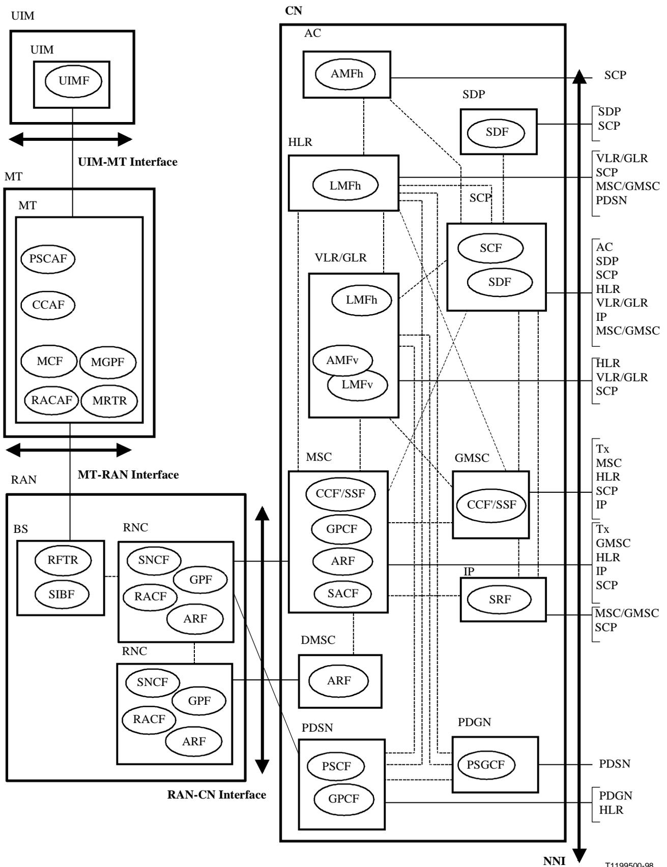
Figure 6-1a/Q.1711 – Generic reference model for IMT-2000 Alternative 1: Integrated call control and connection control FEs
