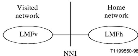
Figure 7-3/Q.1711 – Network interconnection for transfer of user data
