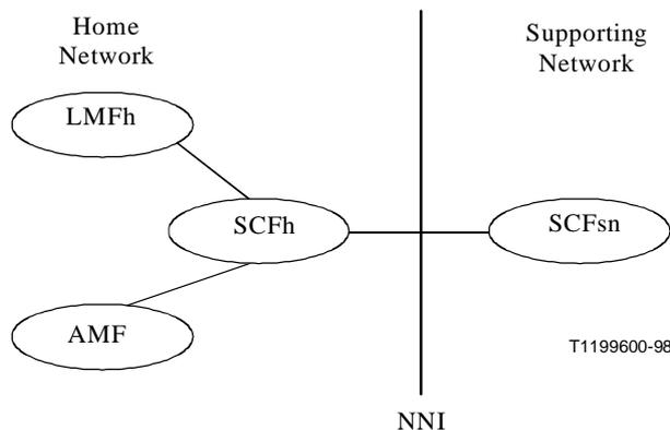
**Figure 7-8a/Q.1711 – VHE scenario: Relay Service Control
