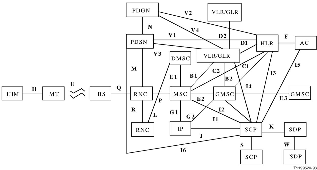
Figure 6-2/Q.1711 – Reference points in IMT-2000 reference model
