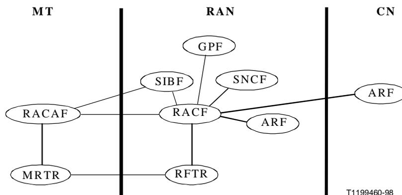
NOTE – The ARF FE has to be mapped to both the RAN and the CN subsystems, since a branch of a BS approach link can be set up via the RAN or via the CN.
