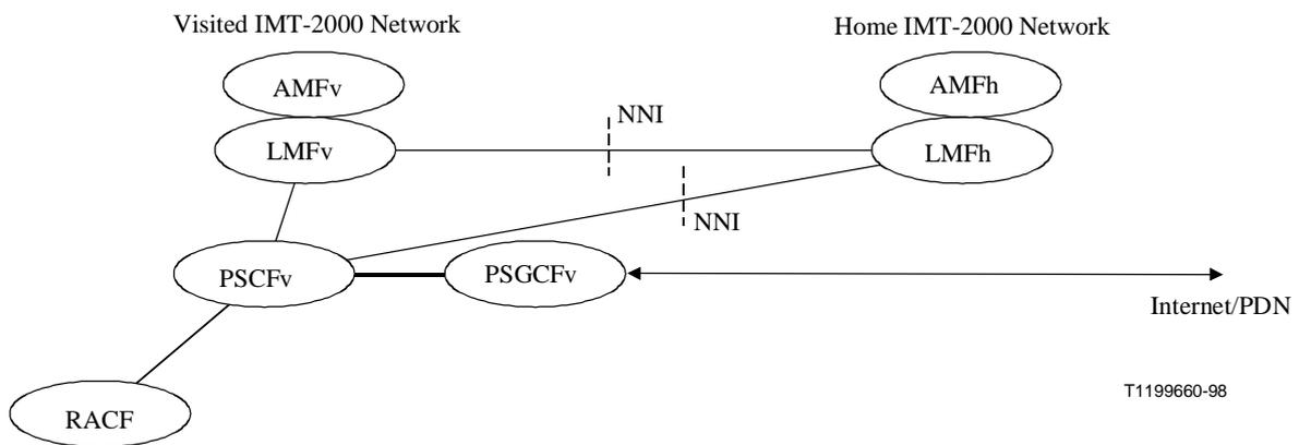
**Figure 7-12a/Q.1711 – Network interconnection scenario II for IMT-2000 packet data services: Using temporary Internet Protocol addresses assigned dynamically by the Visited network**
