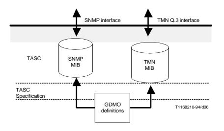
FIGURE 6/Q.1303 Combining SNMP and TMN representations
