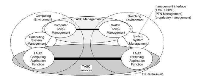
FIGURE 3/Q.1303 Functional representation of TASC Management architecture
