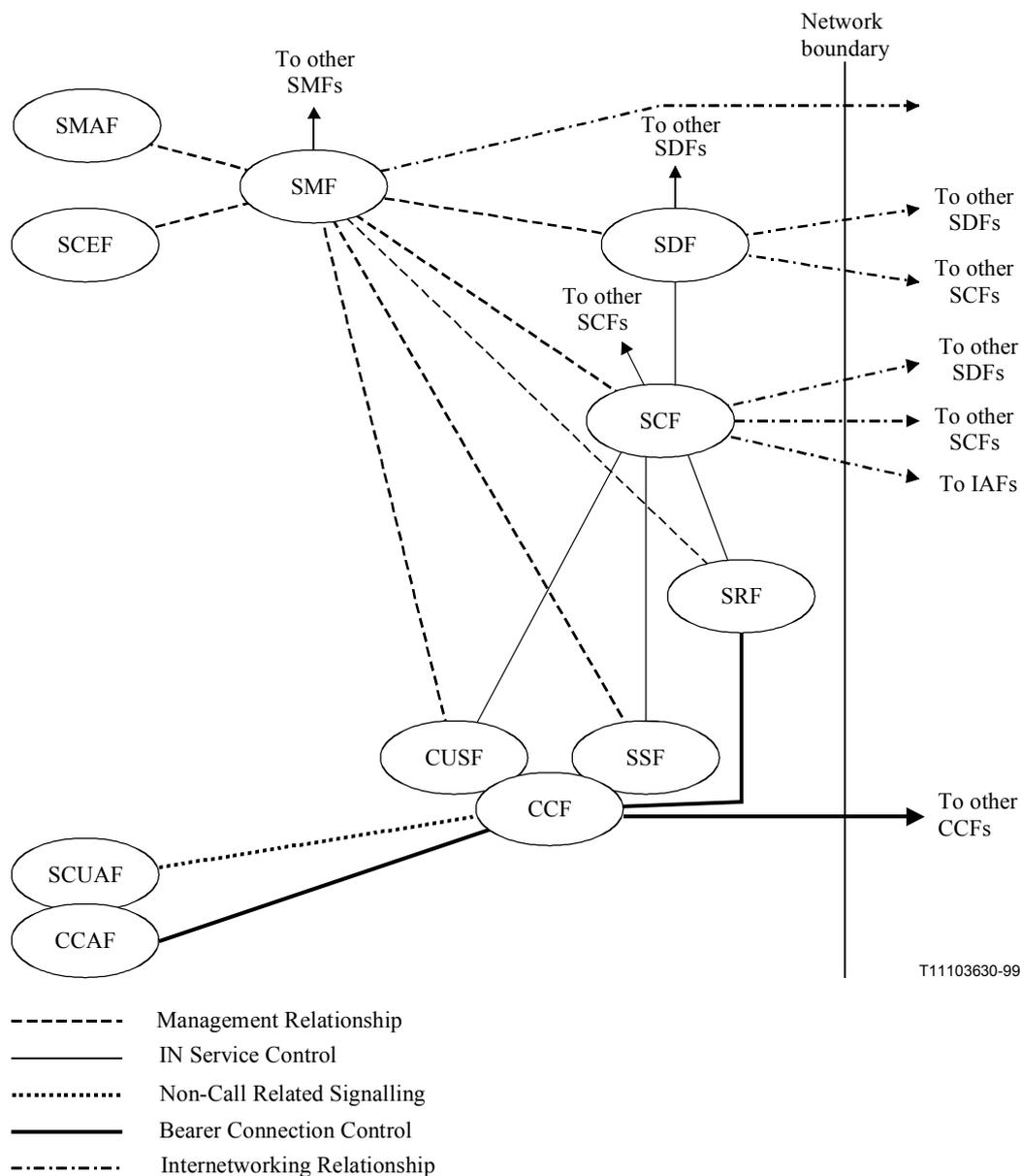
**Figure 1/Q.1241 – IN CS-4 DFP Architecture**
