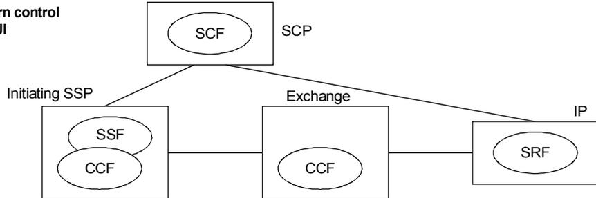
Case v) Hand-off: retain control at assisting SSP after UI completed
