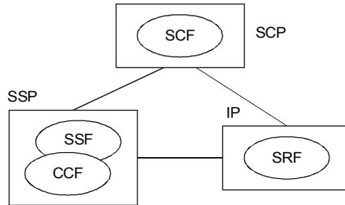
Case iii) Assist with relay; return control to initiating SSP on completion of UI
