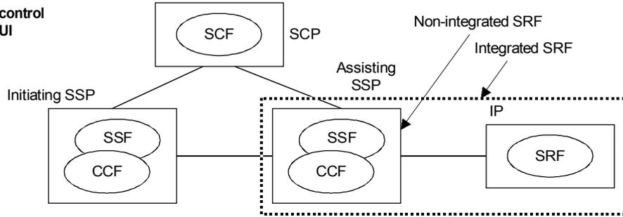
Case iv) Assist without relay: return control to initiating SSP on completion of UI
