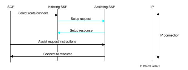
FIGURE 31/Q.1218 Preamble for hand-off case
