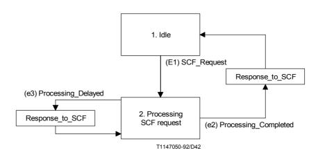
FIGURE 42/Q.1218 The SDF FSM
