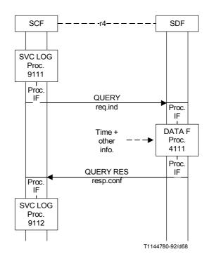
FIGURE 5-42/Q.1214 Information flow diagram "translate" SIB
