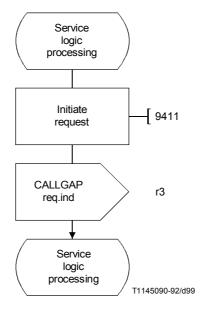
FIGURE 5-66/Q.1214 SCF actions for the call gap capability
