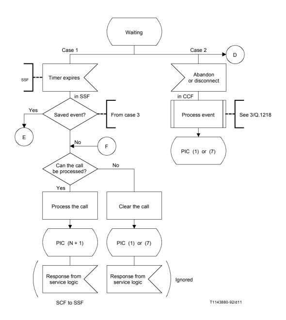
FIGURE 4-8/Q.1214 **Detection point processing**
