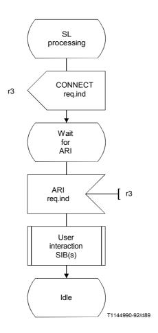
FIGURE 5-56/Q.1214 Service hand-off procedure actions at SCF
