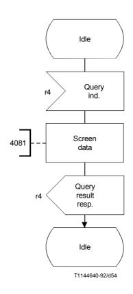
FIGURE 5-30/Q.1214 "Screen" SIB service data functional entity
