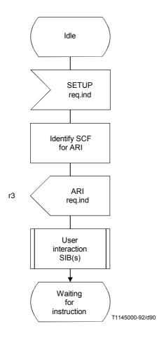
FIGURE 5-57/Q.1214 Service hand-off procedure actions at FE2/FE3
