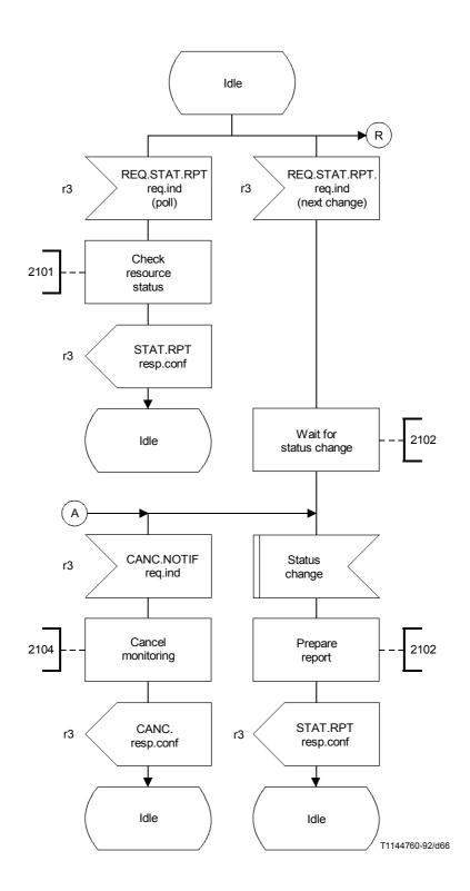
FIGURE 5-41/Q.1214 (sheet 1 of 2) "Status notification" SIB SSF/CCF
