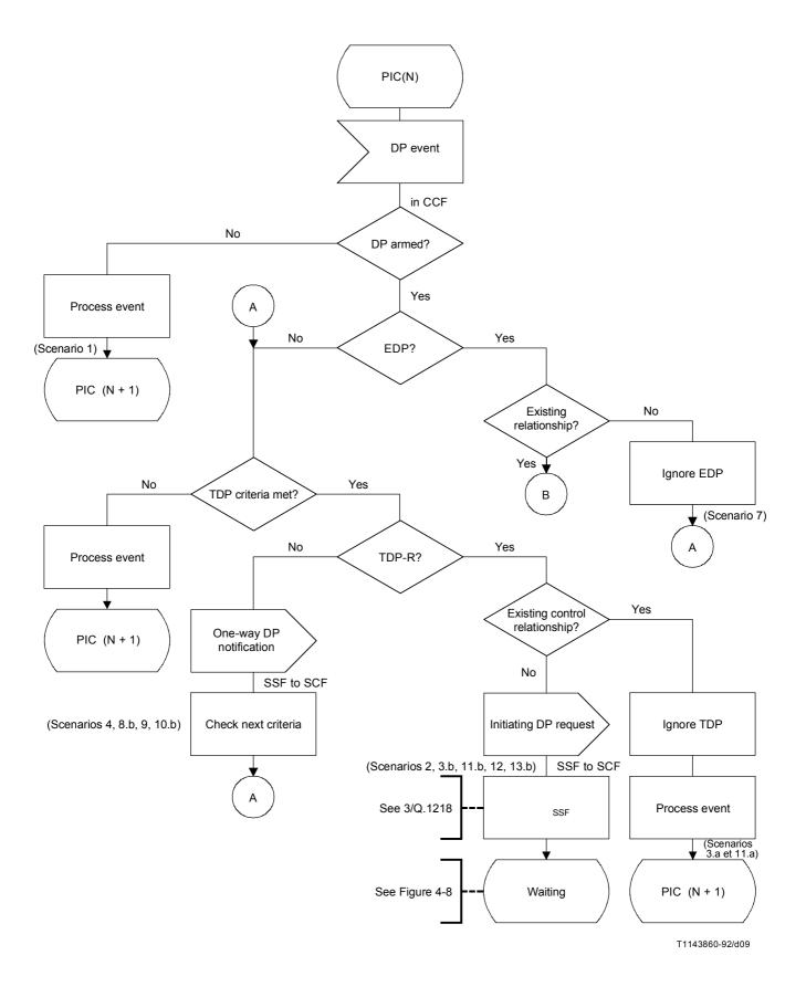
FIGURE 4-6/Q.1214 **Detection point processing**
