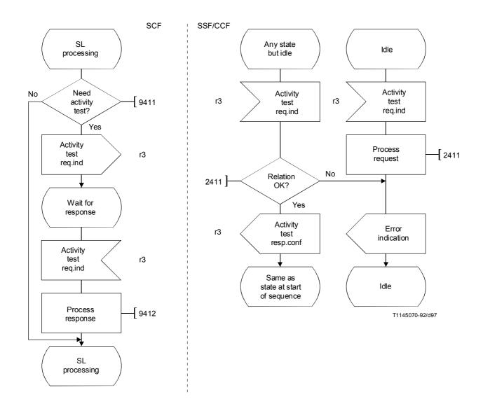
FIGURE 5-64/Q.1214 **SDLs for activity test**
