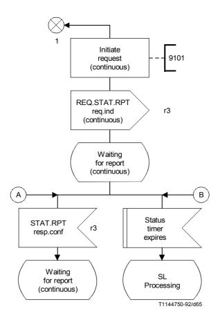
FIGURE 5-40/Q.1214 (sheet 2 of 2) "Status notification" SIB SCF
