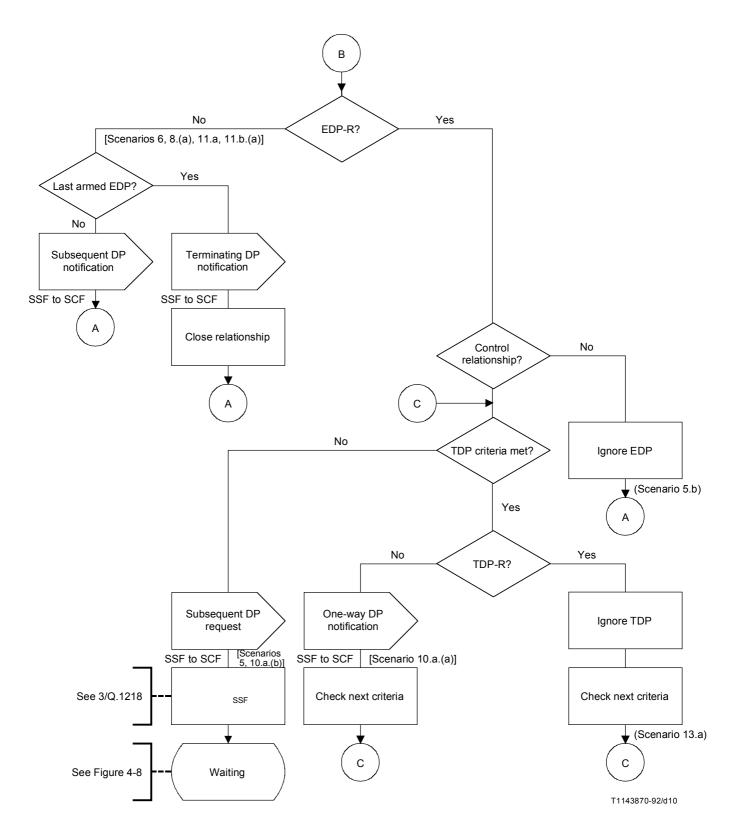
FIGURE 4-7/Q.1214 **Detection point processing**
