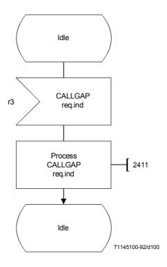
FIGURE 5-67/Q.1214 CCF/SSF actions for the call gap capability
