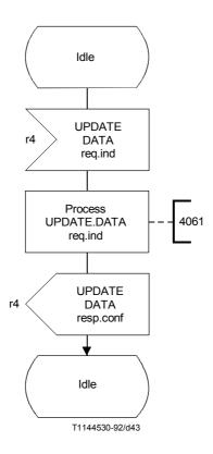
FIGURE 5-20/Q.1214 SDF actions for the "log call information" SIB
