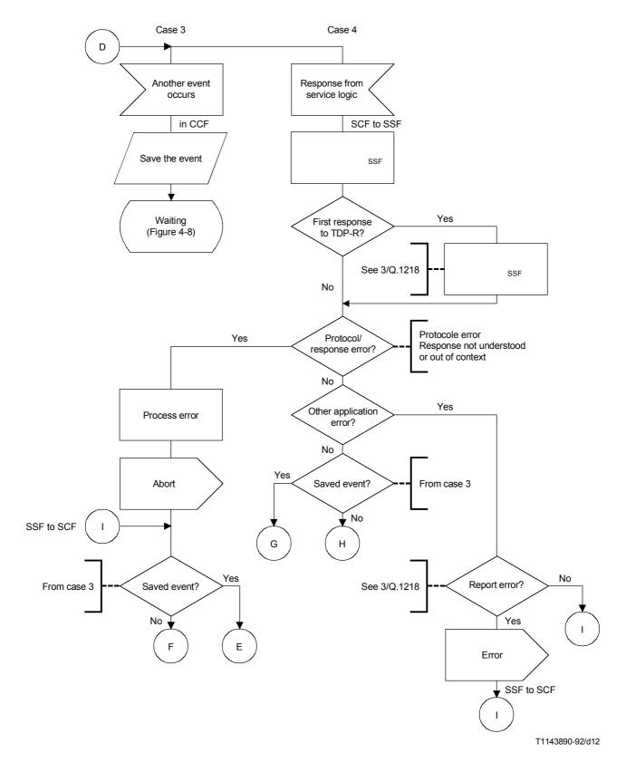
FIGURE 4-9/Q.1214 **Detection point processing**
