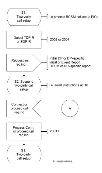
FIGURE 5-60/Q.1214 SDL diagram "basic call process" SIB (two-party call setup)
