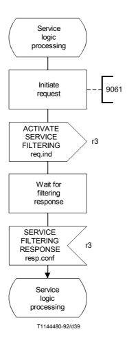
FIGURE 5-15/Q.1214 SCF actions for the "limit" SIB
