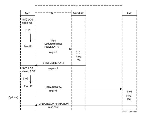
FIGURE 5-37/Q.1214 Information flow diagram "status notification" SIB
