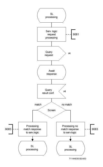
FIGURE 5-29/Q.1214 "Screen" SIB service control functional entity
