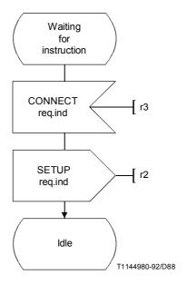
FIGURE 5-55/Q.1214 Service hand-off procedure actions at initiating CCF/SSF (FE)
