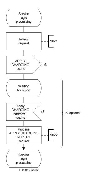
FIGURE 5-8/Q.1214 SCF actions for the "charge" SIB
