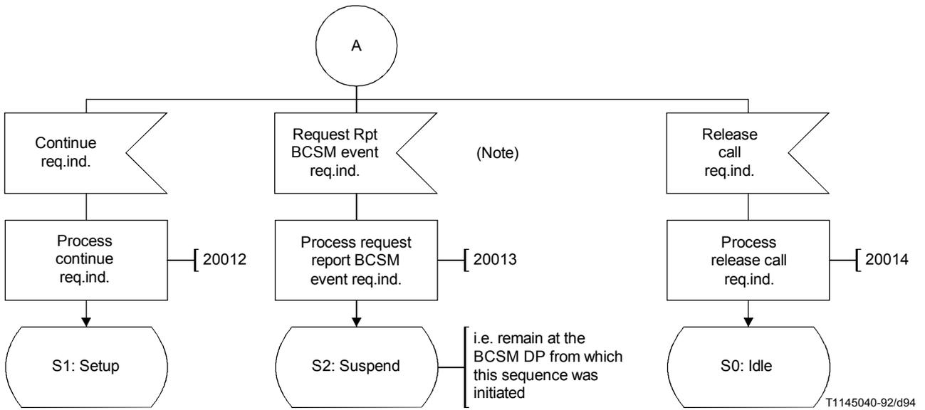
NOTE – The Request Rpt. BCSM Event req.ind should be processed before any instruction to proceed with call processing in this SDL.
