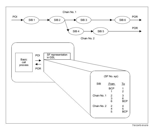
FIGURE 19/Q.1213 Global functional plane blueprint of a service feature
