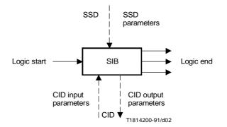
FIGURE 2/Q.1213 Graphical representation of IN CS-1 SIB
