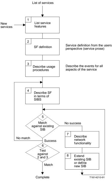
FIGURE 4 Flowchart to identify service independent building blocks
