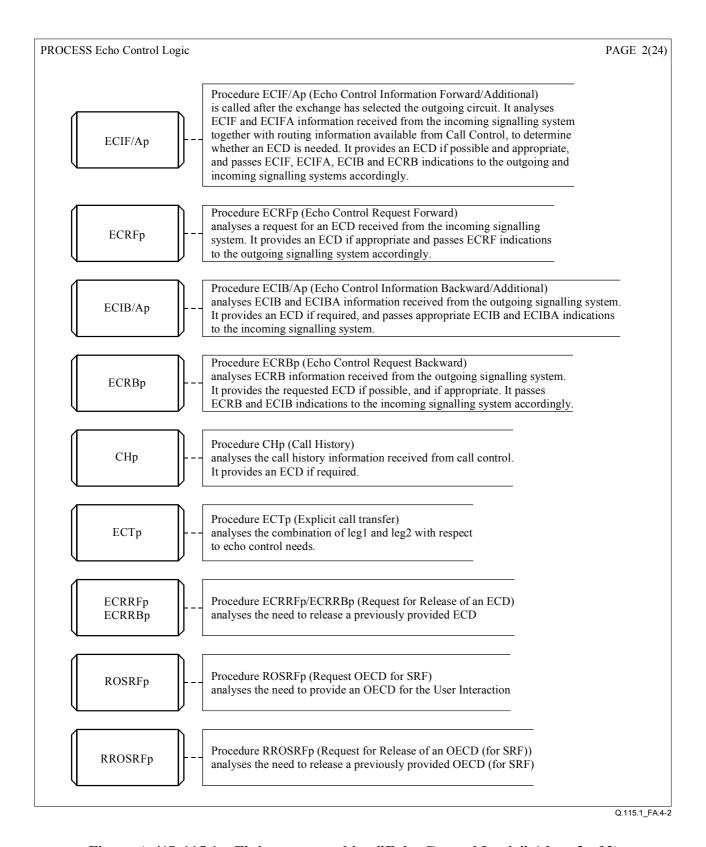
Figure A.4/Q.115.1 – Finite state machine "Echo Control Logic" (sheet 2 of 2)
