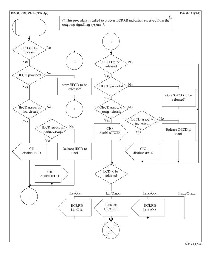
Figure A.20/Q.115.1 – Echo control procedure for the release of an ECD (backward)
