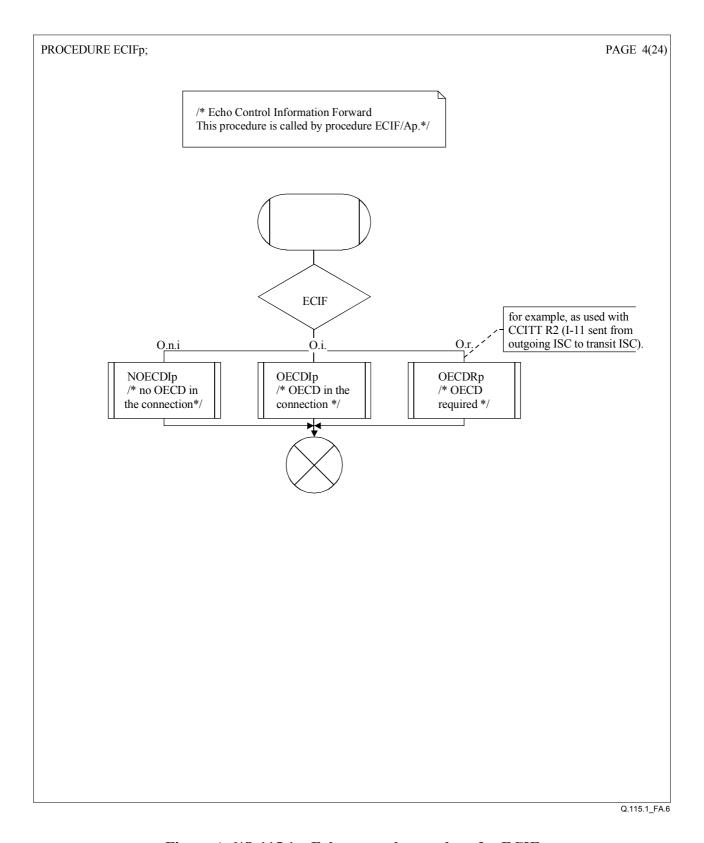
Figure A.6/Q.115.1 – Echo control procedure for ECIF
