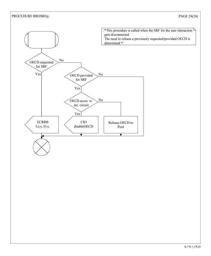
Figure A.23/Q.115.1 – Echo control procedure for the release of an OECD (IN)
