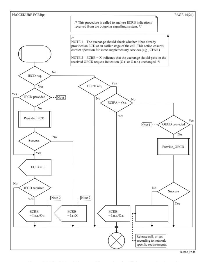
Figure A.15/Q.115.1 – Echo control procedure for ECD request (backward)
