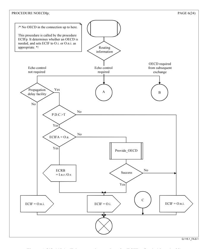
Figure A.8/Q.115.1 – Echo control procedure for ECIF = O.n.i. (sheet 1 of 2)
