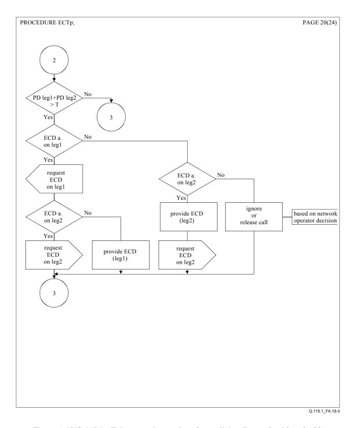
Figure A.19/Q.115.1 – Echo control procedure for explicit call transfer (sheet 3 of 3)
