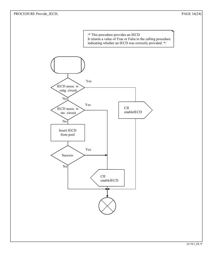
Figure A.17/Q.115.1 – Echo control procedure for providing an IECD
