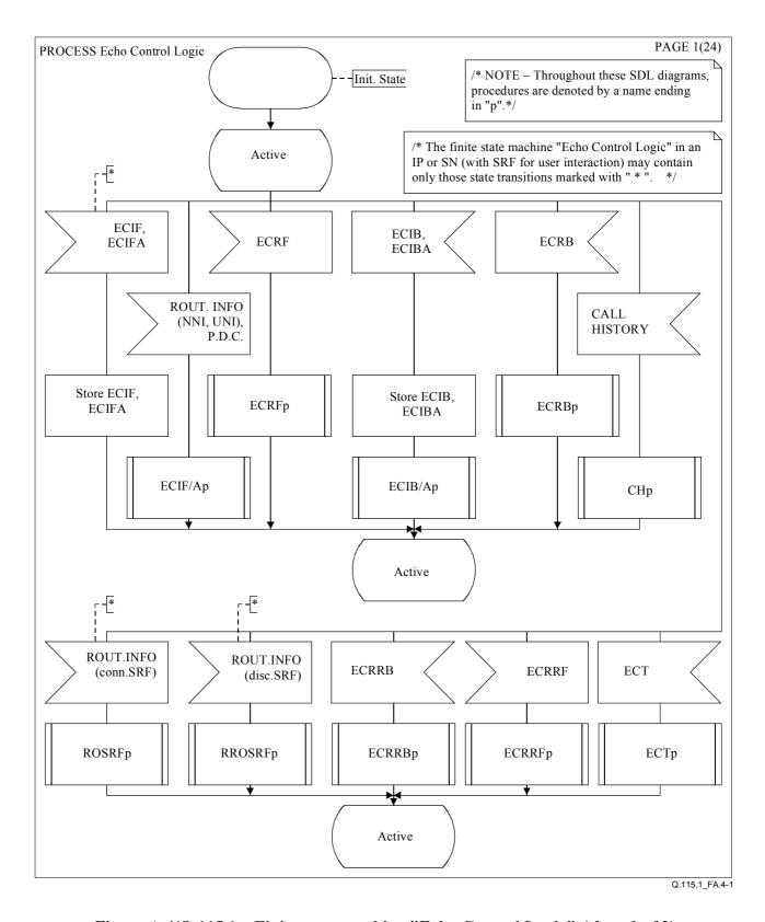
Figure A.4/Q.115.1 – Finite state machine "Echo Control Logic" (sheet 1 of 2)
