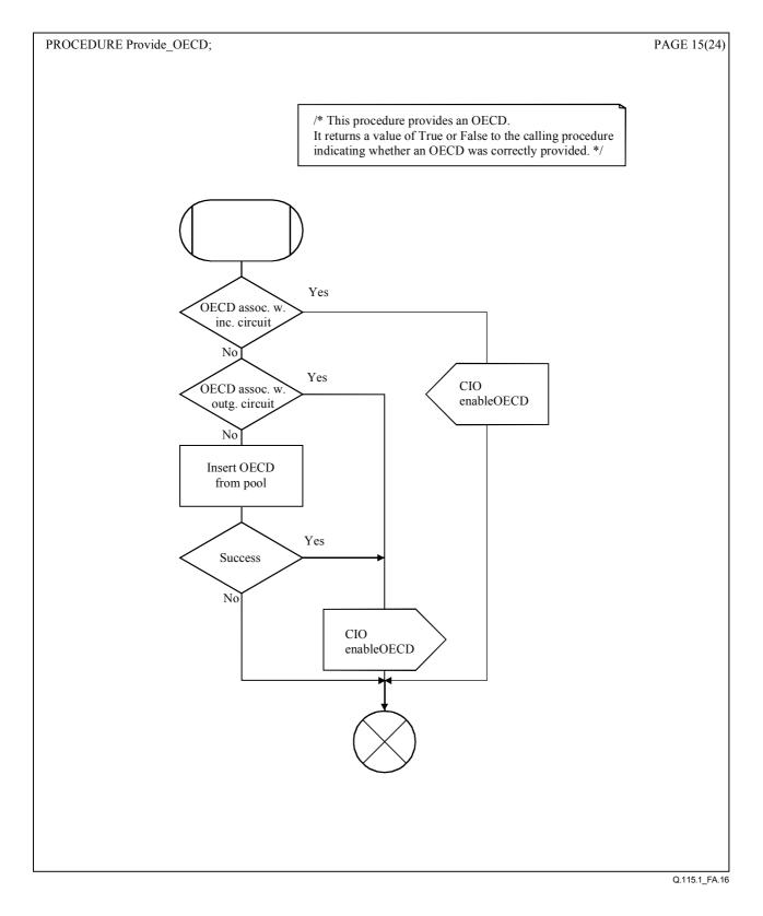
Figure A.16/Q.115.1 – Echo control procedure for providing an OECD
