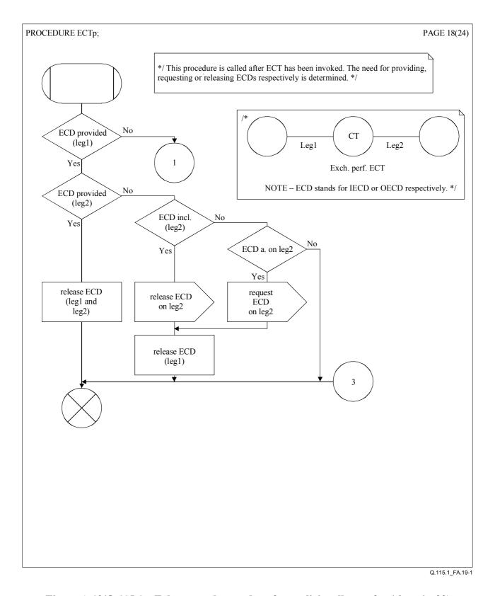
Figure A.19/Q.115.1 – Echo control procedure for explicit call transfer (sheet 1 of 3)
