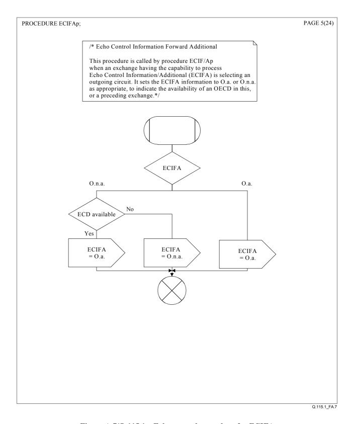
Figure A.7/Q.115.1 – Echo control procedure for ECIFA
