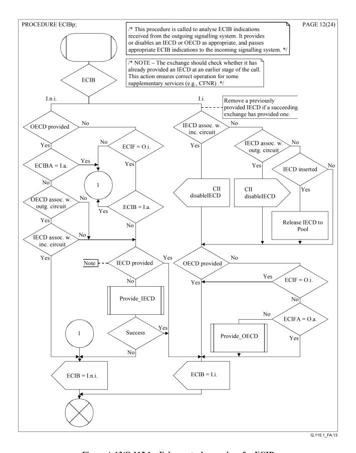
Figure A.13/Q.115.1 – Echo control procedure for ECIB
