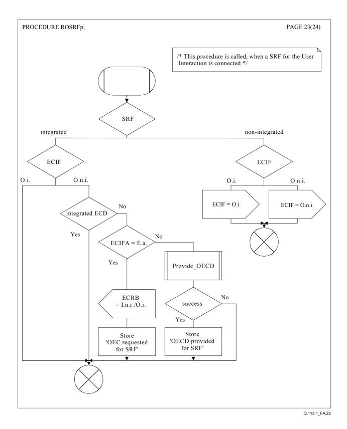
Figure A.22/Q.115.1 – Echo control procedure for the request of an OECD (IN)
