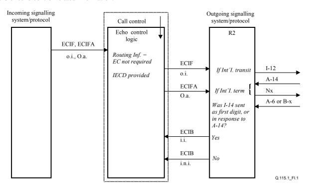
Figure I.1/Q.115.1 – Interactions between echo control logic and ITU-T signalling system R2
