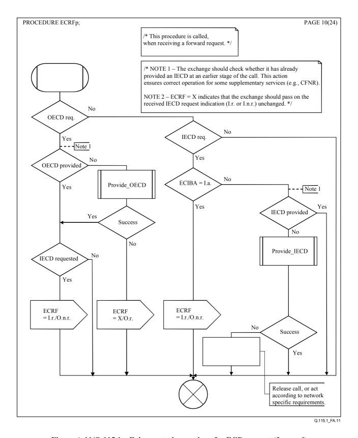
Figure A.11/Q.115.1 – Echo control procedure for ECD request (forward)
