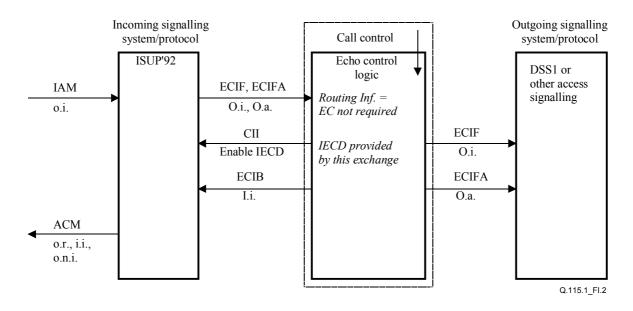
Figure I.2/Q.115.1 – Interactions between echo control logic and ISUP'92 (refer to Exchange 6 in Figure C.1/Q.764, 1993)
