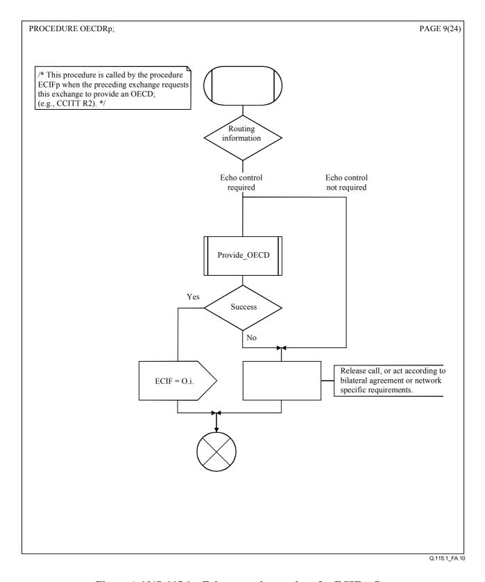
Figure A.10/Q.115.1 – Echo control procedure for ECIF = O.r.
