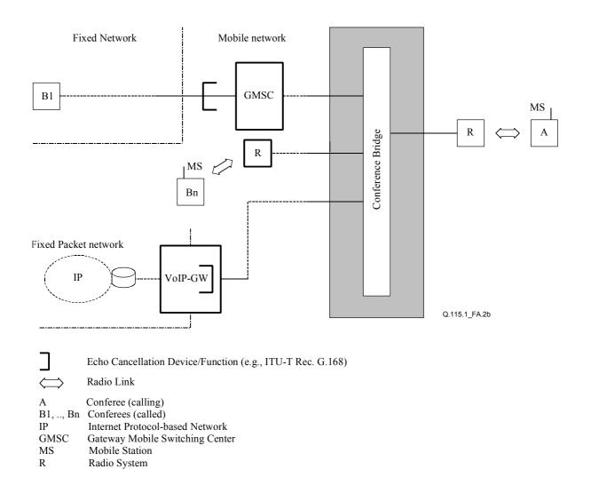
Figure A.2b/Q.115.1 – Example of a network scenario (mobile network)
