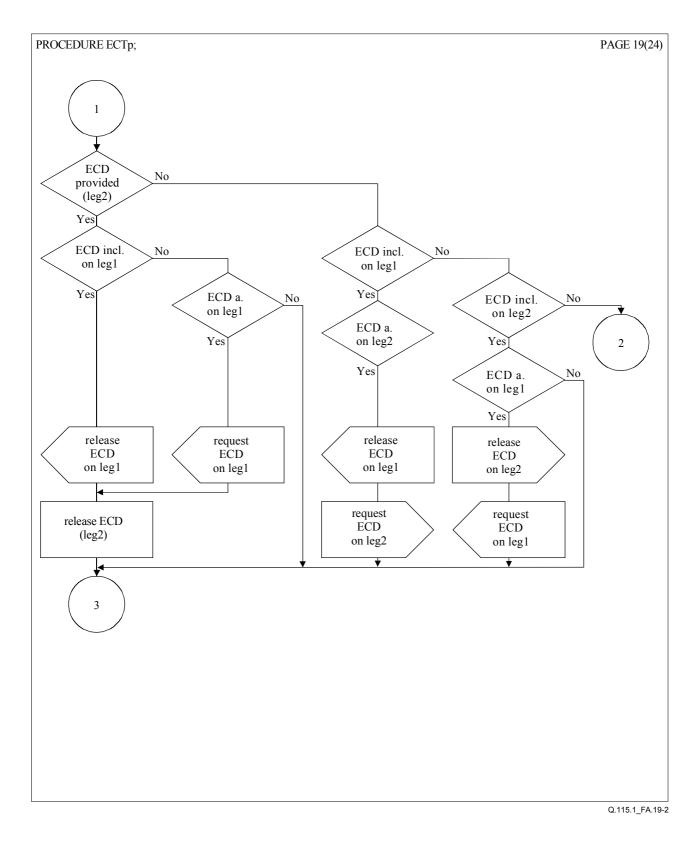
Figure A.19/Q.115.1 – Echo control procedure for explicit call transfer (sheet 2 of 3)
