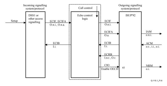
a) The CIO = enable OECD information causes ISUP'92 to provide an OECD and send a forward NRM with o.i. indication to cancel T37 in succeeding ISUP'92 exchanges that do not use the echo control logic described in this Recommendation.
