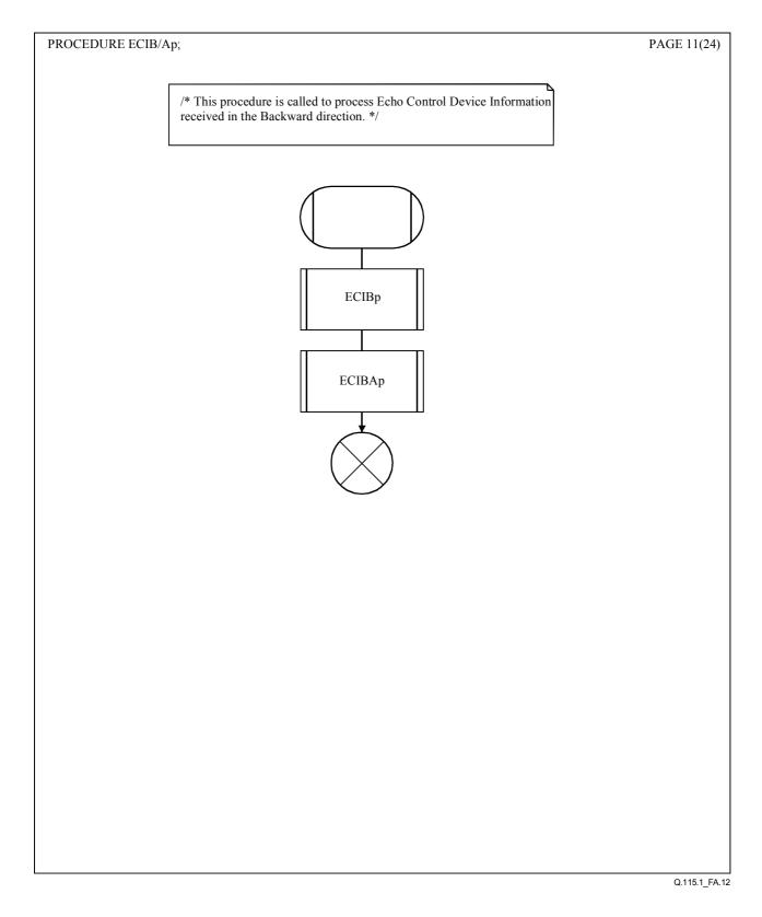
Figure A.12/Q.115.1 – Echo control procedure for ECIB/A
