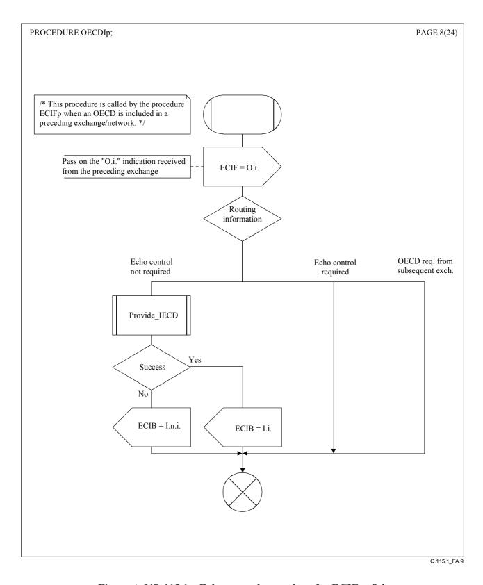
Figure A.9/Q.115.1 – Echo control procedure for ECIF = O.i.
