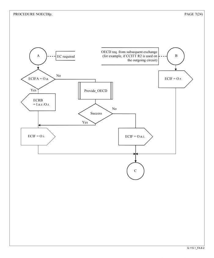
Figure A.8/Q.115.1 – Echo control procedure for ECIF = O.n.i. (sheet 2 of 2)
