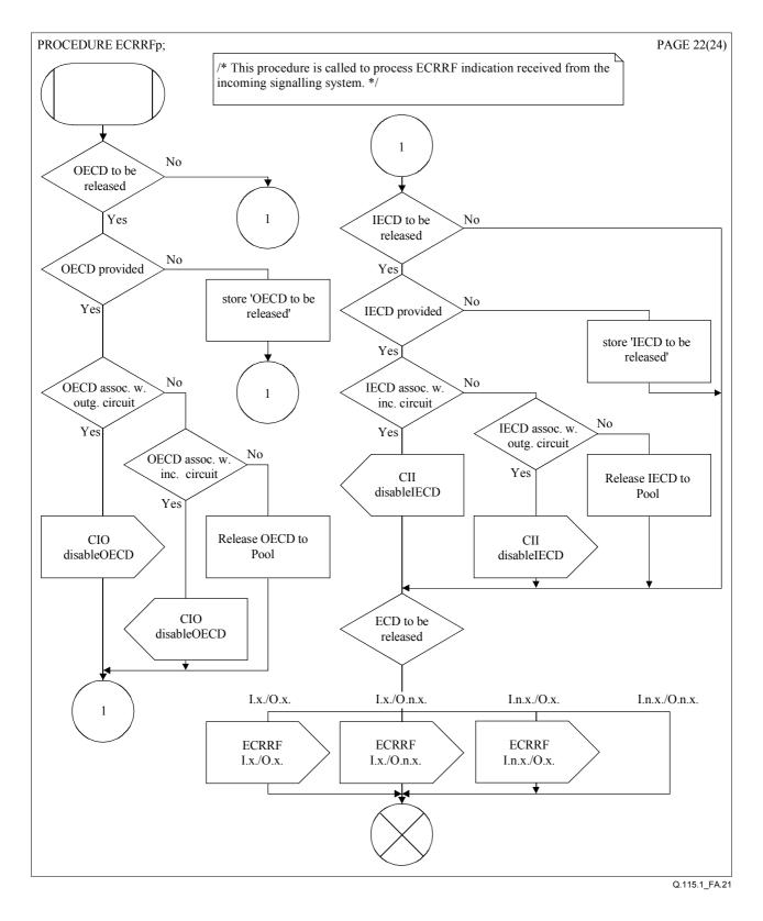
Figure A.21/Q.115.1 – Echo control procedure for the release of an ECD (forward)
