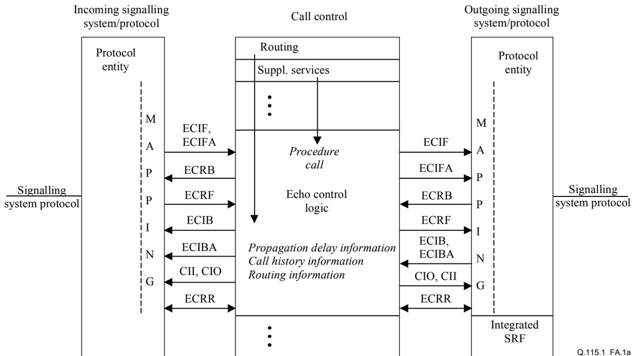
**Figure A.1a/Q.115.1 – Exchange Type 1**
