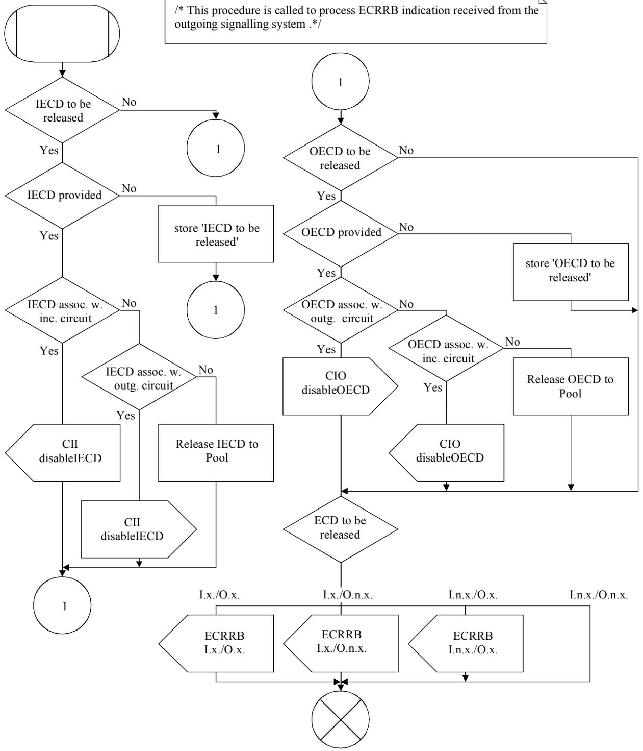
Figure A.20/Q.115.1 – Echo control procedure for the release of an ECD (backward)
