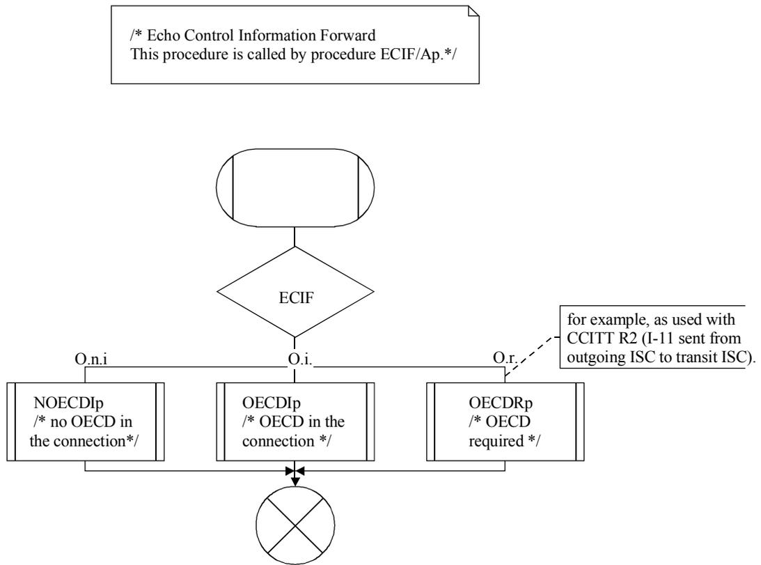
**Figure A.6/Q.115.1 – Echo control procedure for ECIF**
