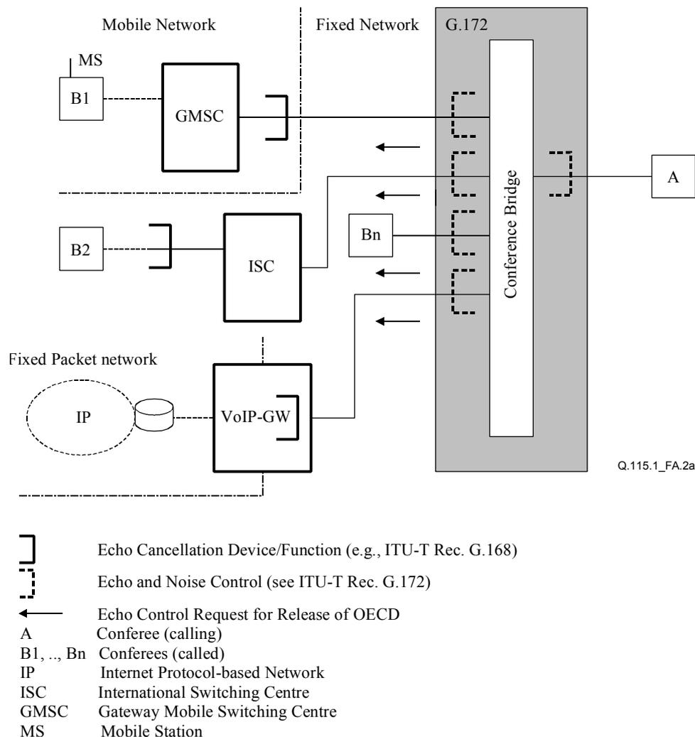
Figure A.2a/Q.115.1 – Example of a network scenario (fixed network)
