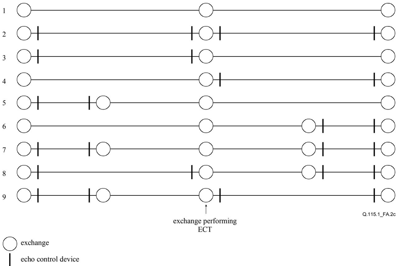
NOTE – If ECT occurs in an exchange Type 2, this may result in a non-optimal placement of ECDs or no ECDs (however required) respectively.
