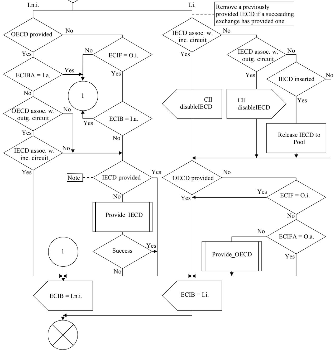
Figure A.13/Q.115.1 – Echo control procedure for ECIB
