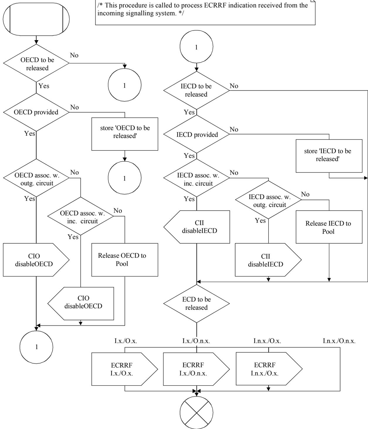
Figure A.21/Q.115.1 – Echo control procedure for the release of an ECD (forward)
