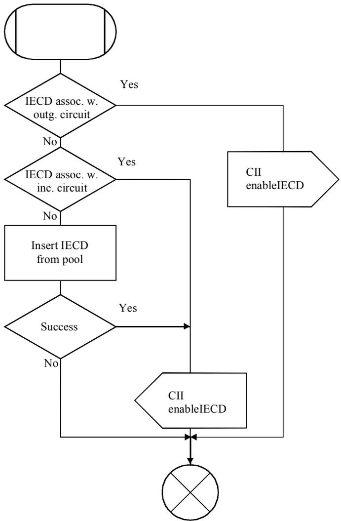
Figure A.17/Q.115.1 – Echo control procedure for providing an IECD
