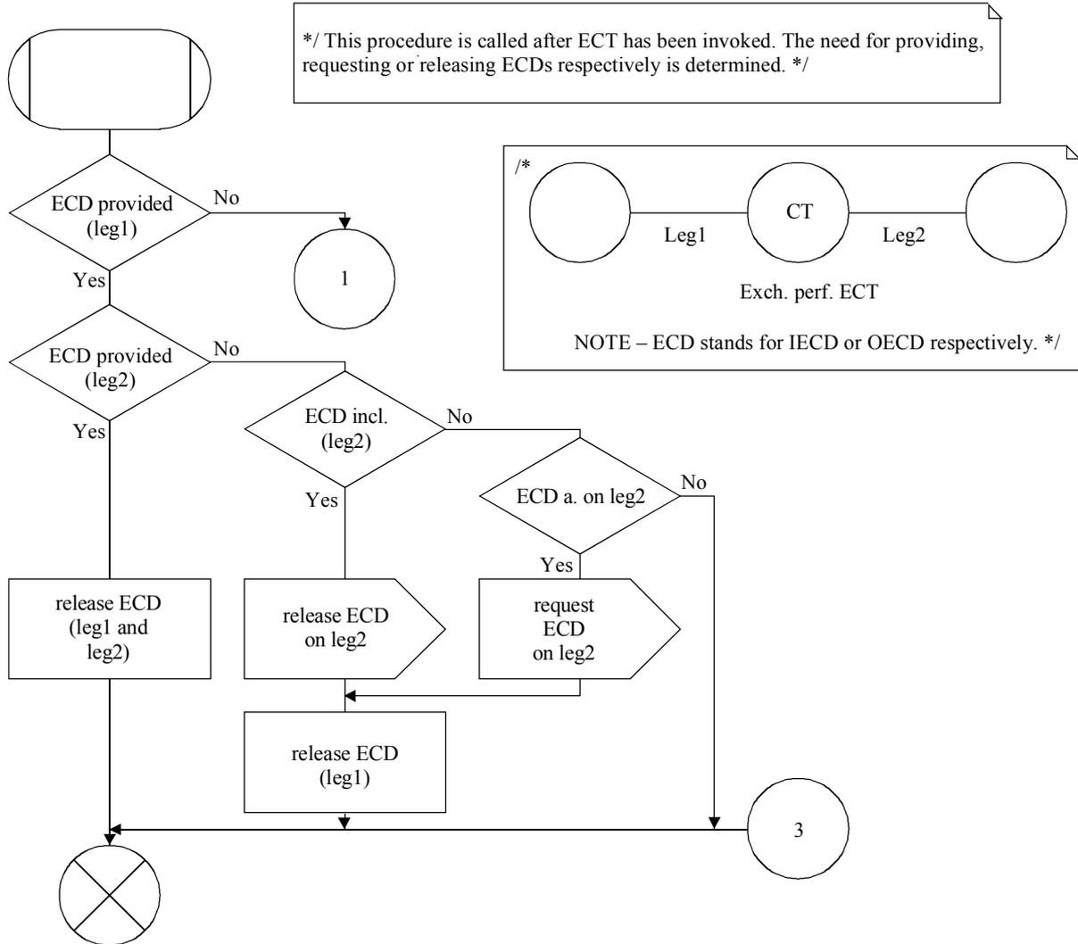
Figure A.19/Q.115.1 – Echo control procedure for explicit call transfer (sheet 1 of 3)
