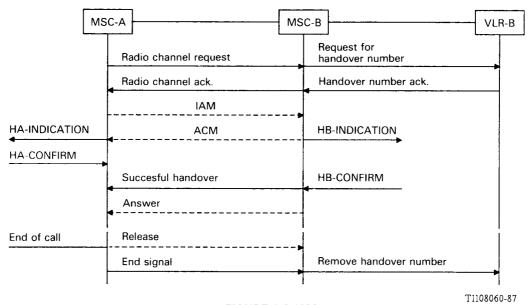
FIGURE 4/Q.1005 Basic handover procedure
