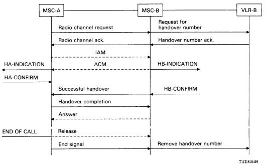
FIGURE 7/Q.1005 Basic handover procedure
