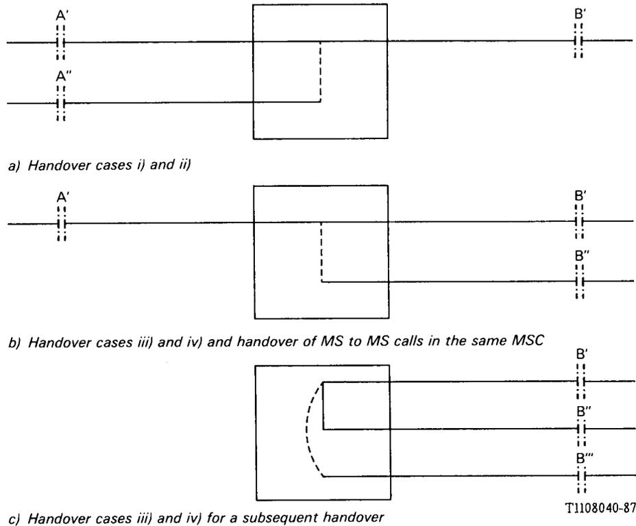
Note – In a) and b) A' is released after handover; in c) B'' is released after handover.
