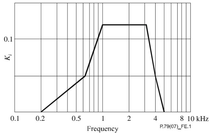
**Figure E.1 – Coefficients  $K_i$  for the  $D$ -factor**
