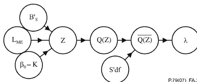
**Figure A.3 – Simplified flow diagram showing how loudness,  $\lambda$ , is related to sensation level,  $Z$**
