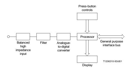
FIGURE 1/P.56 Block diagram of a typical meter
