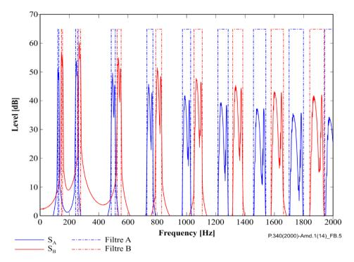
Figure B.5 – Power spectral density of input signals for Test 4 (shown only up to 2 kHz, although the signal contents span to 7 kHz range)
