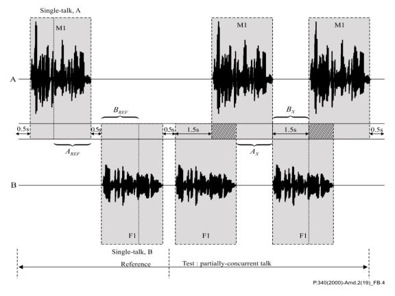
Figure B.4 – Input signal of Test 3
