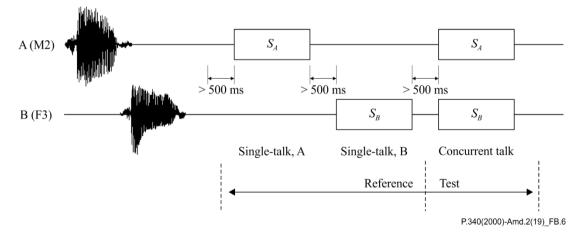
Figure B.6 – Input signal diagram of Test 4
