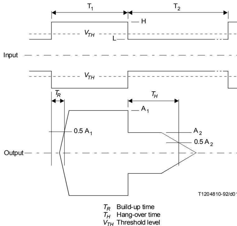
NOTE – In the case shown here, the switching time  $T_S$  is larger than  $T_R + T_H$ .
