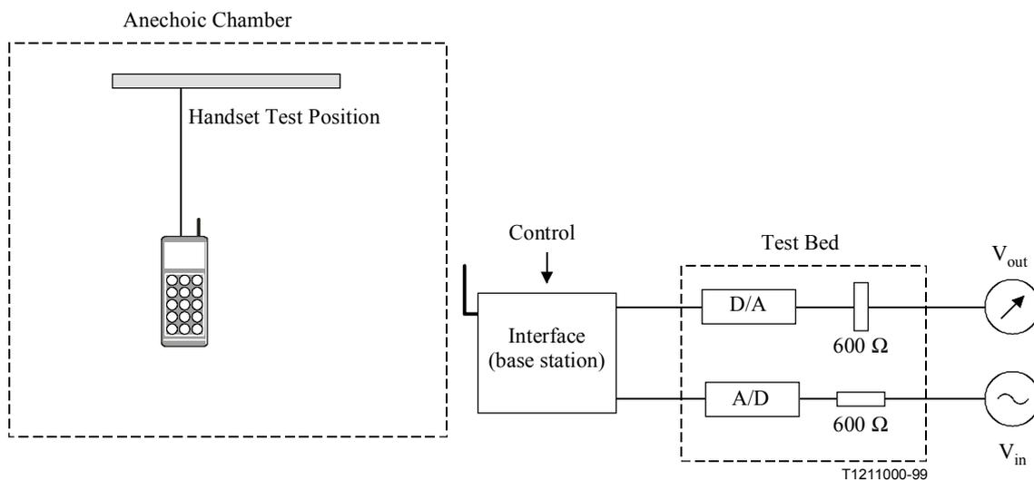
**Figure 7/P.313 – Terminal coupling loss measurement method**
