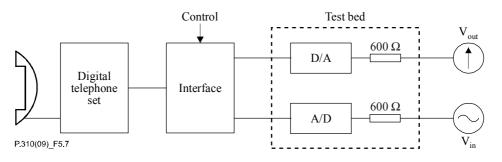
Figure 5-7 – Measurement of terminal coupling loss, HATS position
