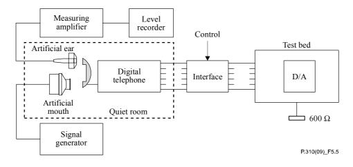
Figure 5-5 – Measurement of talker sidetone sensitivity/frequency characteristic, HATS position
