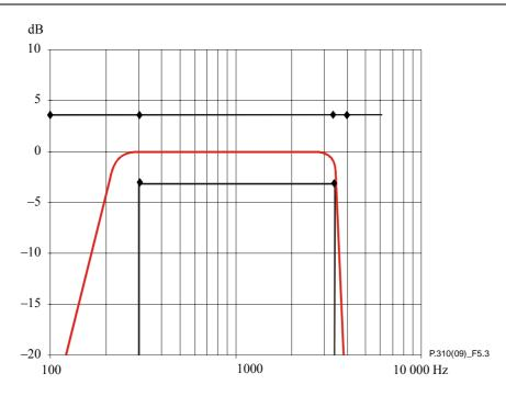
Figure 5-3 – Receiving mask with HATS, diffuse-field equalized
