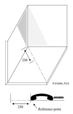
Figure 5-8 – Reference corner and reference position
