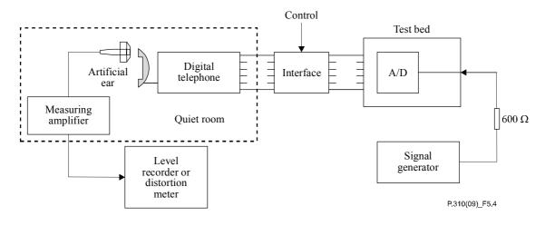
Figure 5-4 – Measurement of receiving frequency characteristic, HATS position
