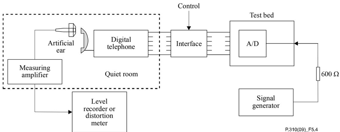
**Figure 5-4 – Measurement of receiving frequency characteristic, HATS position**
