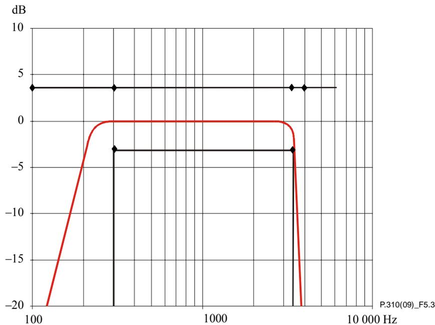
**Figure 5-3 – Receiving mask with HATS, diffuse-field equalized**
