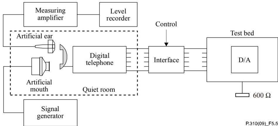
**Figure 5-5 – Measurement of talker sidetone sensitivity/frequency characteristic, HATS position**
