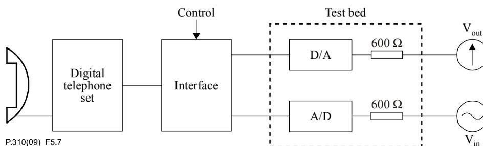
**Figure 5-7 – Measurement of terminal coupling loss, HATS position**
