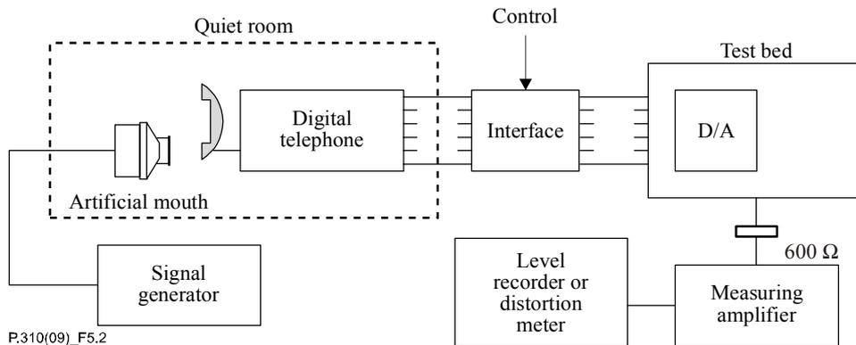
**Figure 5-2 – Measurements of sending frequency characteristic, HATS position**
