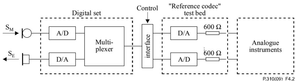
**Figure 4-2 – Digital telephone test arrangement (codec approach)**
