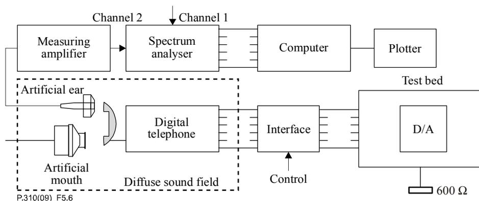
**Figure 5-6 – Measurement of listener sidetone sensitivity/frequency characteristic, HATS position**
