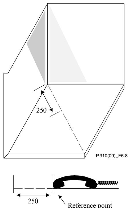
Figure 5-8 – Reference corner and reference position
