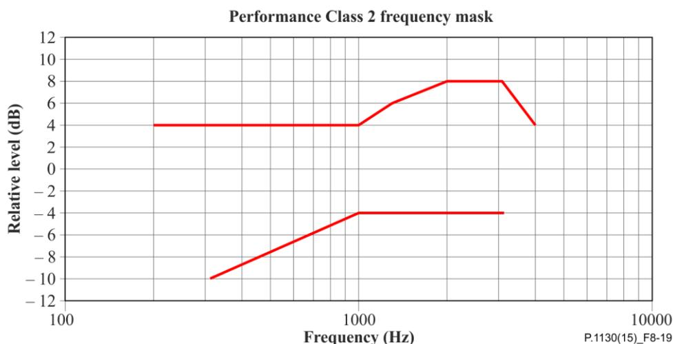
**Figure 8-19 – Signal enhancement frequency response mask (Figure is informative)**
