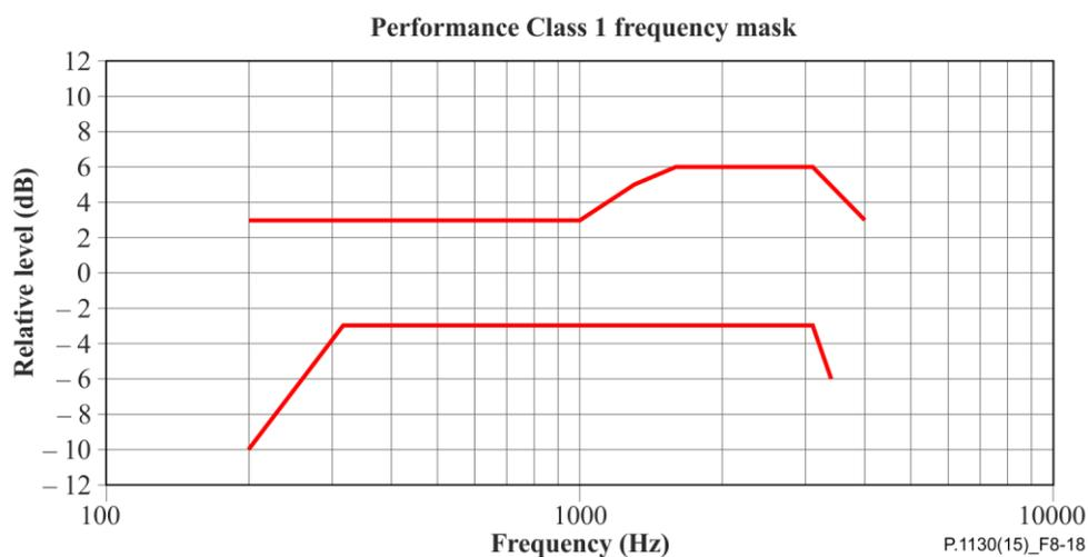
**Figure 8-18 – Signal enhancement frequency response mask (Figure is informative)**
