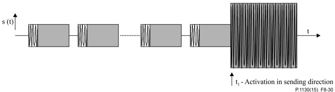
**Figure 8-30 – Structure of the test signal for measuring the attenuation range**
