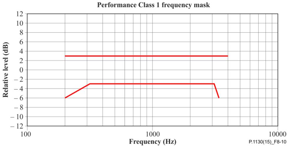
**Figure 8-10 – Audio subsystem frequency response mask (Figure is informative)**
