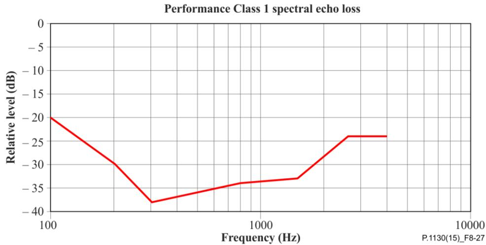
**Figure 8-27 – Spectral echo loss mask Performance Class 1 (Figure is informative)**
