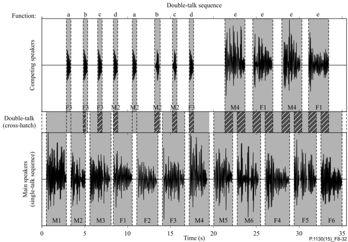
**Figure 8-32 – Double-talk test sequence with overlapping CS-signals in send and receive direction**
