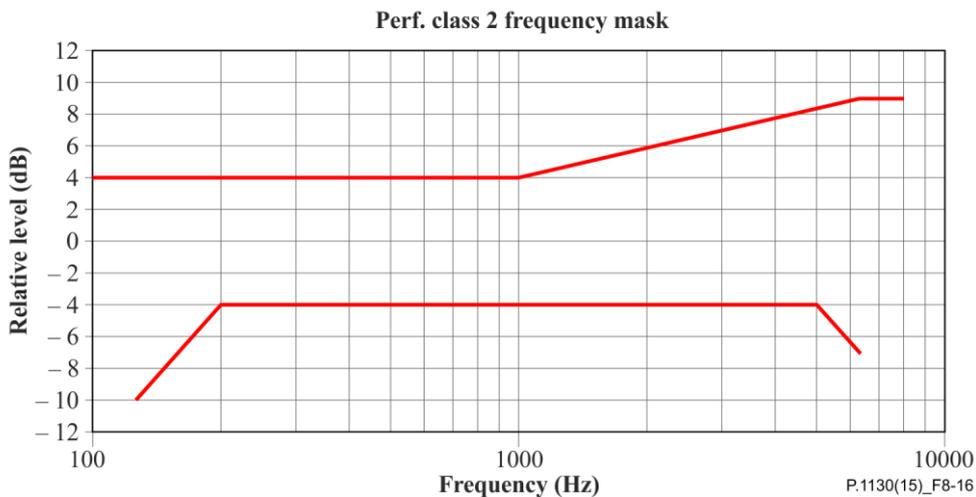
Figure 8-16 – Signal enhancement frequency response mask (Figure is informative)
