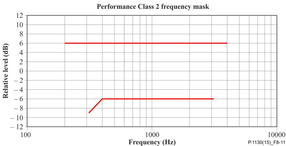
**Figure 8-11 – Audio subsystem frequency response mask (Figure is informative)**
