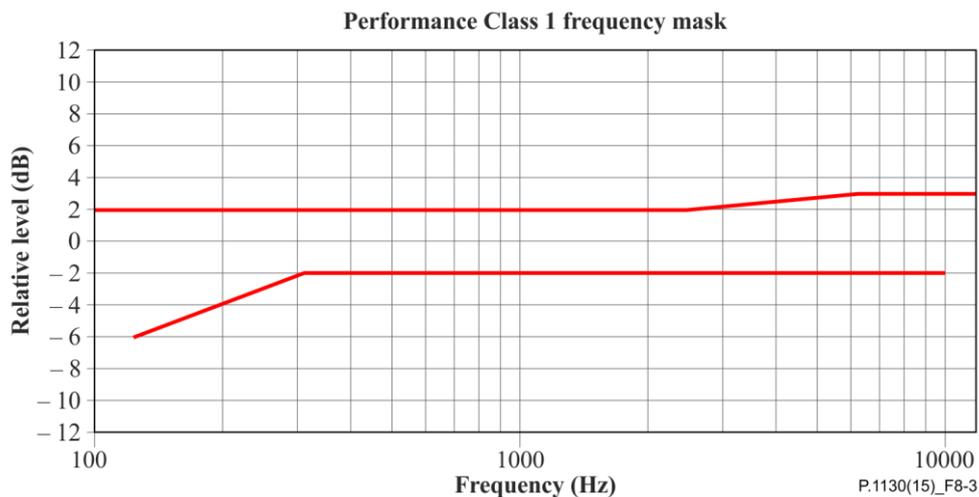
**Figure 8-3 – Microphone frequency response mask (Figure is informative)**
