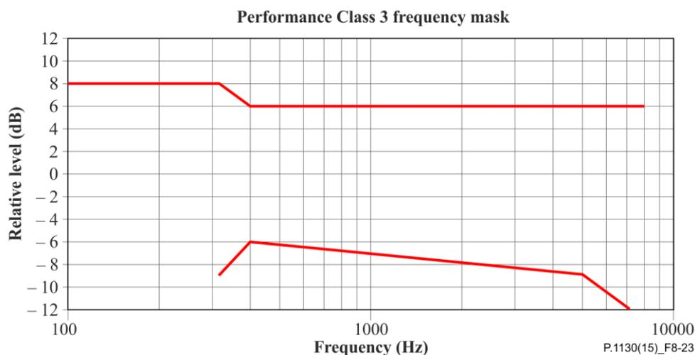
**Figure 8-23 – Signal enhancement frequency response mask (Figure is informative)**
