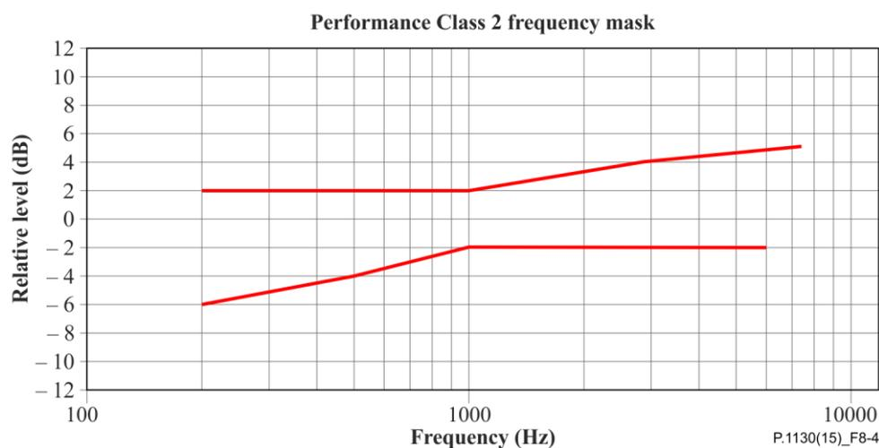
**Figure 8-4 – Microphone frequency response mask (Figure is informative)**
