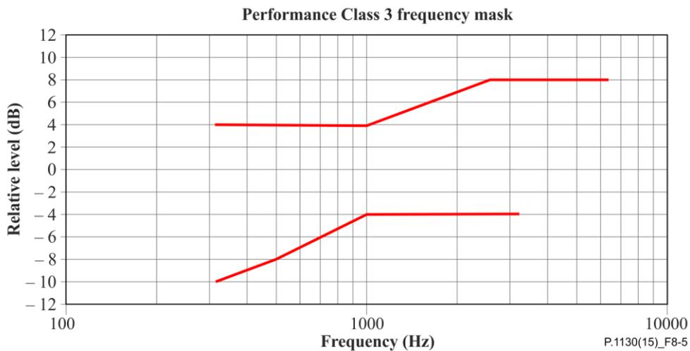
**Figure 8-5 – Microphone frequency response mask (Figure is informative)**
