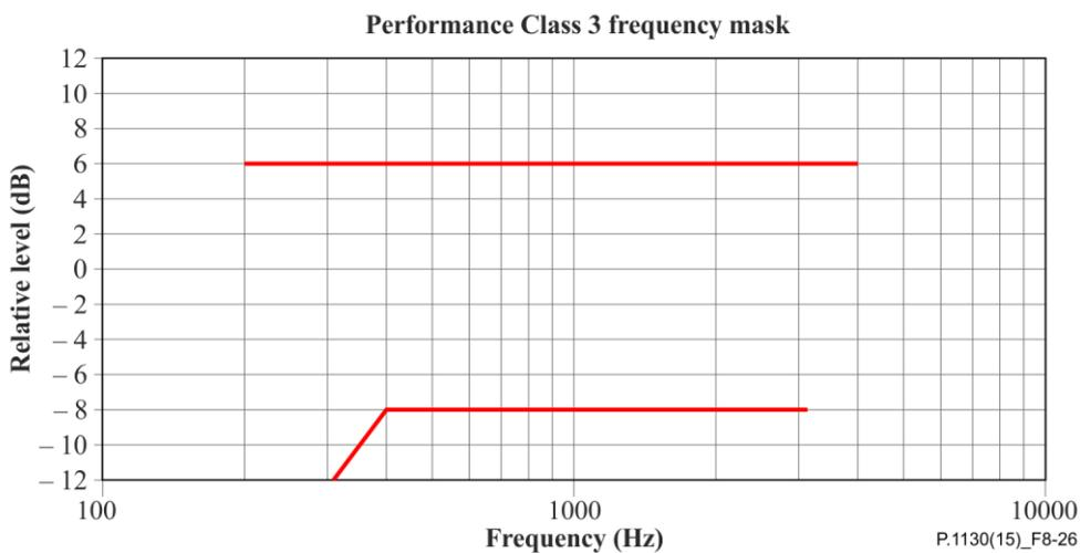
Figure 8-26 – Signal enhancement frequency response mask (Figure is informative)
