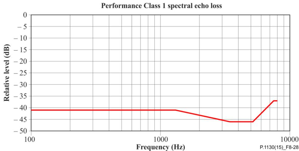
**Figure 8-28 – Spectral echo loss mask Performance Class 1 (Figure is informative)**
