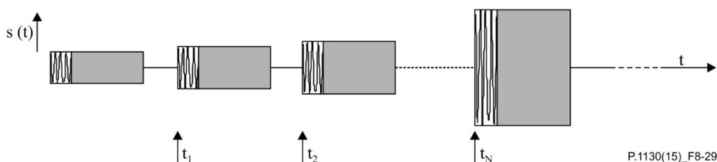
**Figure 8-29 – Test signal to determine the minimum activation level and the built-up time**
