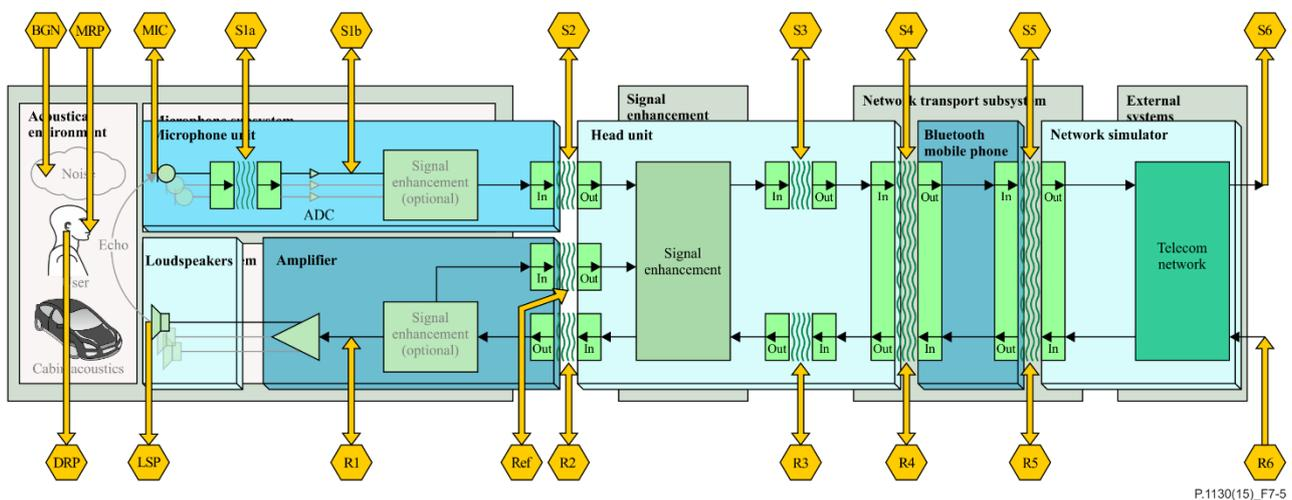
**Figure 7-5 – System overview and test points; example of a typical implementation**
