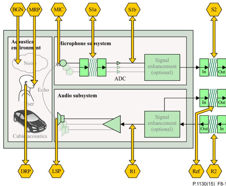
**Figure 8-1 – Acoustic subsystem and test points**
