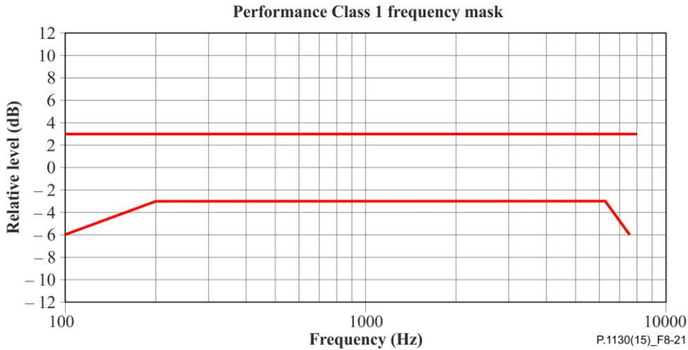
**Figure 8-21 – Signal enhancement frequency response mask (Figure is informative)**
