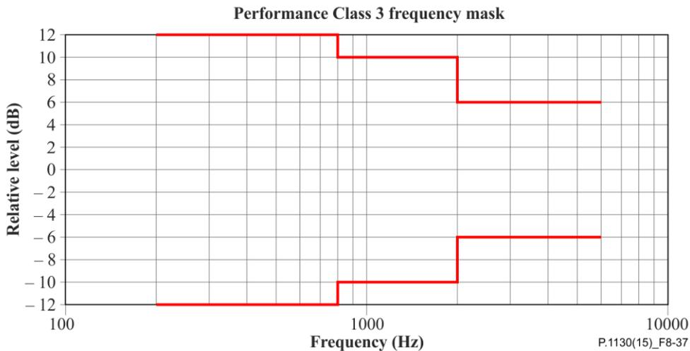
**Figure 8-37 – Spectral limits for the comfort noise injection after enhancement for Performance Class 3 (Figure is informative)**
