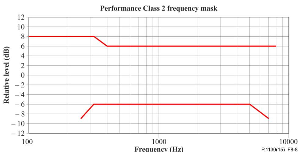
**Figure 8-8 – Audio subsystem frequency response mask (Figure is informative)**
