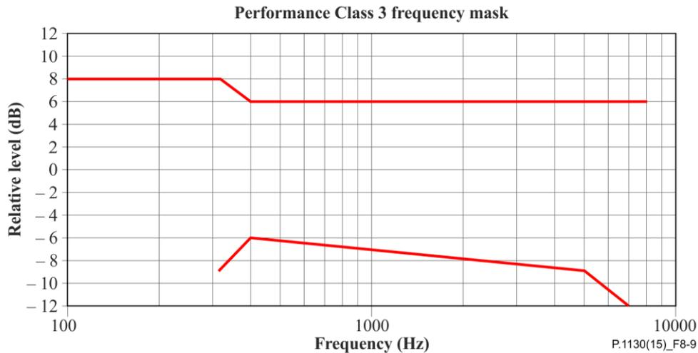
**Figure 8-9 – Audio subsystem frequency response mask (Figure is informative)**
