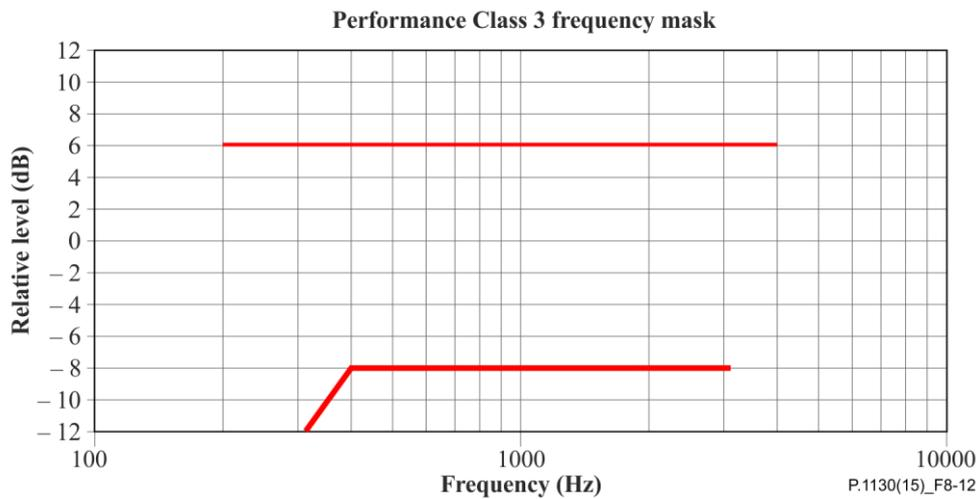
**Figure 8-12 – Audio subsystem frequency response mask (Figure is informative)**
