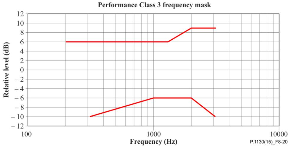
**Figure 8-20 – Signal enhancement frequency response mask (Figure is informative)**
