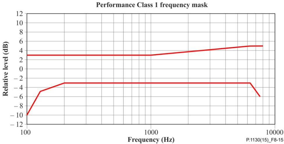
Figure 8-15 – Signal enhancement frequency response mask (Figure is informative)
