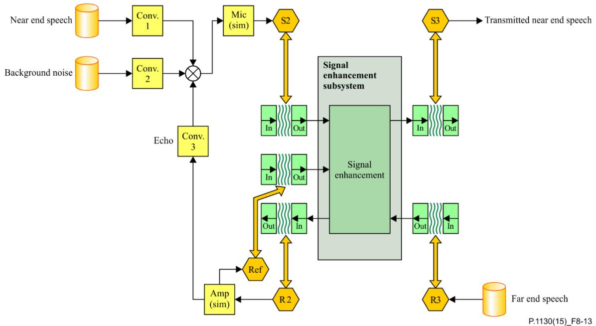
**Figure 8-13 – Signal enhancement subsystem with simulation paths**
