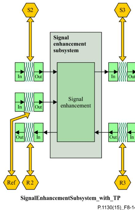
**Figure 8-14 – Signal enhancement subsystem and test points**
