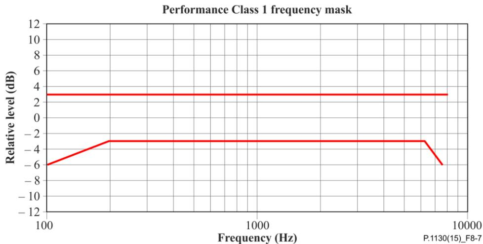
**Figure 8-7 – Audio subsystem frequency response mask (Figure is informative)**
