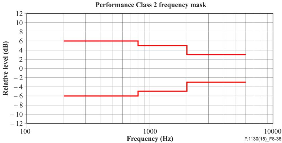
**Figure 8-36 – Spectral limits for the comfort noise injection after enhancement for Performance Class 2 (Figure is informative)**
