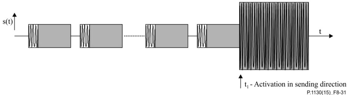
**Figure 8-31 – Structure of the test signal for measuring the attenuation range**
