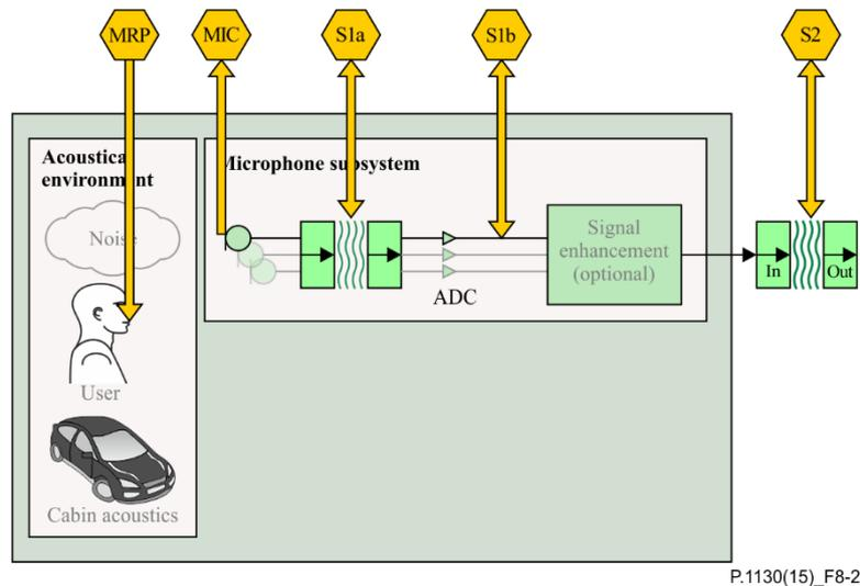
**Figure 8-2 – Microphone subsystem and test points**
