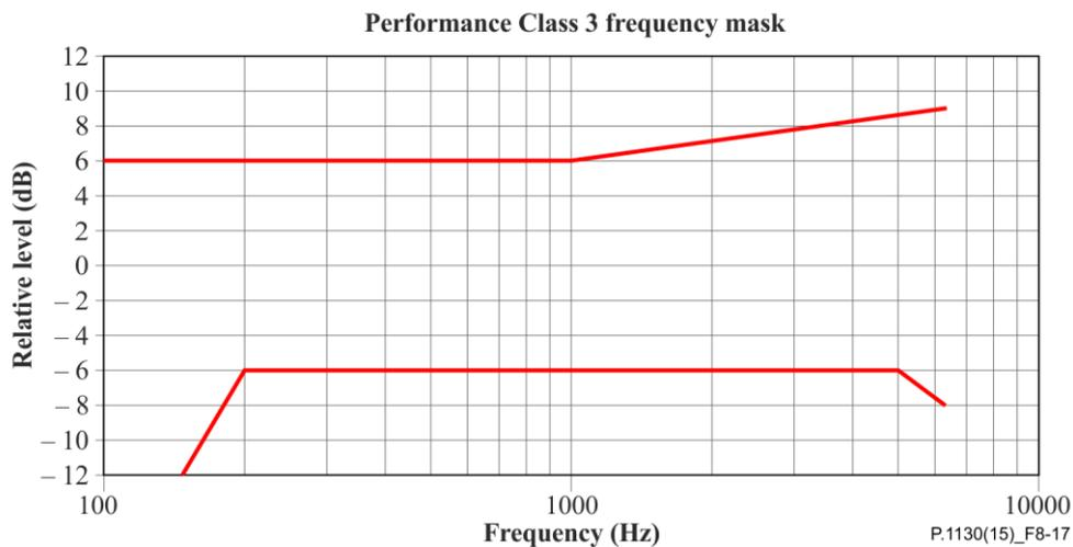
**Figure 8-17 – Signal enhancement frequency response mask (Figure is informative)**
