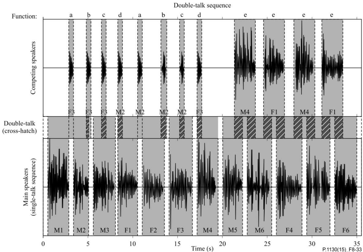
**Figure 8-33 – Double-talk test sequence with overlapping CS-signals in receive and send direction**
