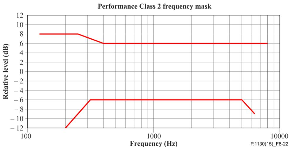
**Figure 8-22 – Signal enhancement frequency response mask (Figure is informative)**
