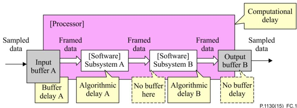
**Figure C.1 – Framing and delays**
