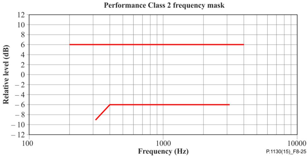
Figure 8-25 – Signal enhancement frequency response mask (Figure is informative)
