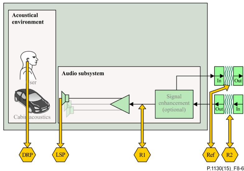
**Figure 8-6 – Audio subsystem and test points**
