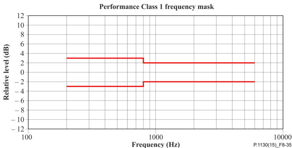
**Figure 8-35 – Spectral limits for the comfort noise injection after enhancement for Performance Class 1 (Figure is informative)**
