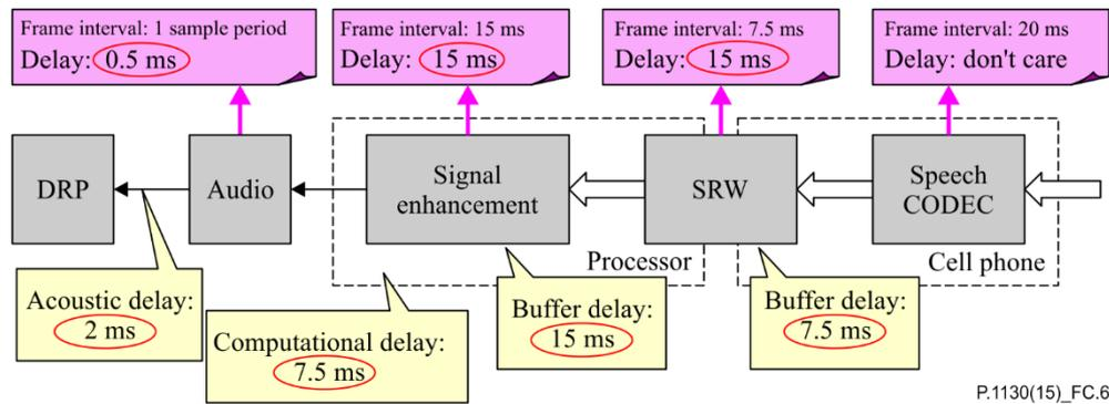
**Figure C.6 – An example of automotive hands-free receive system**
