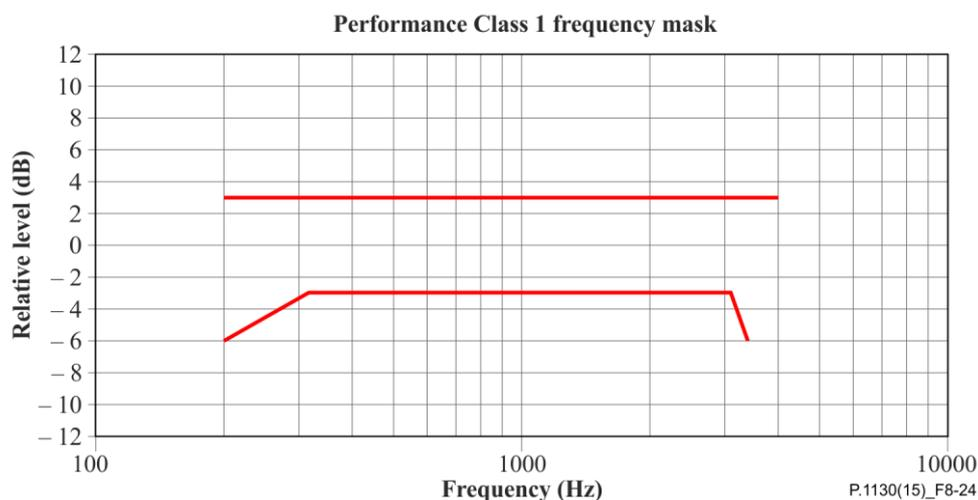
**Figure 8-24 – Signal enhancement frequency response mask (Figure is informative)**
