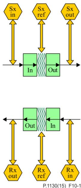
**Figure 10-1 – Unidirectional transport subsystem**
