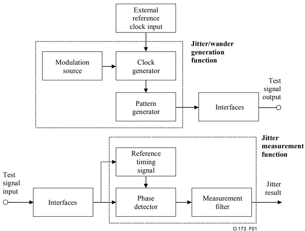
**Figure 1/O.173 – Functional block diagram for jitter test set**
