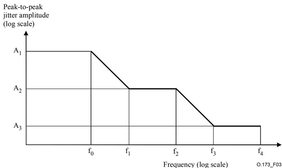
**Figure 3/O.173 – Measured jitter amplitude versus jitter frequency**
