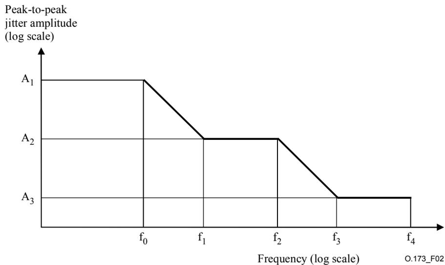
**Figure 2/O.173 – Generated jitter amplitude versus jitter frequency**
