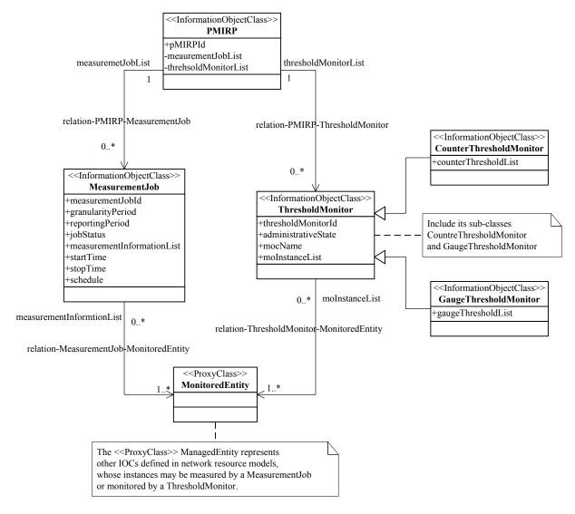
Figure 7-4 – Performance measurement information object classes
