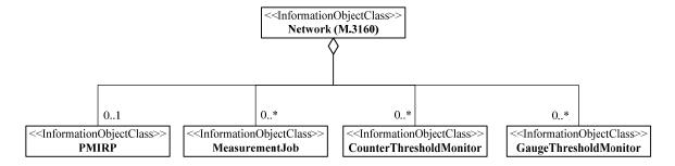
Figure 7-3 – Containment diagram of performance management IOCs
