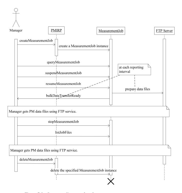
Figure 7-9 – Sequence diagram of performance measurement management
