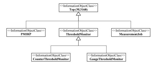
Figure 7-5 – Performance measurement IOCs inheritance
