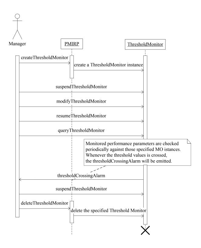
Figure 7-10 – Sequence diagram of performance threshold management
