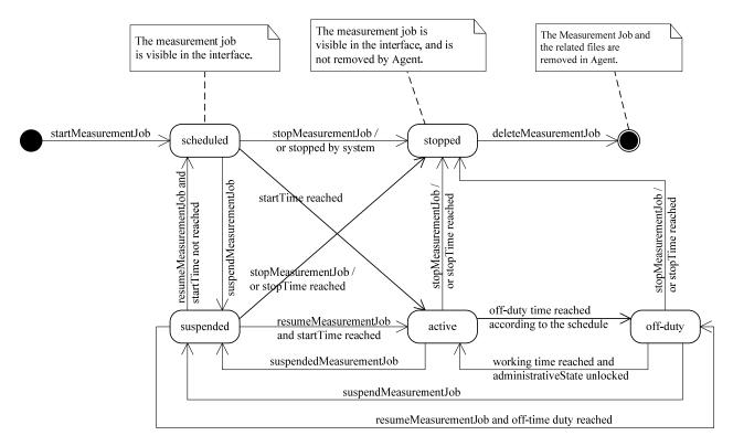
Figure 7-6 – MeasurementJob state diagram
