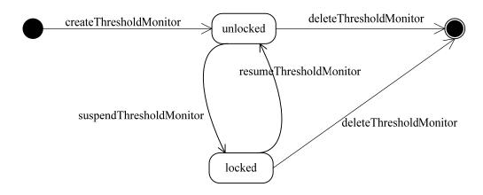
Figure 7-7 – ThresholdMonitor state diagram
