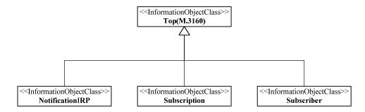
Figure 6 – Inheritance diagram for IOCs in notification management
