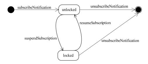
Figure 7 – State diagram of notification subscription
