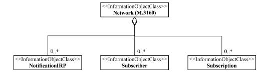
Figure 4 - Containment diagram of notification management IOCs
