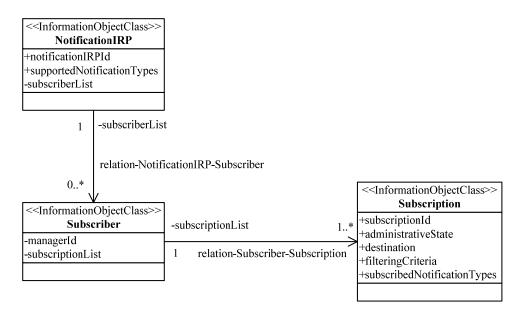
Figure 5 - Class diagram of notification management IOCs
