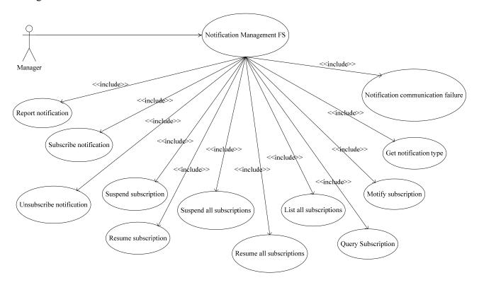
Figure 1 – High-level use case diagram of the notification management interface
