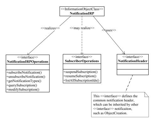
Figure 8 – Class diagram for the notification interface
