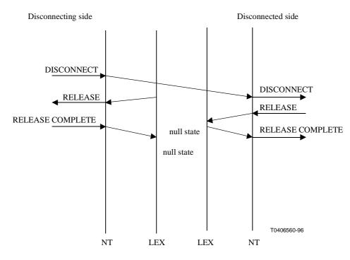
Figure 8/M.3650 – Disengagement delays
