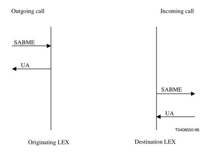
Figure 7/M.3650 – Layer 2 activation delay
