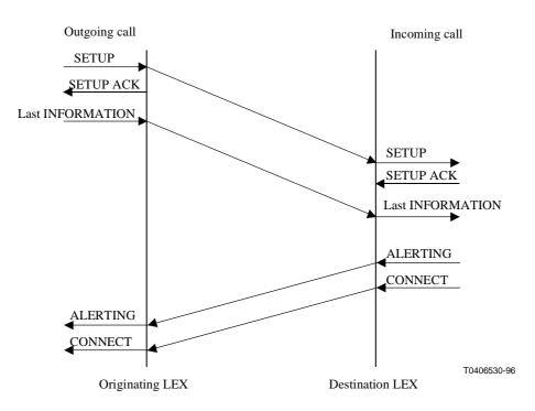
Figure 5/M.3650 – Alerting delays for overlap sending and receiving
