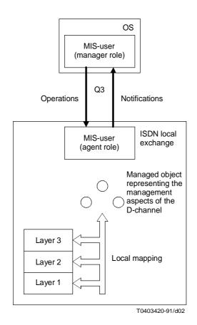
$FIGURE\ 2/M.3640$  Reference configuration for management of the access protocol
