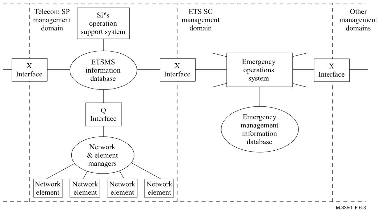
**Figure 6-3/M.3350 – Architecture of ETSMS across the X-interface**
