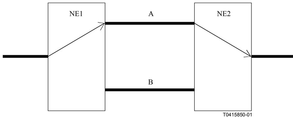
Figure 10/M.3100 – Unidirectional cross-connection
