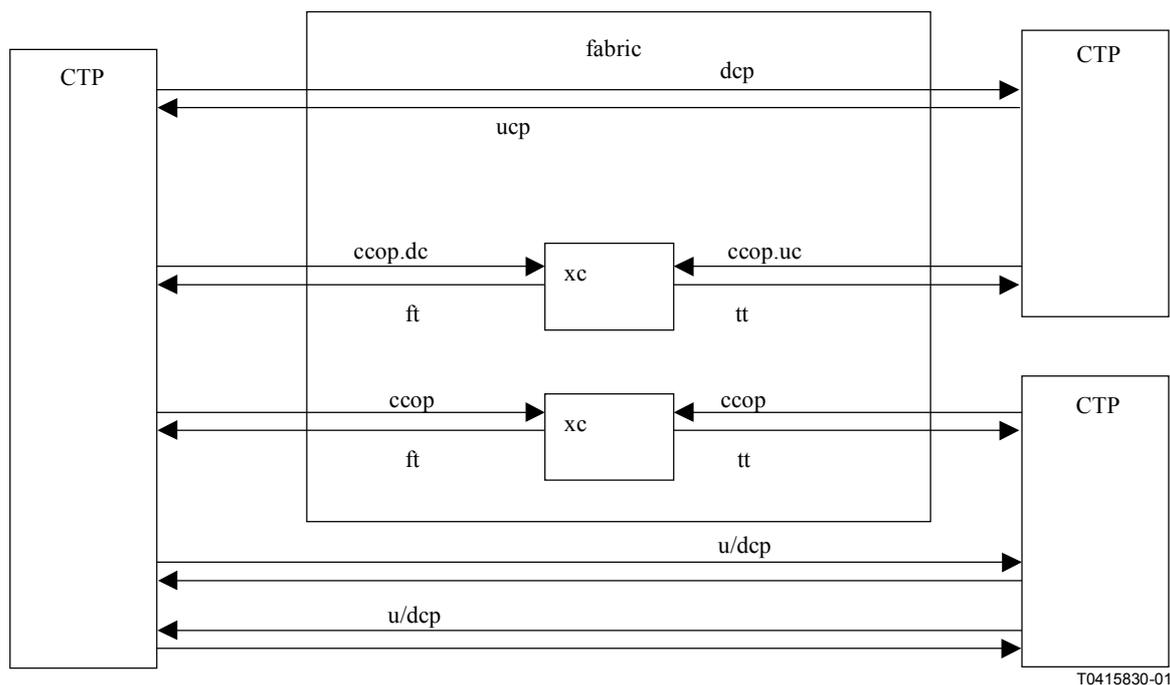
**Figure 8/M.3100 – Roll operation (point-to-point bidirectional)**
