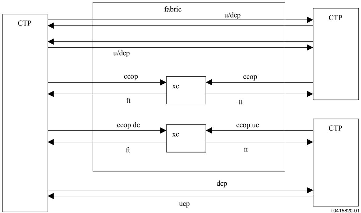
**Figure 7/M.3100 – Bridge operation (point-to-point bidirectional)**
