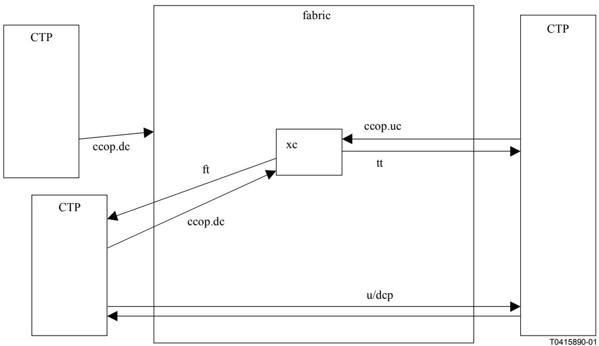
**Figure 14/M.3100 – Release operation (point-to-point unidirectional sink end)**
