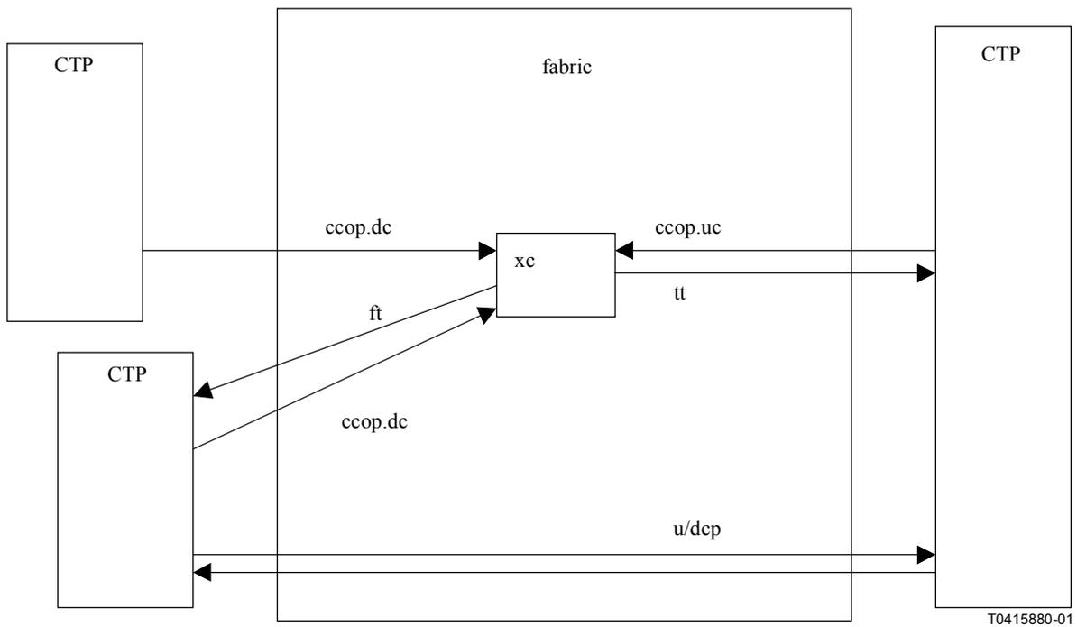
**Figure 13/M.3100 – Roll operation (point-to-point unidirectional sink end)**
