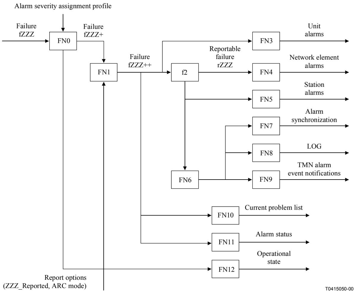
**Figure 7/M.3100 – Alarm flow functional model**
