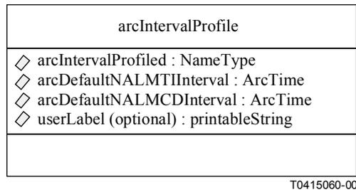
**Figure 8/M.3100 – Alarm reporting control interval profile object class**
