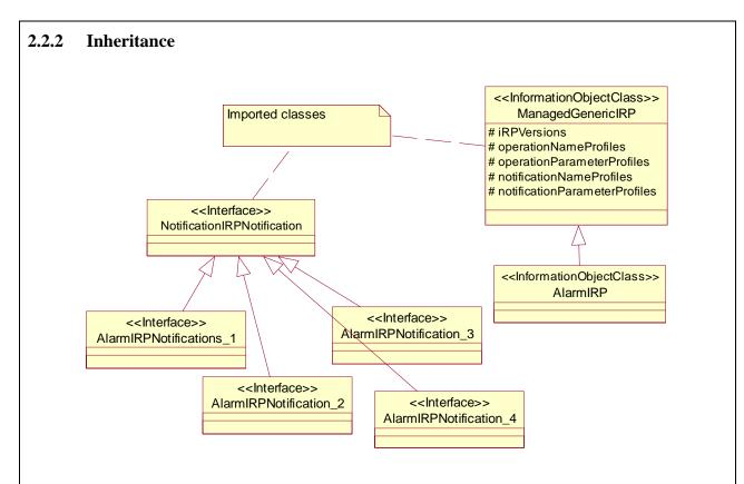
Figure II.2 – Alarm management IOC inheritance
