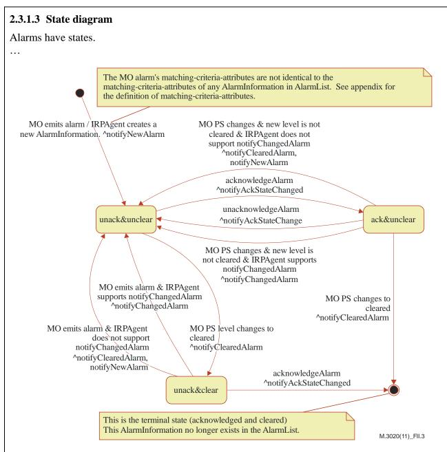
Figure II.3 – Alarm information state diagram
