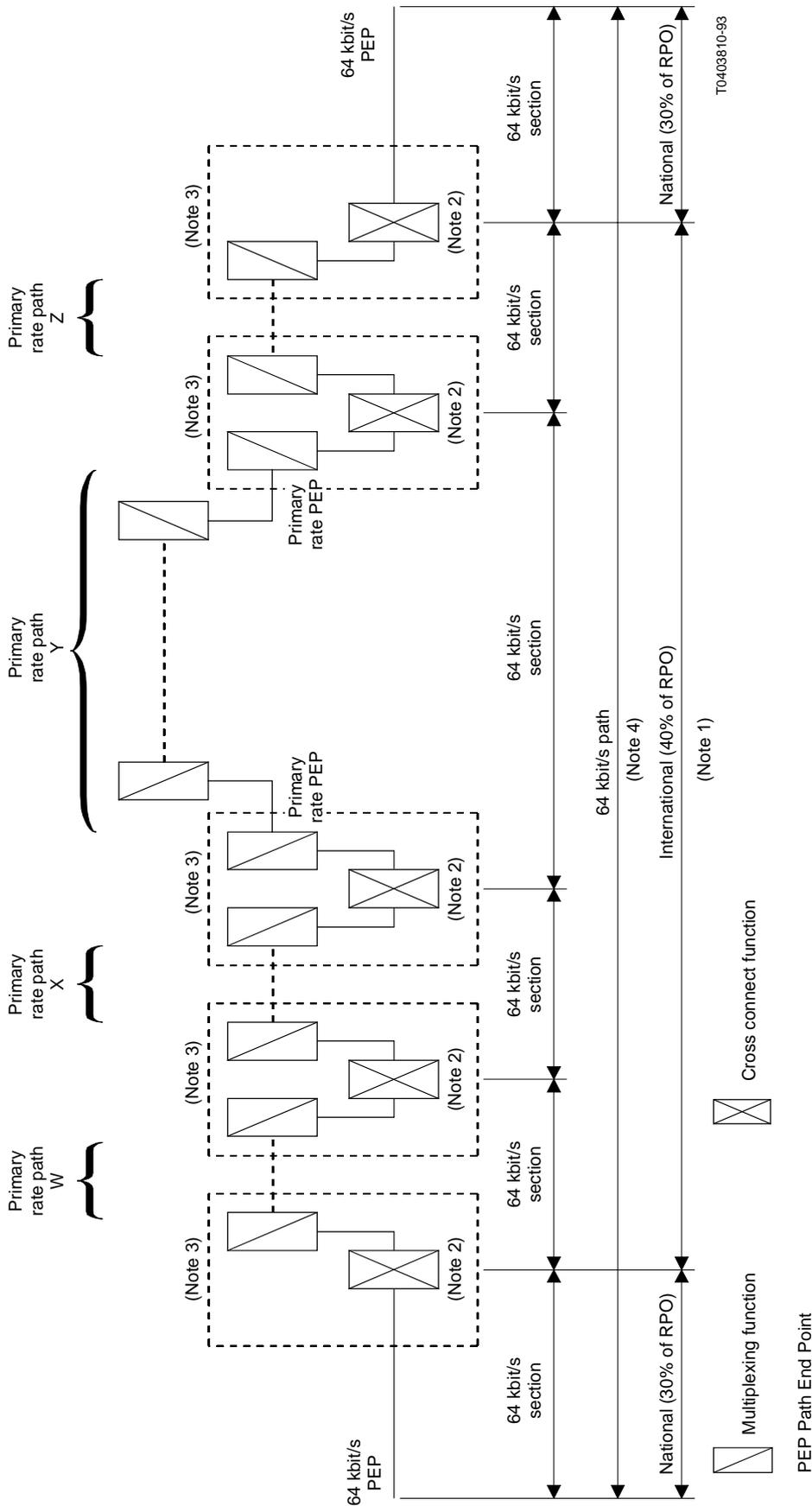
Note 1 – The International portion of 64 kbit/s path may be made up of up to 4 tandem primary rate paths W, X, Y and Z, where  $W + X + Y + Z \leq 40\%$  of the total RPO.
