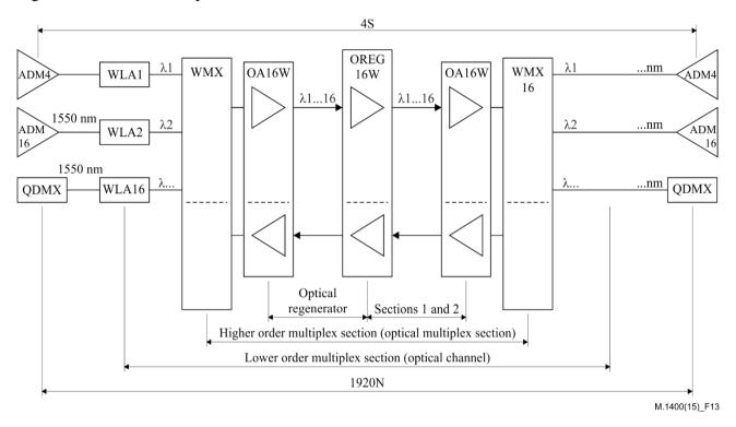
Figure 13 – Example of the scheme for DWDM with wavelength adapters on one side
