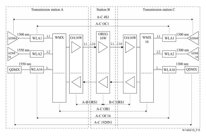
Figure 15 – Example of the DWDM scheme with the function codes
