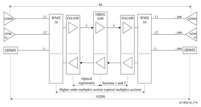
Figure 14 – Example of the scheme for DWDM without wavelength adapters
