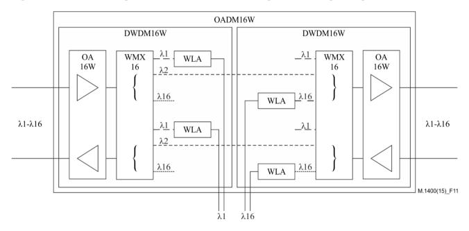
Figure 11 – Detail of the optical add-drop multiplexer 16 wavelengths with 2 wavelengths extracted and inserted
