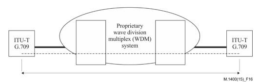
Figure 16 – Single optical channel (OCh) with reduced functionality
