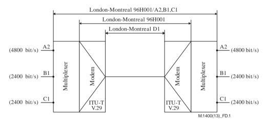
Figure D.1 – Example of the channel numbering scheme for data transmission systems
