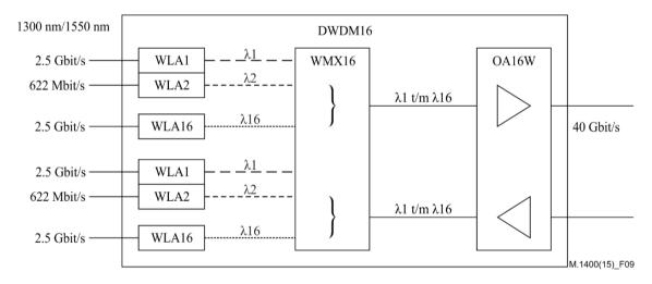
Figure 9 – Example of the equipment on one side with 16 wavelengths
