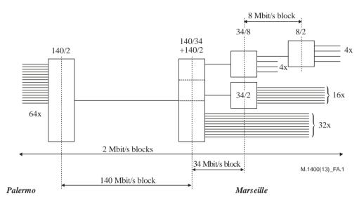
Figure A.1 – Digital block bidirectional asymmetrical configuration
