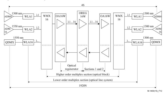
Figure 12 – Example of the scheme for DWDM with wavelength adapters on both sides
